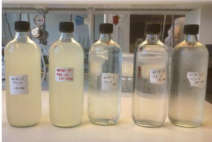
**Figure 23.** *The difference in the sediment content of the water from the locations are easily discernable. The samples were left for sedimentation for 1-2 hours before transfer and acidification of 30 mL for analysis for metals. A large part of the particles were still in suspension at this point in time and may potentially have released additional metals to the water during acidification.*
