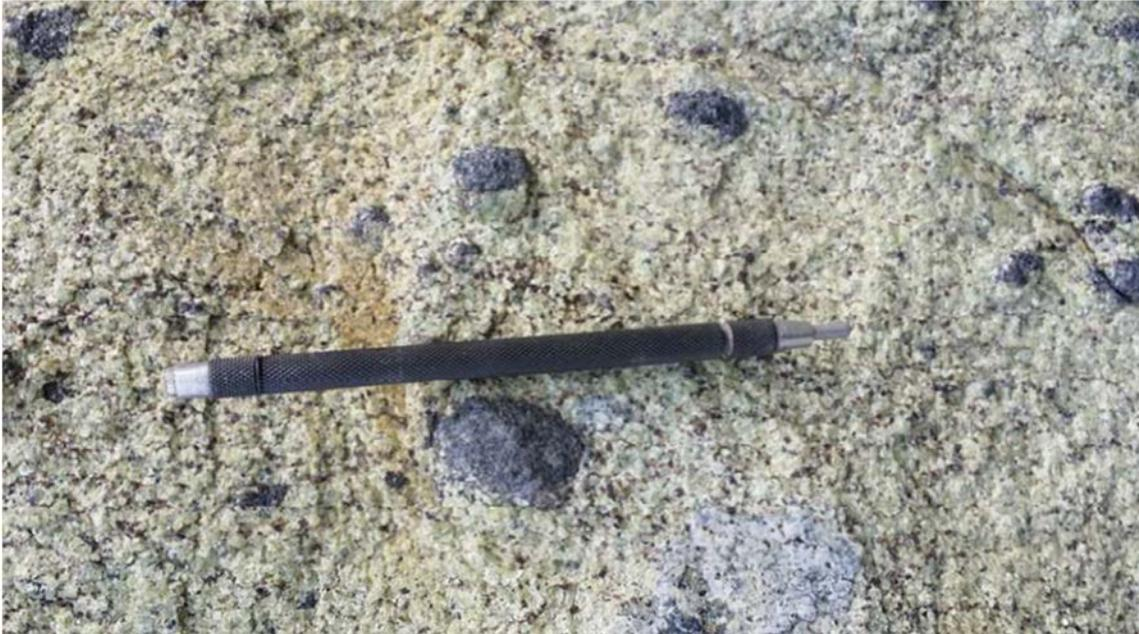
**Figure 40.** *Dunite with small brown opx crystals and large black magnetite aggregates.*
