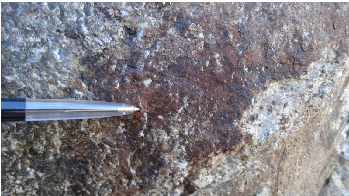
**Figure 123.** Dip-oblique slickensides along a fault plane.
