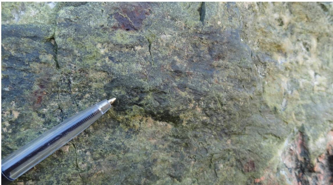
**Figure 97.** Strike-slip slickensides along the NE-SW trending fault.
