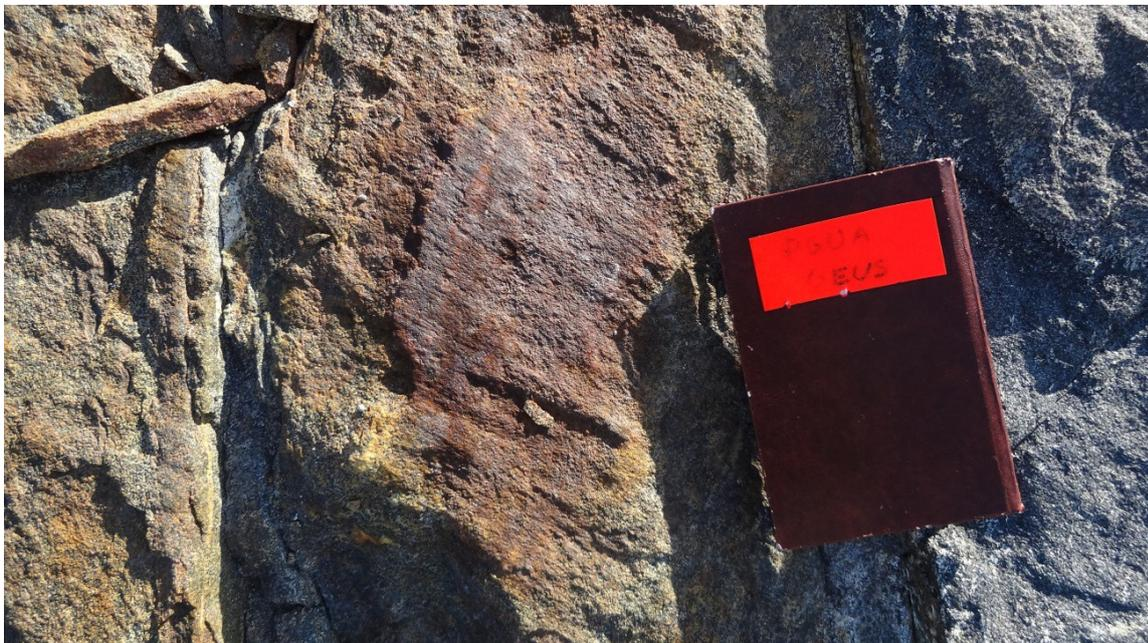
**Figure 126.** Dip-oblique slickensides along a fault plane.
