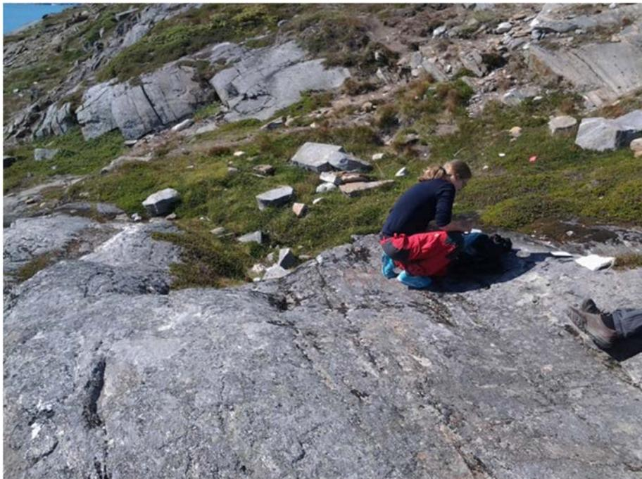
**Figure 131.** *Making sure that everything is ready for the measurements, the white plate is the spectralon for reference measurements.*
