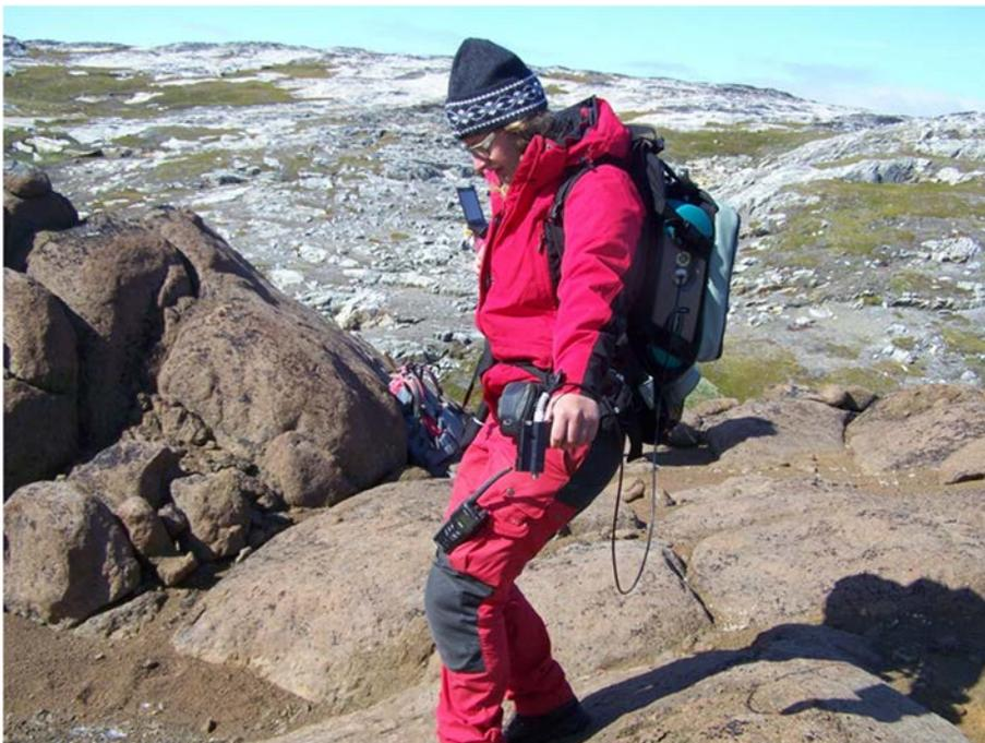
**Figure 130.** *The ASD FieldSpec operator walking towards the sun holding the sensor at an arm's length away from the body to minimise the influence on the measurements.*
