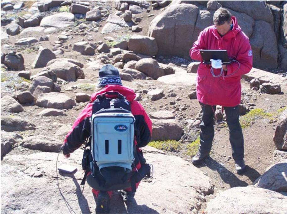
Figure 129. White reference calibration of the ASD FieldSpec 3.
