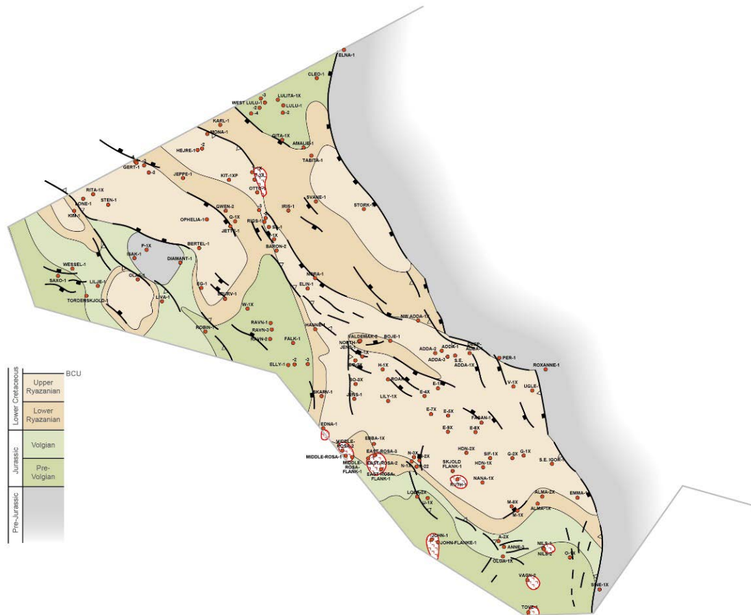
Fig. 8C.3. BCU sub-crop map with indications of degree of truncation into the Jurassic. Gentle truncation is associated with fault activity in the central part of the Central Graben. On structural highs deep erosion of the Jurassic is recognised. On the Ringkøbing Fyn High and on the Inge High the BCU marker forms the top of Paleozoic or older rocks (basement).
