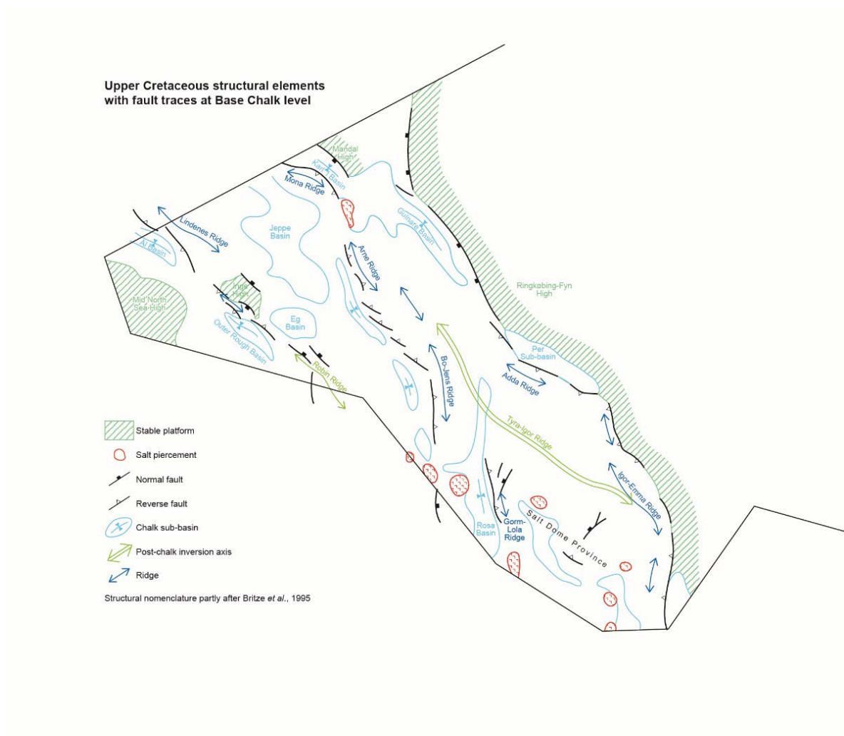
Fig. 8A.6. Upper Cretaceous structural element with fault traces at Base Chalk level.
