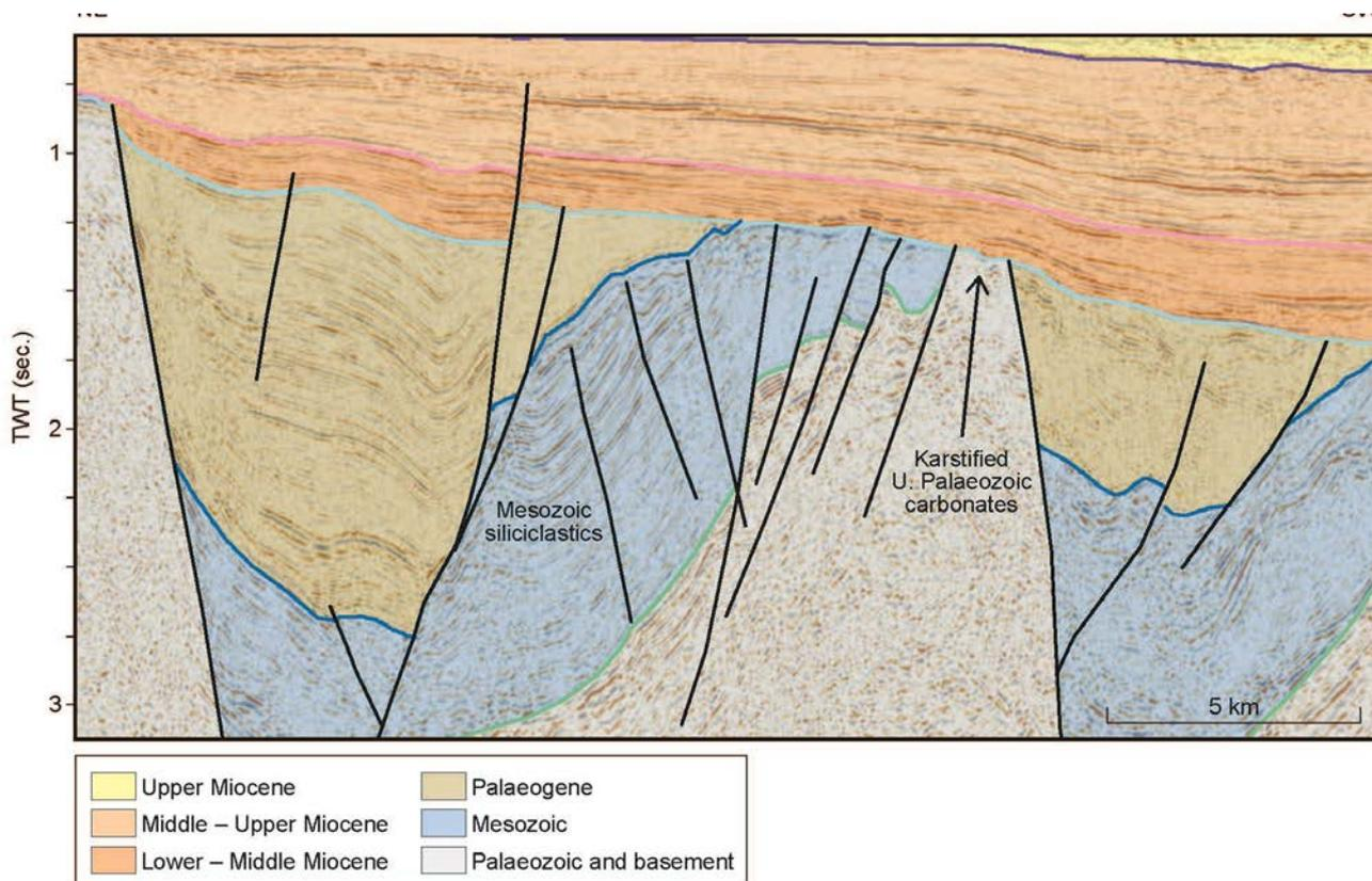
**Figure 7.** Seismic transect illustrating karstified Upper Paleozoic carbonates subcropping the Cenozoic. Younger deposits probably of Mesozoic age also subcrop the Cenozoic, but often distinguish from karstified carbonates by their smoother subcropping relief and internal reflection pattern.
