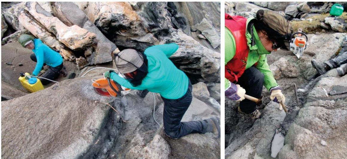
**Figure 58.** *The work carried out on the vein. First we cut a profile with the rock saw and afterwards the samples could be chipped out.*
