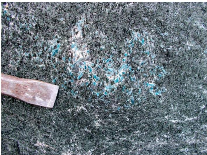
**Figure 30.** *Randomly oriented blue minerals in reaction zone with amphibole at locality 34. SEM analysis after the field season showed that the mineral is an alumnosilicate.*
