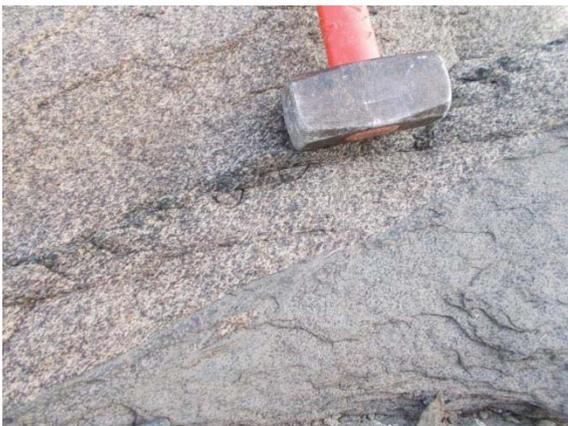
**Figure 85.** *The transition from fine grained to the coarser grained part is visible. The rock is most likely a dyke, locality 100*
