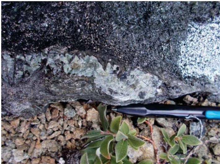
**Figure 84.** Green mineral in reaction zone in ultramafic rock, and SEM results point towards it being apatite.
