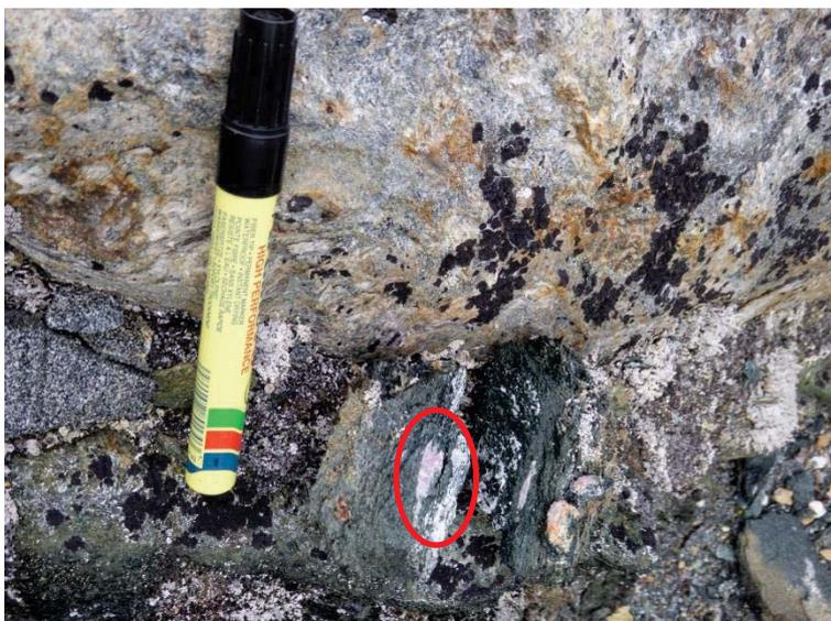
**Figure 28.** *Green amphibole with pink corundum and white feldspar. Note that the corundum grain is slightly elongated. A pegmatite is next to the corundum bearing rock.*
