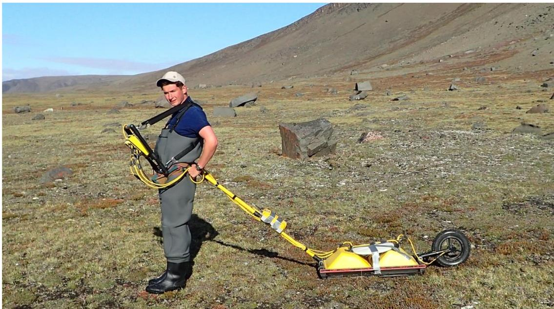
**Figure 3.** The GPR equipment in the field. The GPS antenna was mounted on the GPR antennas and between them. The GPS unit was mounted on the GPR handle.
