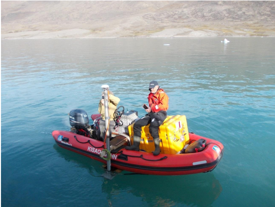
Figure 3. The Mob boat with electronics in the yellow crate. Transducer pole mounted with the GPS antenna on top.
