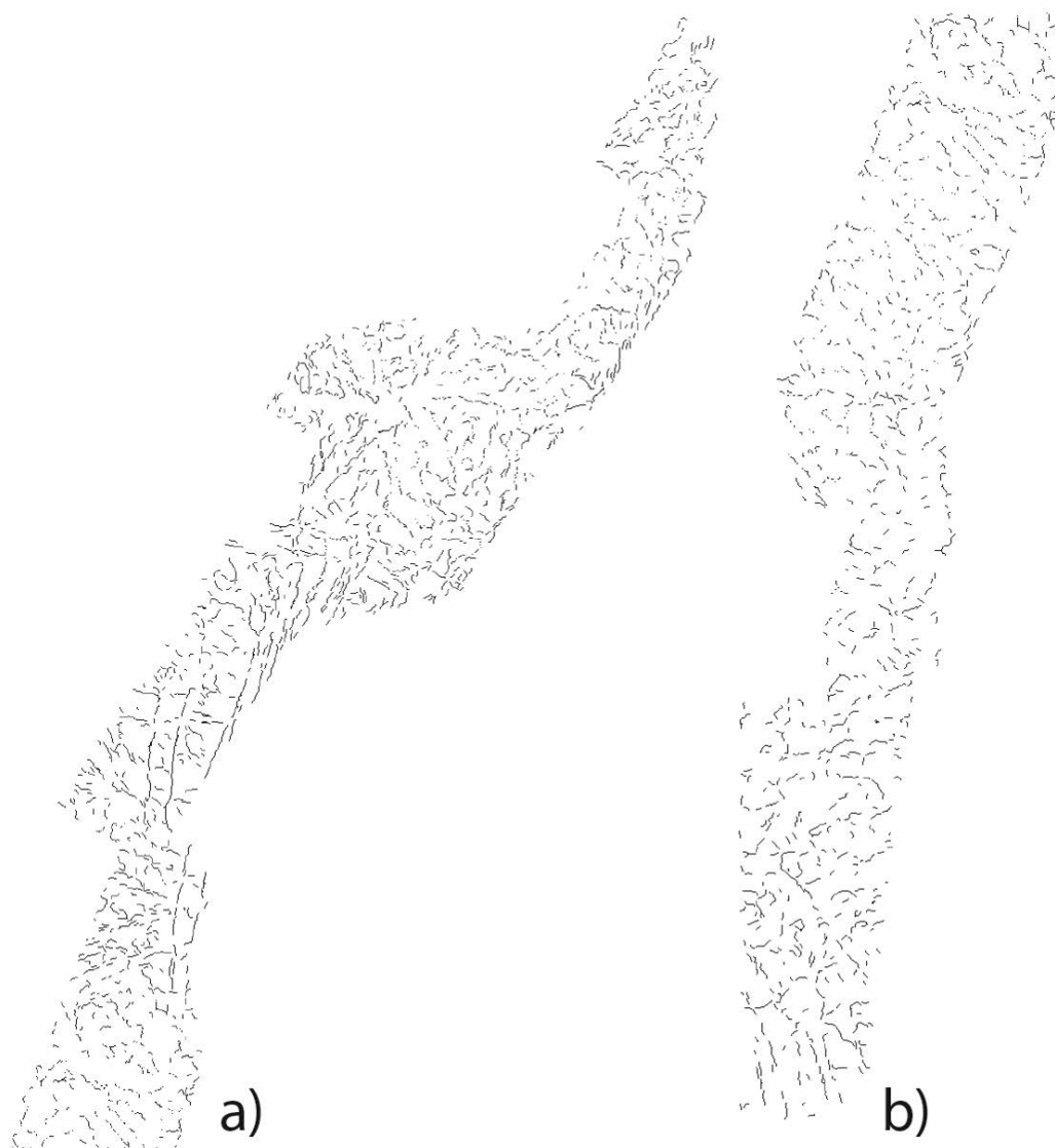
Figure 44. Because the topography of the survey area (ground clearance of the flights) artificially introduces features in Figure 40, features are removed in areas, where the curvature of the ground clearance (Fig. 43) has high magnitudes.
