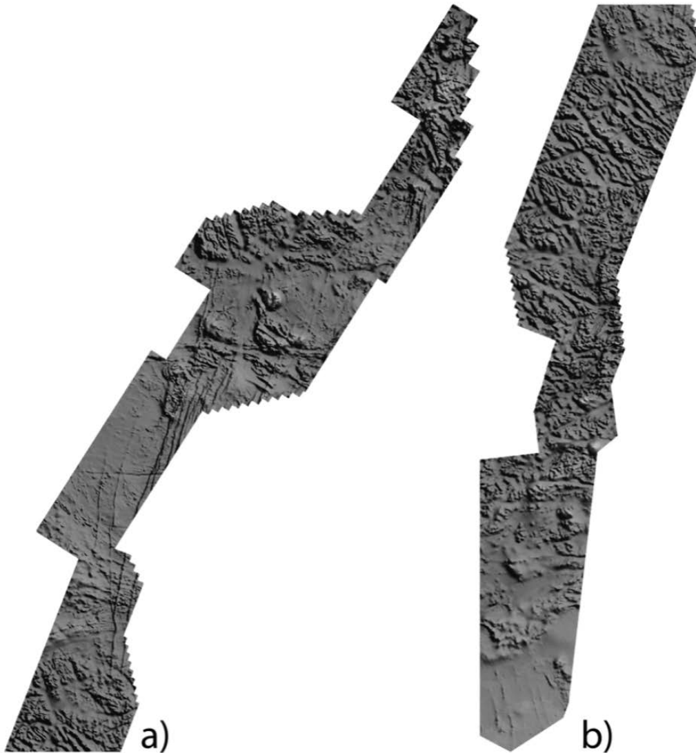
Figure 32. Shaded total magnetic intensity plots (inclination and declination of light source is 45°) from the regional airborne surveys of the AEROMAG project in East Greenland. a) and b) show the northern and southern part these surveys, respectively. A downward continuation of 100 m and a reduced-to pole transform have been applied to the displayed data.
