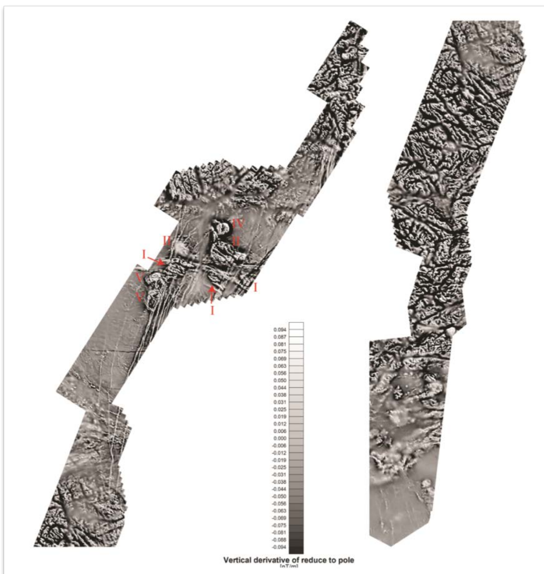
Figure 15.2 Vertical gradient of the reduced-to-pole image shown in Fig. 15.1 - for geographical location please refer to this figure. Colour shading is applied to this plot; declination and
