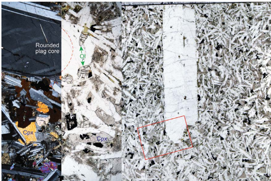
Figure 12.7 Thin section of sample GGU541367. Right half shows a flat-bed scanned image of a feldspar megacryst in a sub-ophitic matrix. To the left, a microscope photograph (crossed polarized left half and plane polarized right half) shows rounded internal outline of the feldspar megacryst overgrown by albite twinned plagioclase. The matrix is made up of plagioclase laths, subhedral olivines (ol) and opaques, as well as interstitial augite (cpx).
