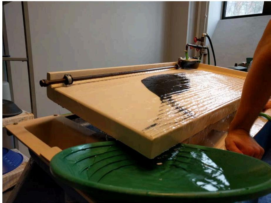
**Figure 2.** Wilfley water-shaking table used to make a heavy mineral concentrate.
