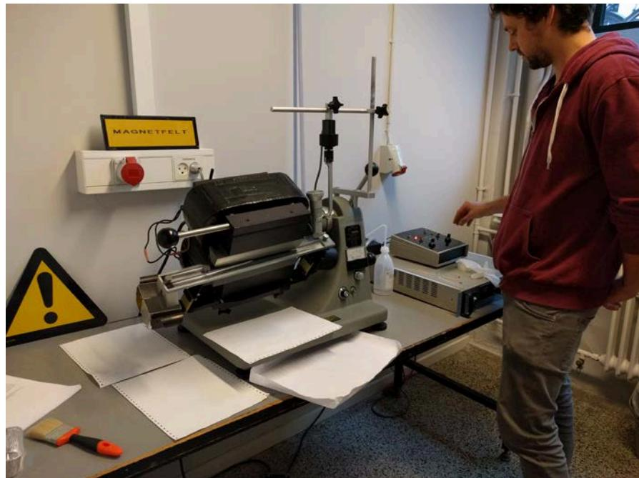
**Figure 4.** The electro-magnetic Frantz separator used for extraction of the ilmenite concentrate.
