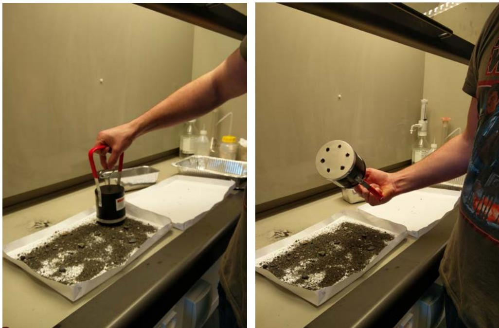
**Figure 3.** Black sand hand-magnet used for the extraction of magnetite.
