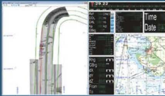
Real-time navigation using NaviPac's Helmsman's display displaying a sailing route, own position, subsea equipment position and sensor coverage.
