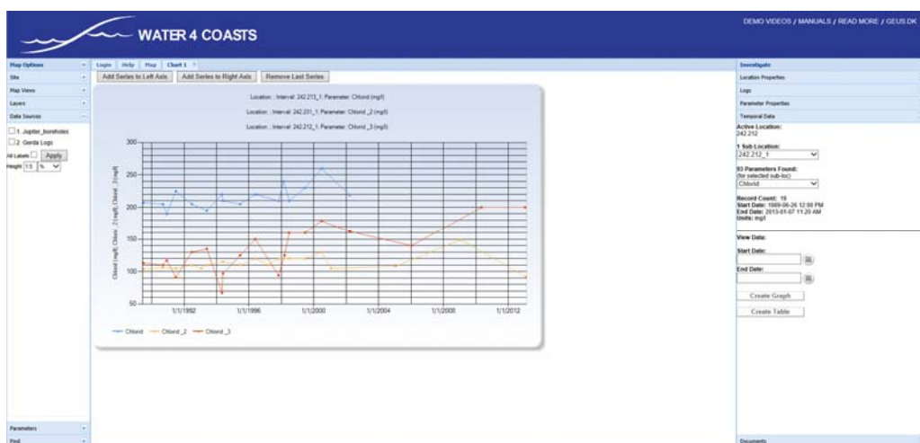
Figure 12. Graphing capabilities in EacoWeb, where data sets from different parameters and even different boreholes can be investigated online on the same graph.
