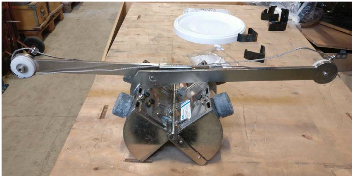
Figure 2 The Van Veen grab used for collecting offshore samples.
