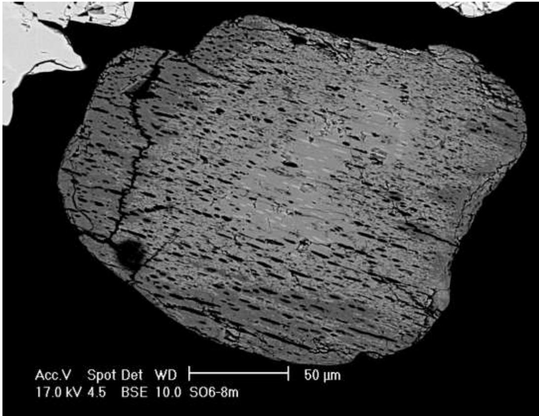
**Figure 24** Backscatter image of an ilmenite grain with increasing degree of leaching of the iron component towards the rim. In the core hematite exsolution lamina are seen (white). Where these are removed by leaching the grain has a micron scale porosity. The gray rim is pseudorutile.
