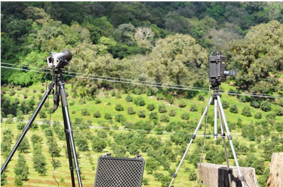
**Figure 4.** Setup of VarioCAM HD<sup>®</sup> infrared camera on the left and Flyspec<sup>®</sup> spectrometer on the right.
