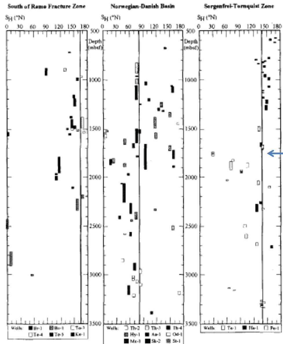
**Fig. 5.**  $S_H$  orientation vs. depth for wells south of the Rømø Fracture Zone, Norwegian-Danish Basin and Sorgenfrei-Tornquist Zone. Solid lines show the mean  $S_H$  orientation for A to C quality data in the respective tectonic regions disregarding the results from the Brems-1 and Skive-2 wells. The accuracy with which C quality data is believed to record the horizontal tectonic stress data according to Zoback (1992) is shown in grey.
