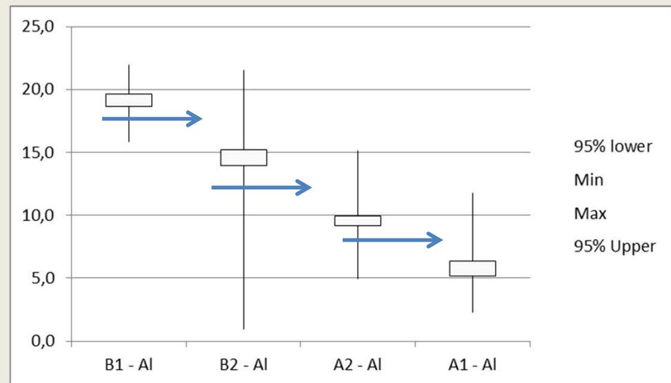
Rock type B is relatively S-rich - S content Would appear to be a very good separator between the 4 rock types
