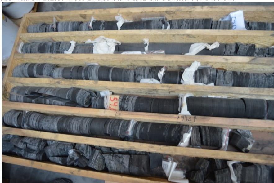
Figure 2-19: Example of core preservation from the Gislövshammar core. Box level 54 m, Furongian Peltura zone. Pyrite rich intervals are covered with the “pyrite plague” – a white “silver” layer. The high pyrite shales in the Furongian are much more reactive to the humidity than the Middle Cambrian shales.
