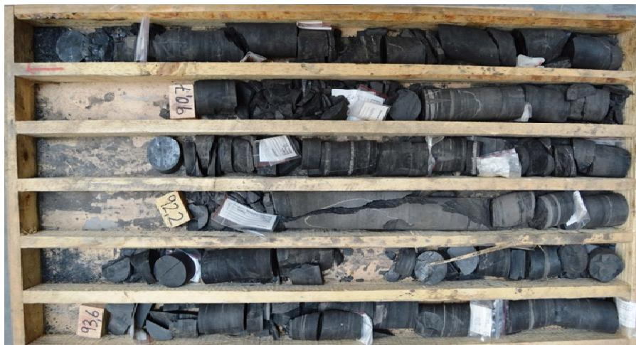
Figure 2-18: Example of core box from Gislövshammar-2. Depth 89-93 m, Middle Cambrian. Excellent preservation state. Note silt streaks and carbonate concretion.
