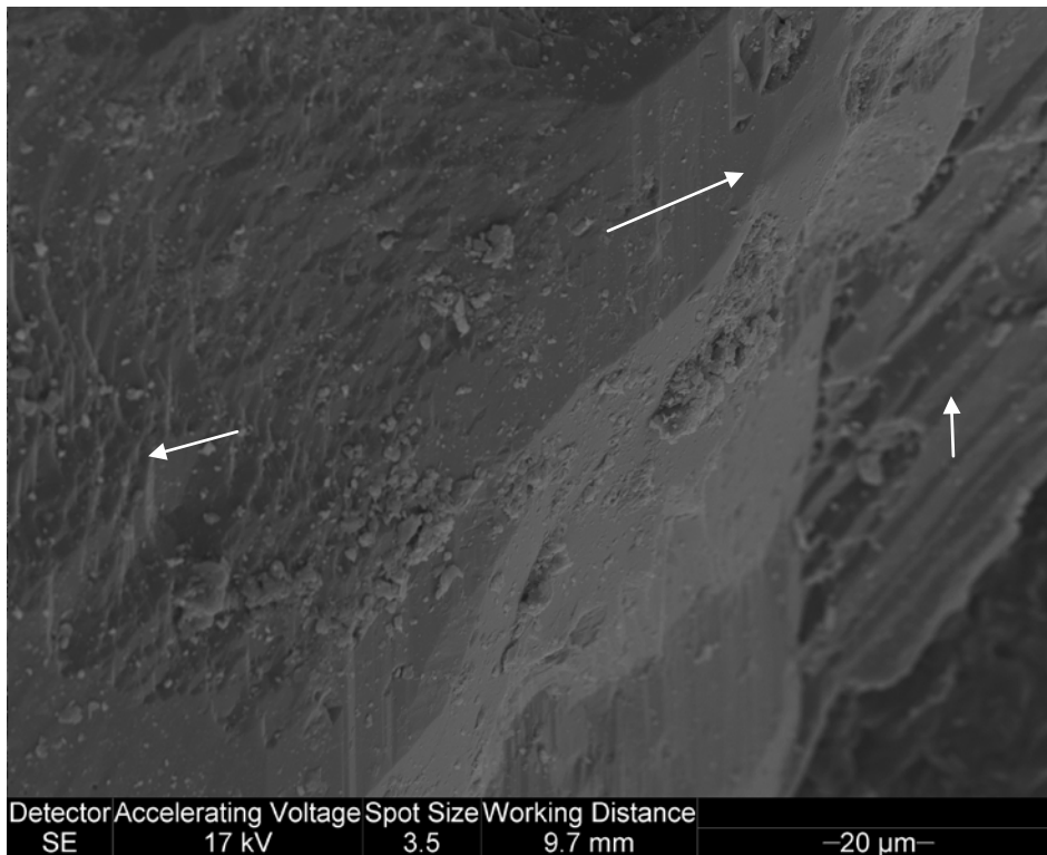
Figure 12.A: Euhedral quartz overgrowths (arrows) on a quartz grain.
