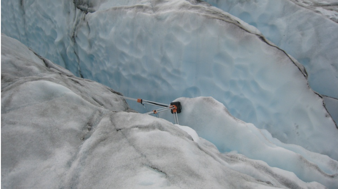
Figure 22. A GPS tracker fallen into a crevasse during the deployment period on Daugaard-Jensen Glacier (DJG in Fig. 21). Photo: Søren Nielsen © GEUS.
