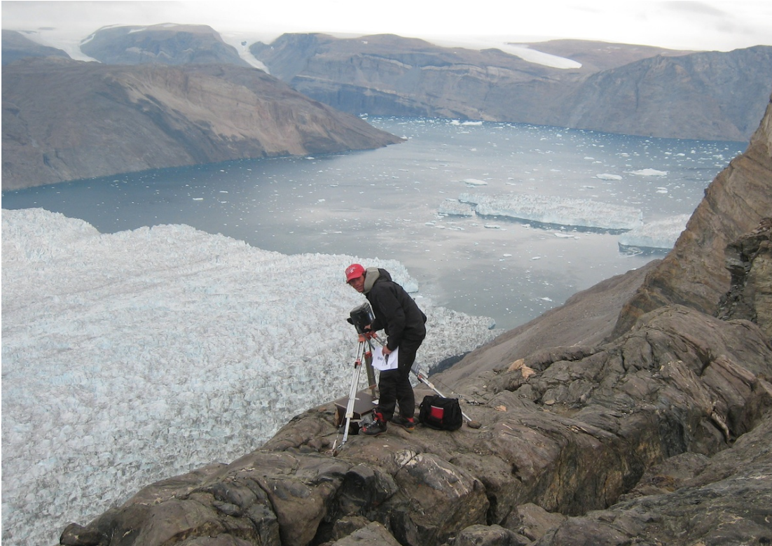
Figure 46. Maintenance and data retrieval from EIS camera at Daugaard-Jensen Glacier (DJG in Fig. 21). Photo: Søren Nielsen © GEUS.
