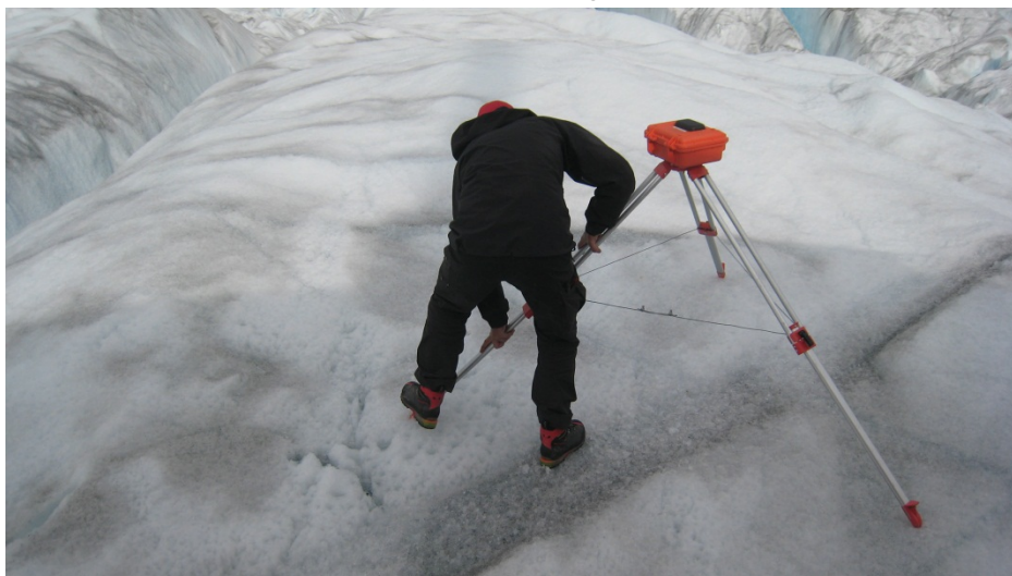
Figure 26. Deployment of a GPS tracker on Daugaard-Jensen Glacier in 2012. Photo: Søren Nielsen © GEUS.
