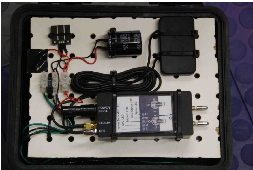
Figure 24. A look inside the IVEL GPS box with a view to antennas and the controller unit. The battery pack is situated below the board. Photo: Alberto Behar.
