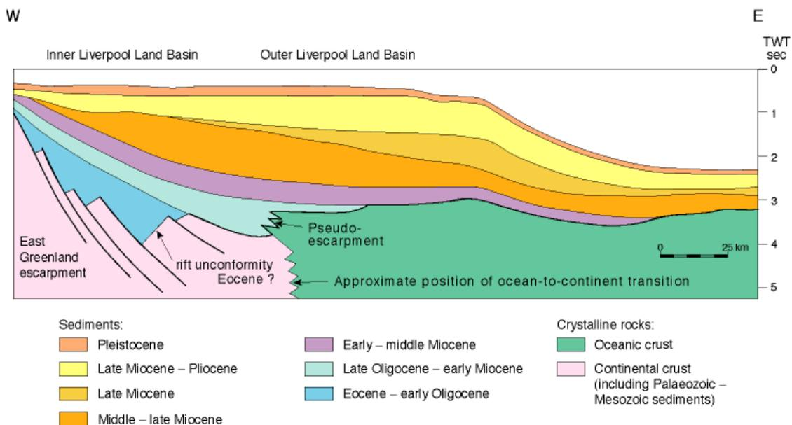
*E-W cross-section across the transition from continental crust to oceanic crust and the overlying Liverpool Land Basin at c.71 o N, East Greenland. Vertical exaggeration x 3.8.*
