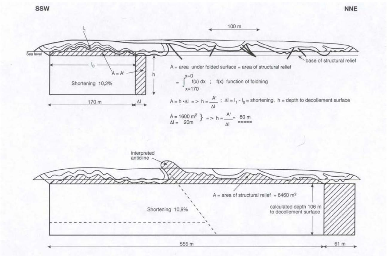
**Figure 30.** The Feggeklit cliff section and the demonstration of the calculation of the depth to the décollement surface by the application of the balanced cross section method.
