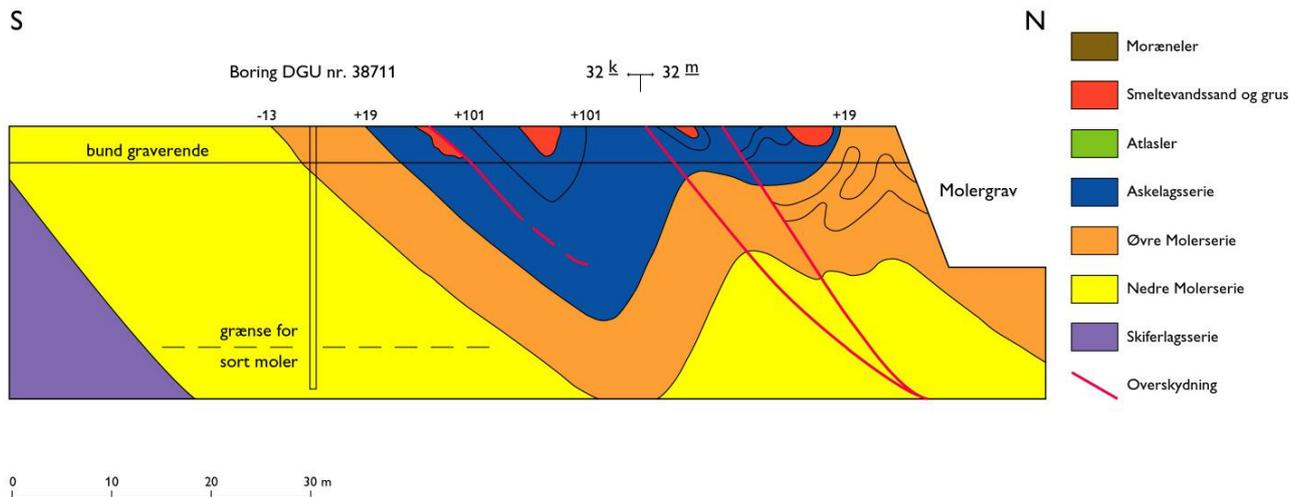
**Figure 36.** The hill crest of Fur is still the target for exploitation. In the pit instructive cross sections of the up thrust diatomite with ash layers can be seen.
