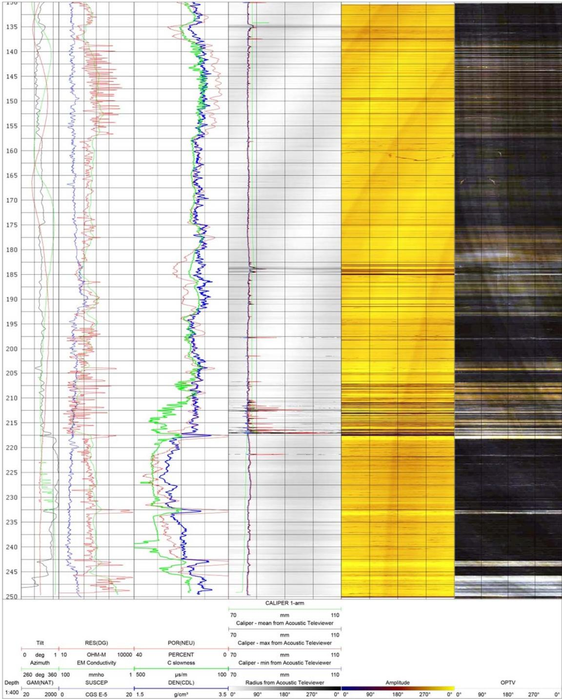
**Figure 4.** Presentation of selected logs measured in the Sommerrodde-1 well by Rambøll in the interval 130.0-250.3 m.
