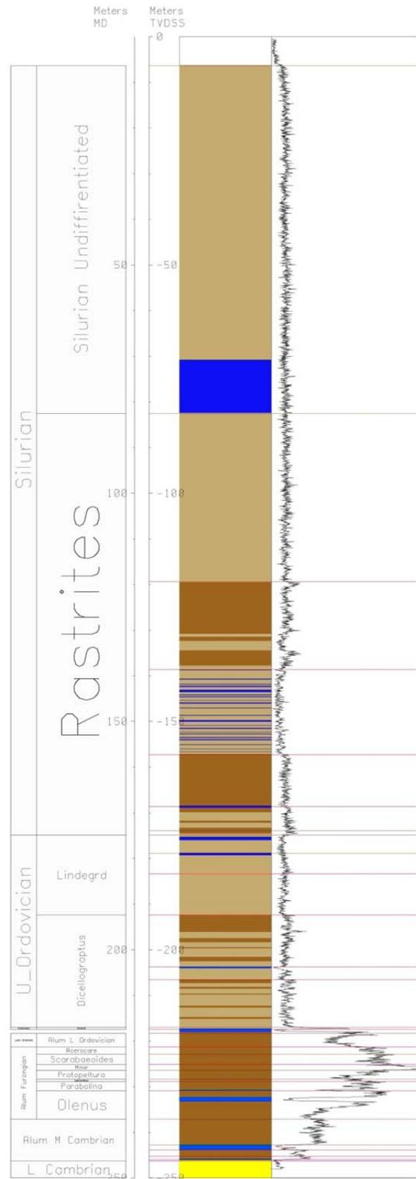
**Figure 2.** Overview of the Sommerrodde-1 well. Legend: yellow, sandstone; dark brown, dark shale; light brown, light grey-brown shale; light blue, carbonate/limestone; dark blue, carbonate cemented shale. Log curve: gamma ray curve obtained by GEUS. Log picks are presented in Table 2.
