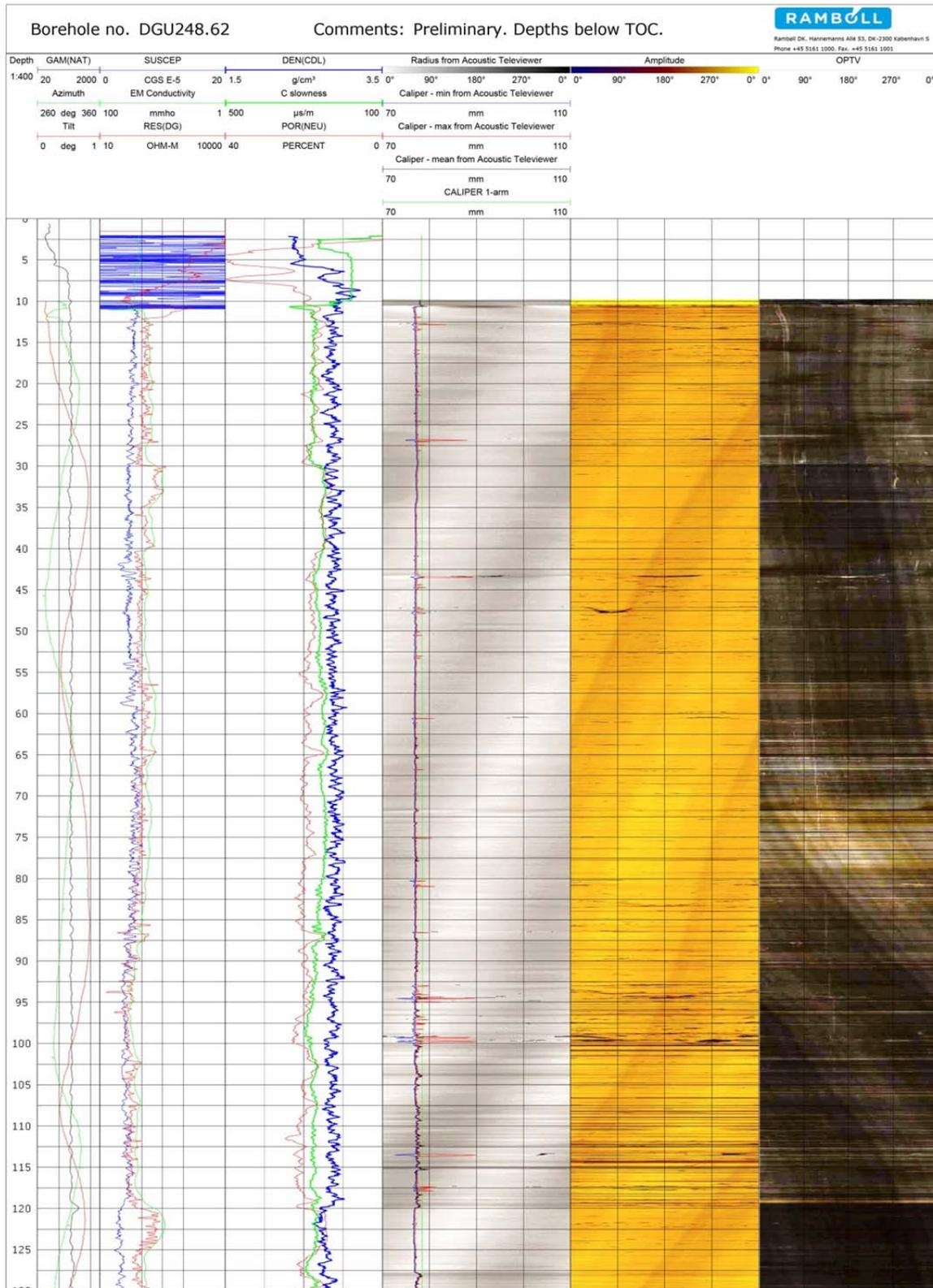
**Figure 3.** Presentation of selected logs measured in the Sommerrodde-1 well by Rambøll in the interval 0-130.0 m.
