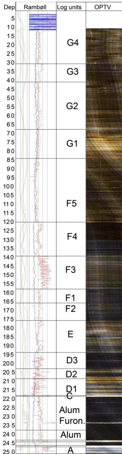
**Figure 11.** Logstratigraphical analysis of the Sommerodde well. The logs are obtained by Rambøll (see Figure 3 and 4).
