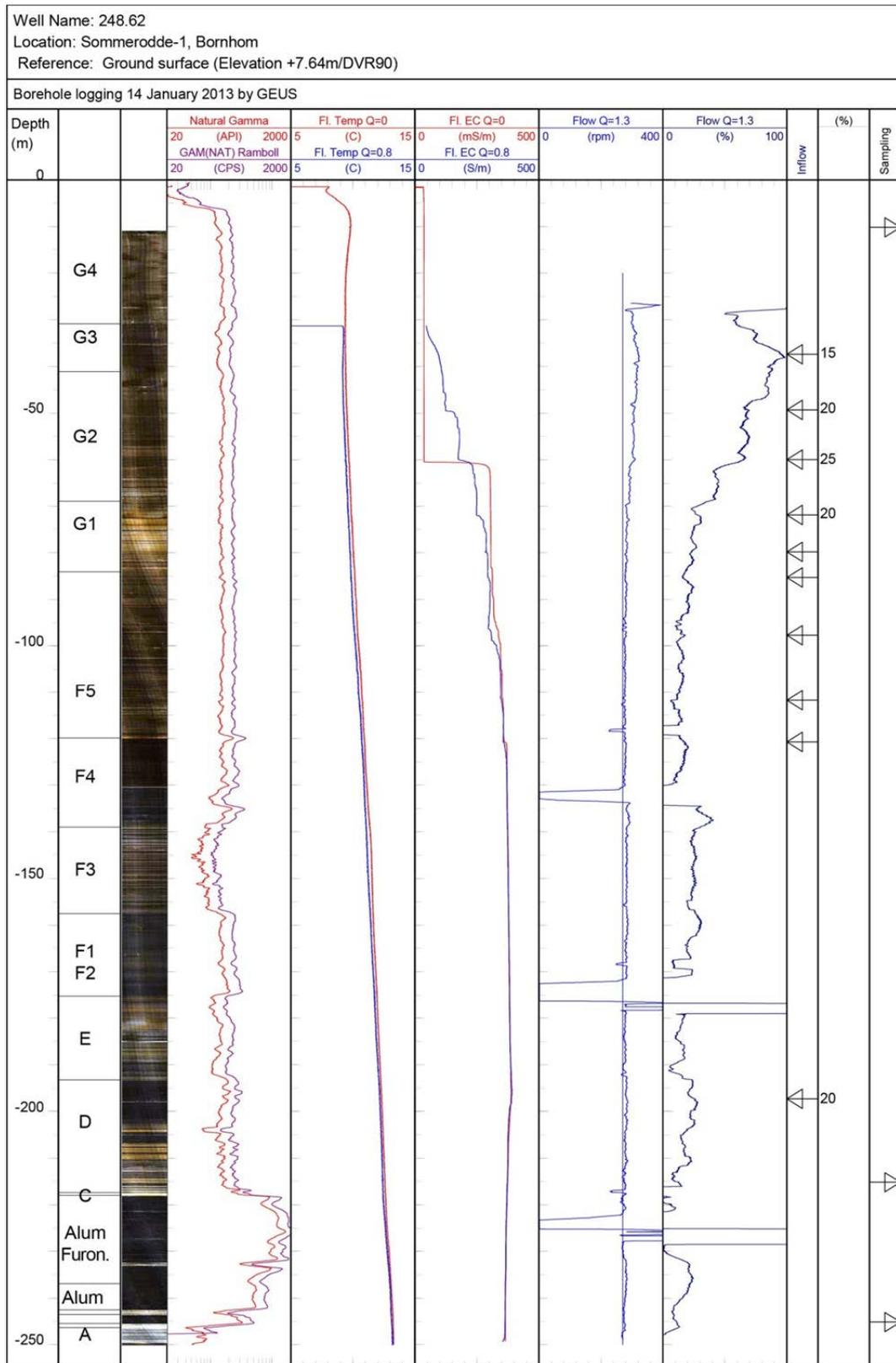
**Figure 5.** Presentation of logs measured in the Sommerodde-1 well by GEUS. Arrows pointing to the left indicate significant water inflow zones. Number indicate the percentage contribution to the total flow for each inflow zone. Arrows pointing to the right indicate position of water samples. The optic televiwer shown on the left is acquired by Rambøll.
