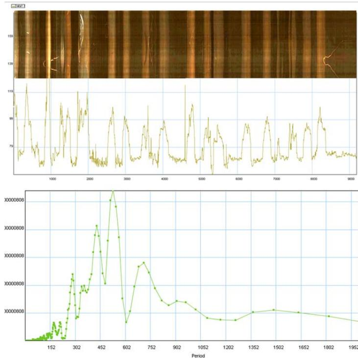
**Figure 12.** Example of an analysis of the cyclicity in the F3 unit. The top illustration shows a 7.8 m long section from the optic televiwer log and the corresponding grey tone variation within the interval. The illustration below shows a spectral density analysis of the grey tone variation. The periods are in pixels (9187 along the 7.8 m section) and the analysis indicates that there are multiple frequencies present notably at 24, 37 and 42 cm.
