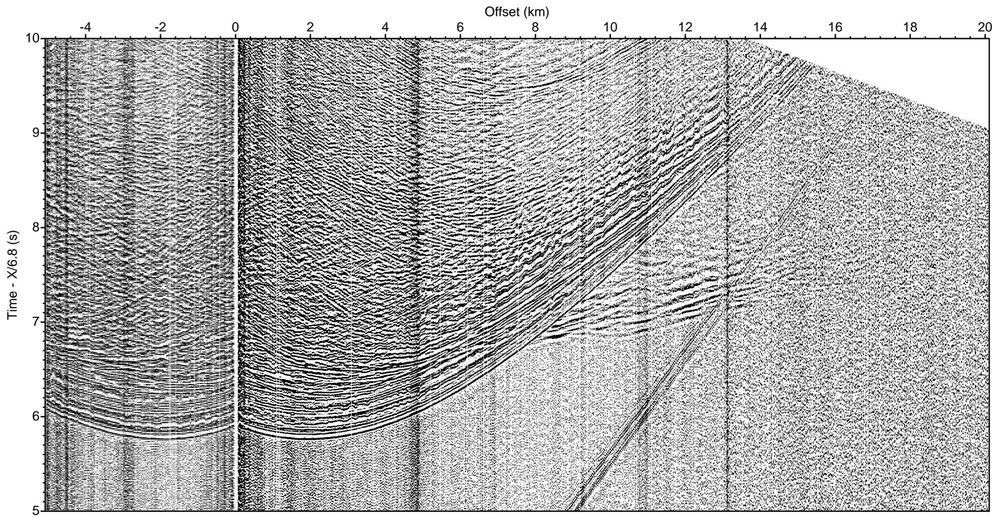
LOMROG III (2012) - Line 9 Sonobuoy 9-30 aux ch 3 (drift correction, deconv., bpf 5-40 Hz)
