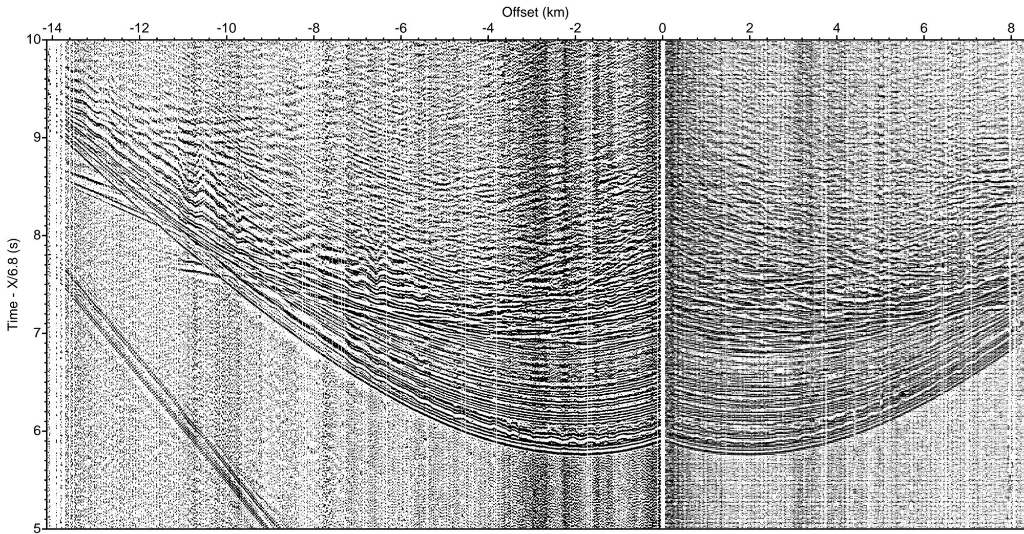
LOMROG III (2012) - Line 10 Sonobuoy 10-32 aux ch 4 (drift correction, deconv., bpf 5-40 Hz)
