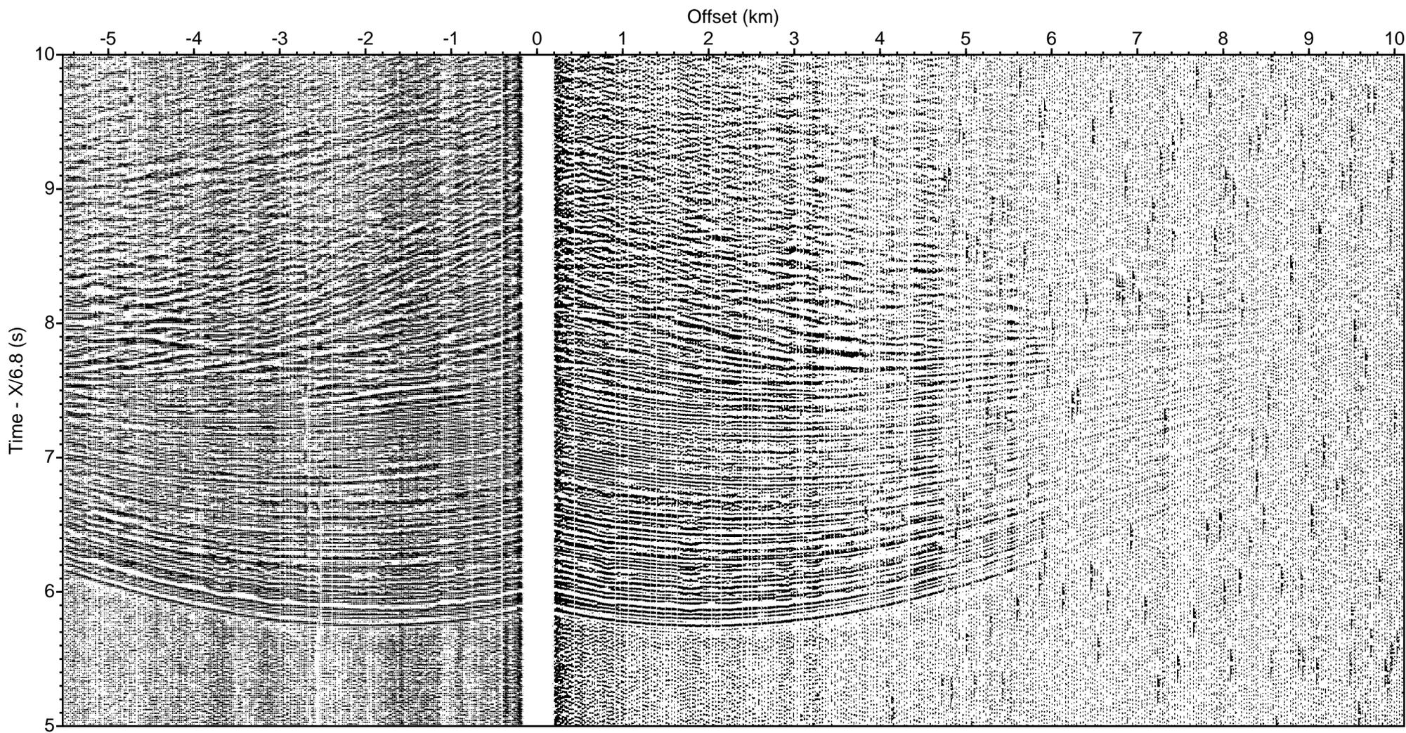
LOMROG III (2012) - Line 12 Sonobuoy 12-42 aux ch 2 (drift correction, deconv., bpf 5-40 Hz)
