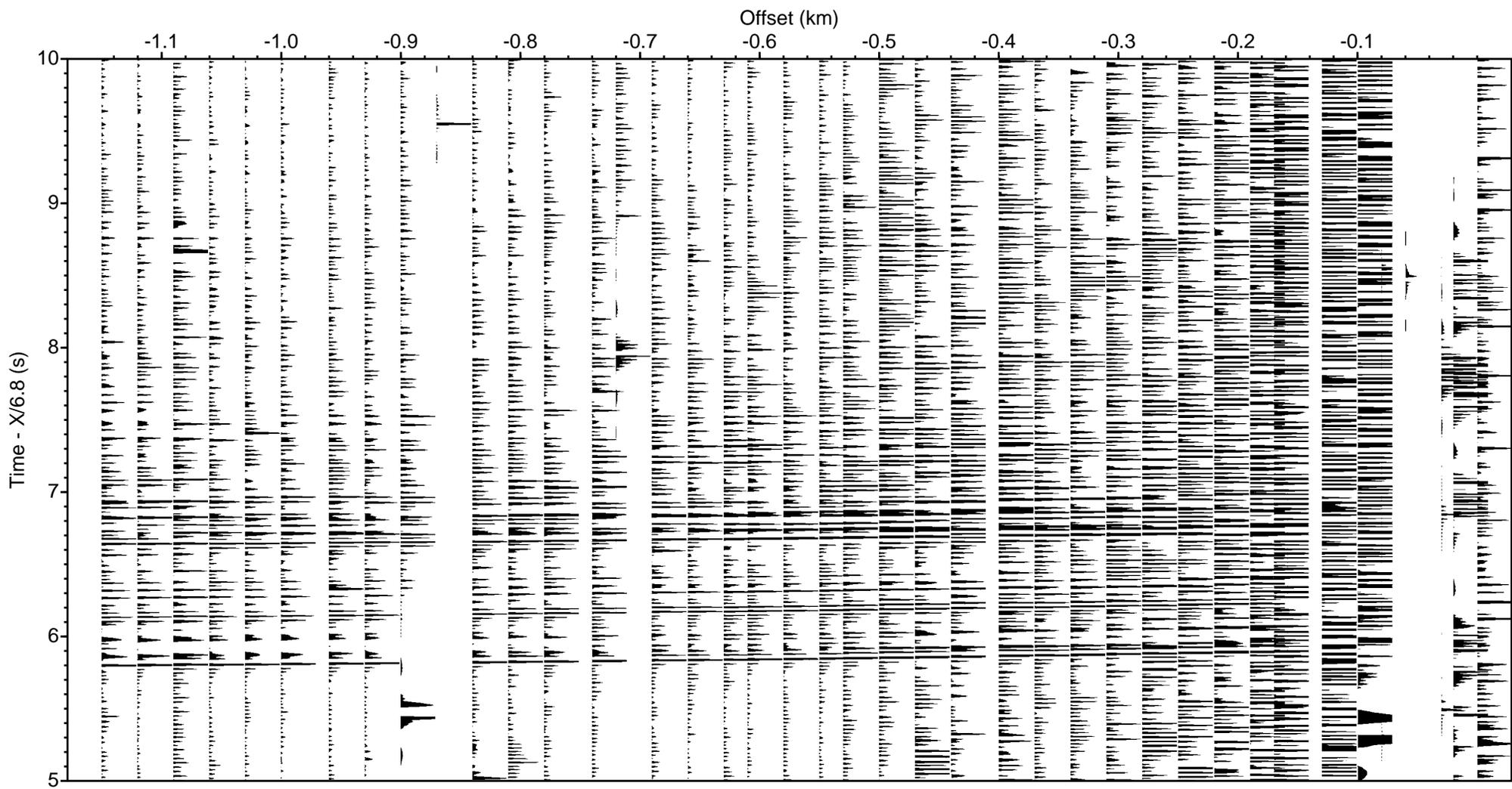
LOMROG III (2012) - Line 10 Sonobuoy 10-31 aux ch 1 (drift correction, deconv., bpf 5-40 Hz)
