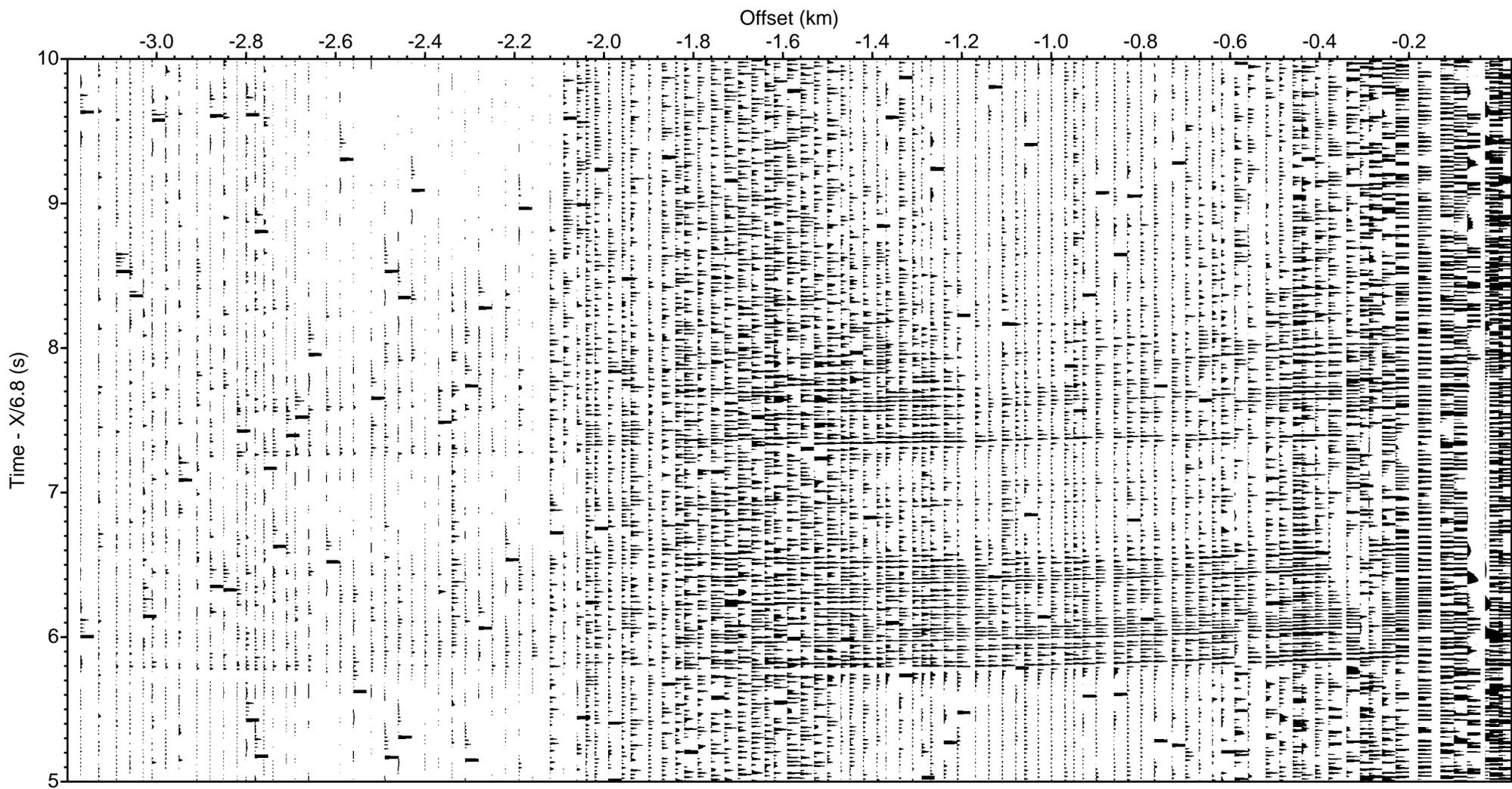
LOMROG III (2012) - Line 11 Sonobuoy 11-36 aux ch 1 (drift correction, deconv., bpf 5-40 Hz)
