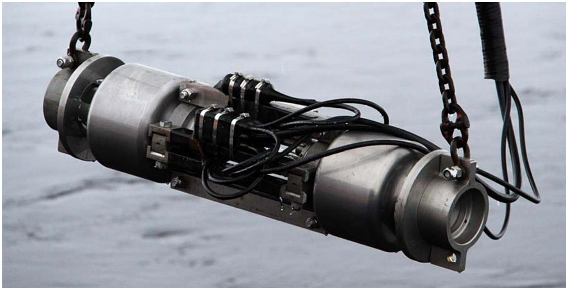
**Figure 22.** 1040 cu. in. G-gun array used for the seismic experiment.
