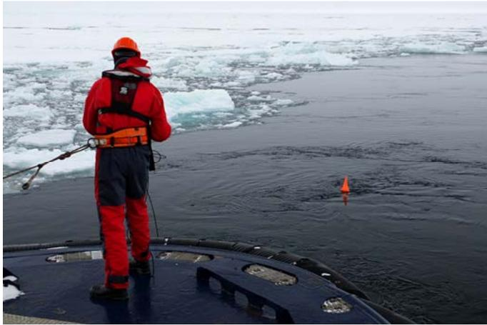
**Figure 30.** Sonobuoy deployment from the afterdeck of Oden. The parachute (not shown) of the sonobuoy is attached to a rope during the deployment. Photo: Marie Lykke Rasmussen.
