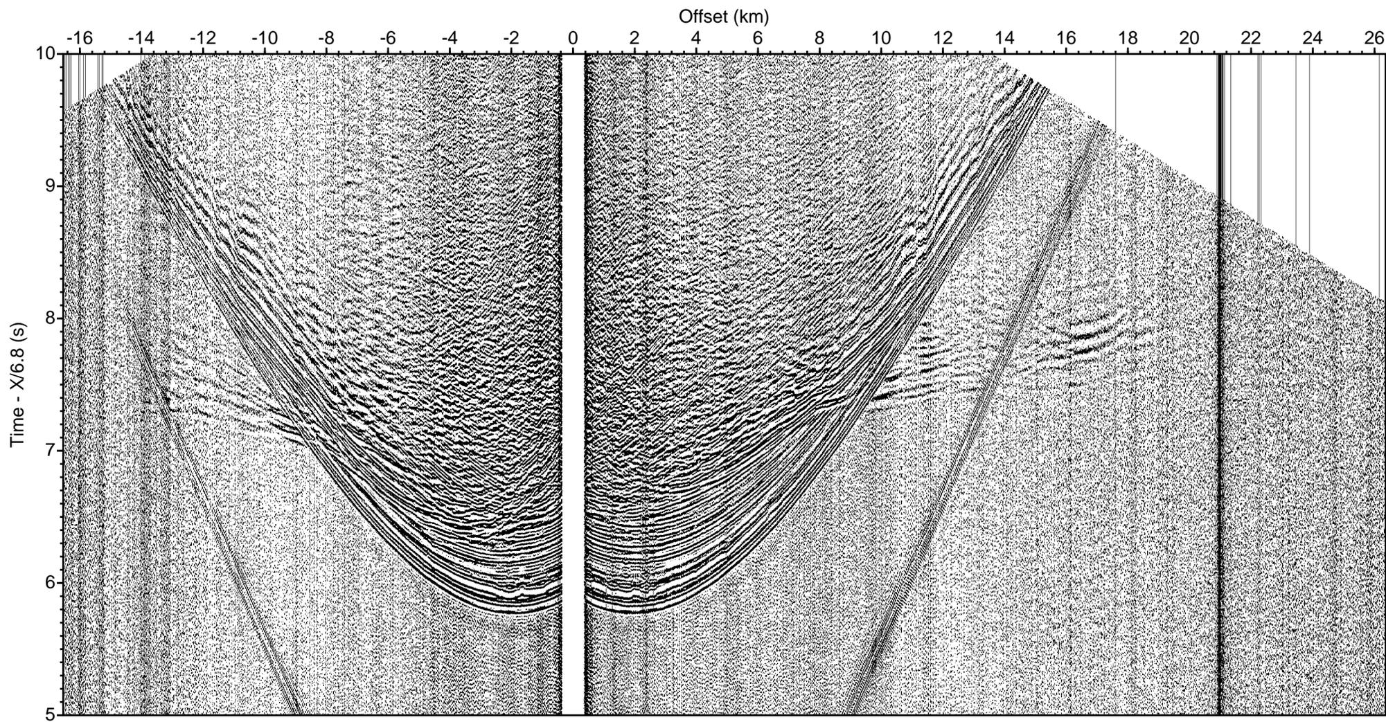
LOMROG III (2012) - Line 7 Sonobuoy 7-22 aux ch 3 (drift correction, deconv., bpf 5-40 Hz)
