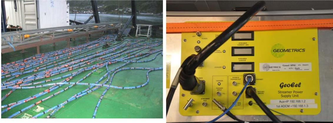
**Figure 4.** *Geometrics GeoEel streamer on deck (left) - for streamer on winch see Figs. 9 and 11. Geometrics GeoEel streamer power supply unit SPSU (right).*
