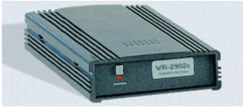
The WINRADIO WR-2902e VHF/UHF Sonobuoy Telemetry Receiver is designed to receive signals from analogue (DIFAR) and digital (BARRA) sonobuoy transmitters, operating in the 136 to 173.5 MHz frequency range. This standard frequency range can be easily extended up to 1.5 GHz to suit special requirements.
