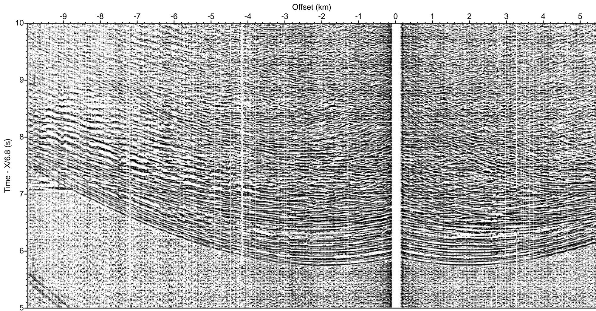
LOMROG III (2012) - Line 17 Sonobuoy 17-61 aux ch 4 (drift correction, deconv., bpf 5-40 Hz)
