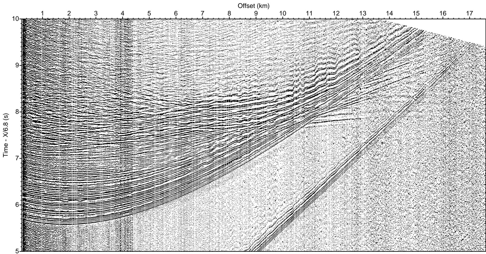
LOMROG III (2012) - Line 12 Sonobuoy 12-43 aux ch 3 (drift correction, deconv., bpf 5-40 Hz)
