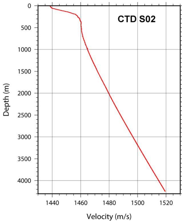
**Figure 34.** Velocity-depth function obtained from CTD measurement S02. The complete set of CTD measurements relevant to the seismic data are shown in Appendix C.
