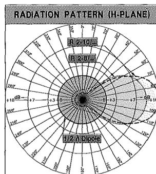
If the antennas are mounted for vertical polarization these curves show the radiation patterns in the vertical plane.
