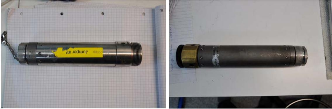
**Figure 17.** Photos of the new connection jumpers. On the left photo is the jumper cable side; while on the right photo is the streamer cable side. These new connectors make it easier to connect the jumper cable and the streamer section for the people working at the tail fan of Oden.
