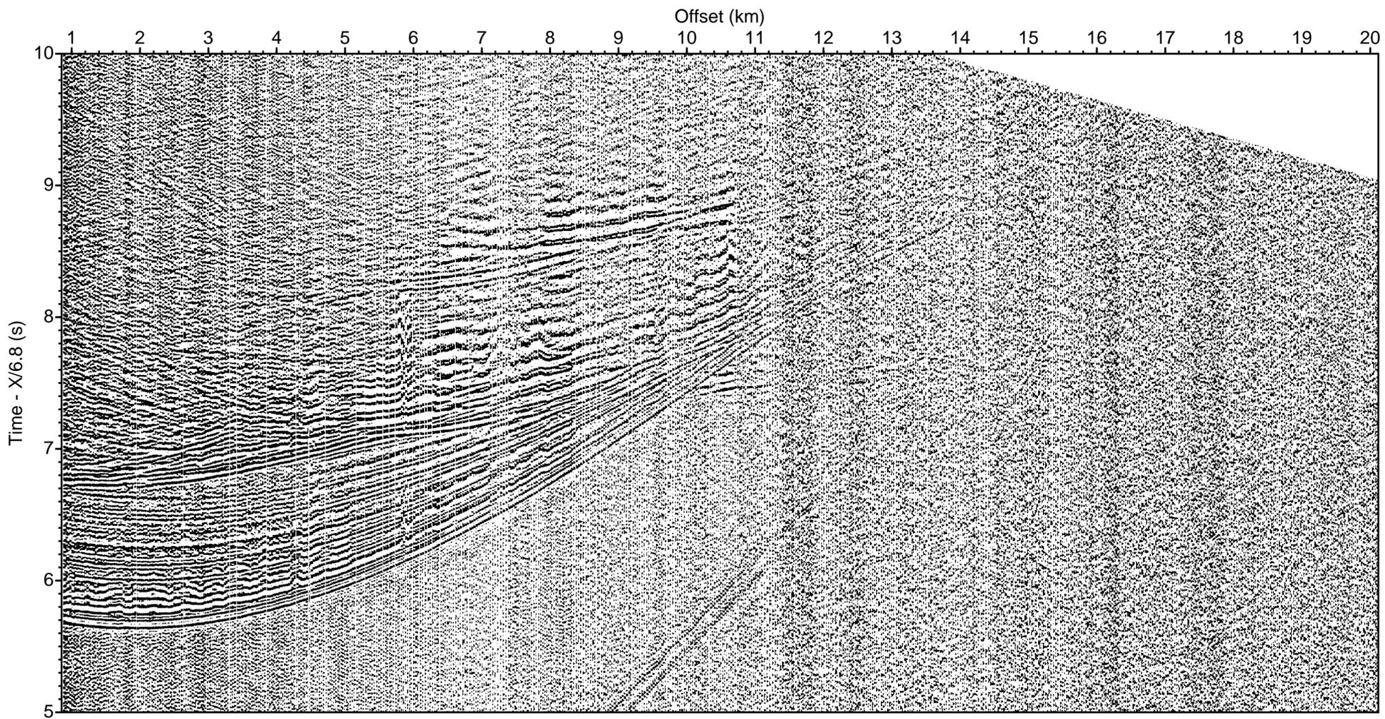
LOMROG III (2012) - Line 2 Sonobuoy 2-6 aux ch 4 (drift correction, deconv., bpf 5-40 Hz)
