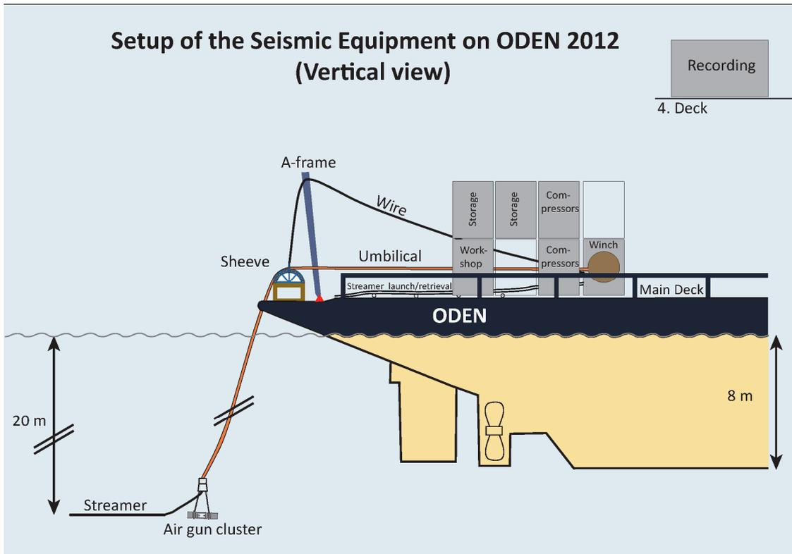
**Figure 19.** Vertical view of the setup during data acquisition. The text in the grey rectangles (containers) indicates the function they have in the seismic setup.
