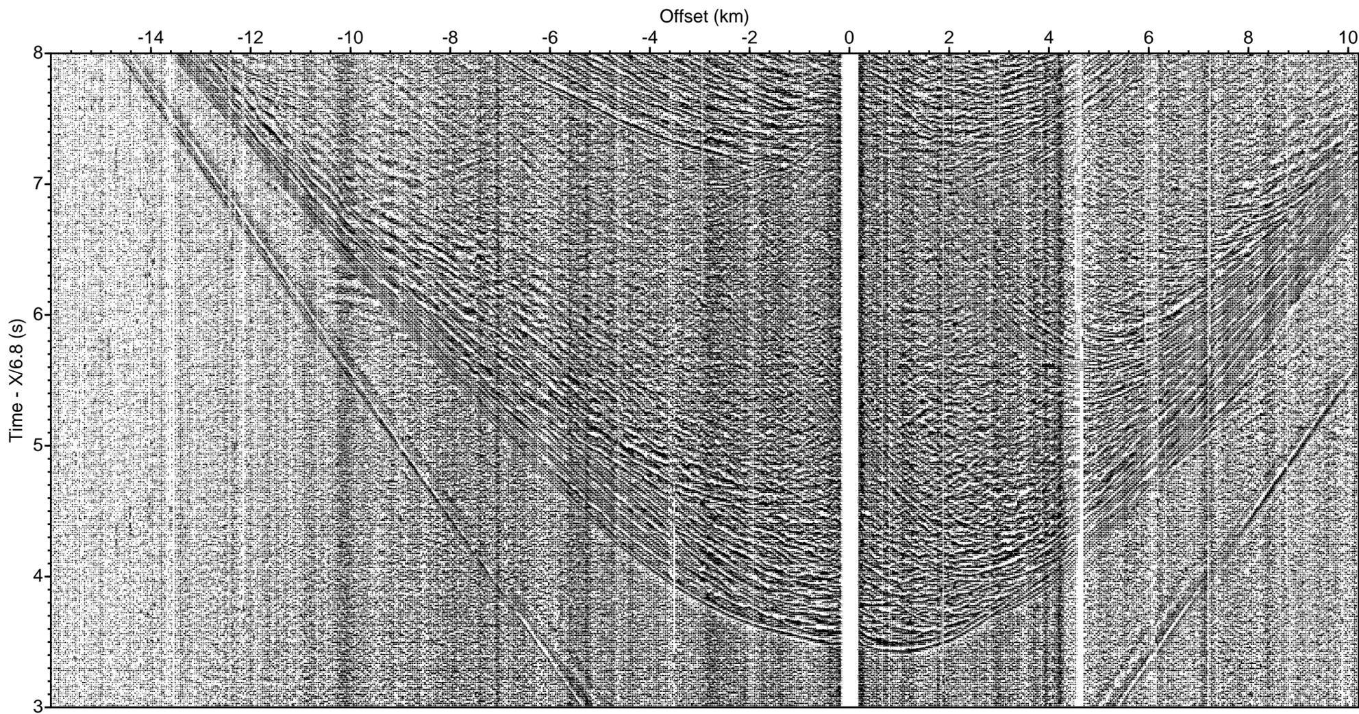
LOMROG III (2012) - Line 6 Sonobuoy 6-16 aux ch 2 (drift correction, deconv., bpf 5-40 Hz)
