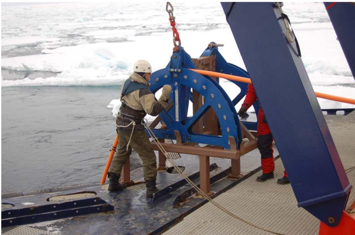
**Figure 18.** Umbilical sheave locked and air gun and streamer fully deployed.
