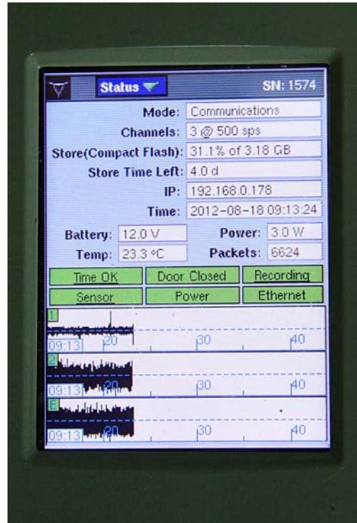
**Figure 26.** Taurus seismometer in the recording container on the fourth deck of Oden.
