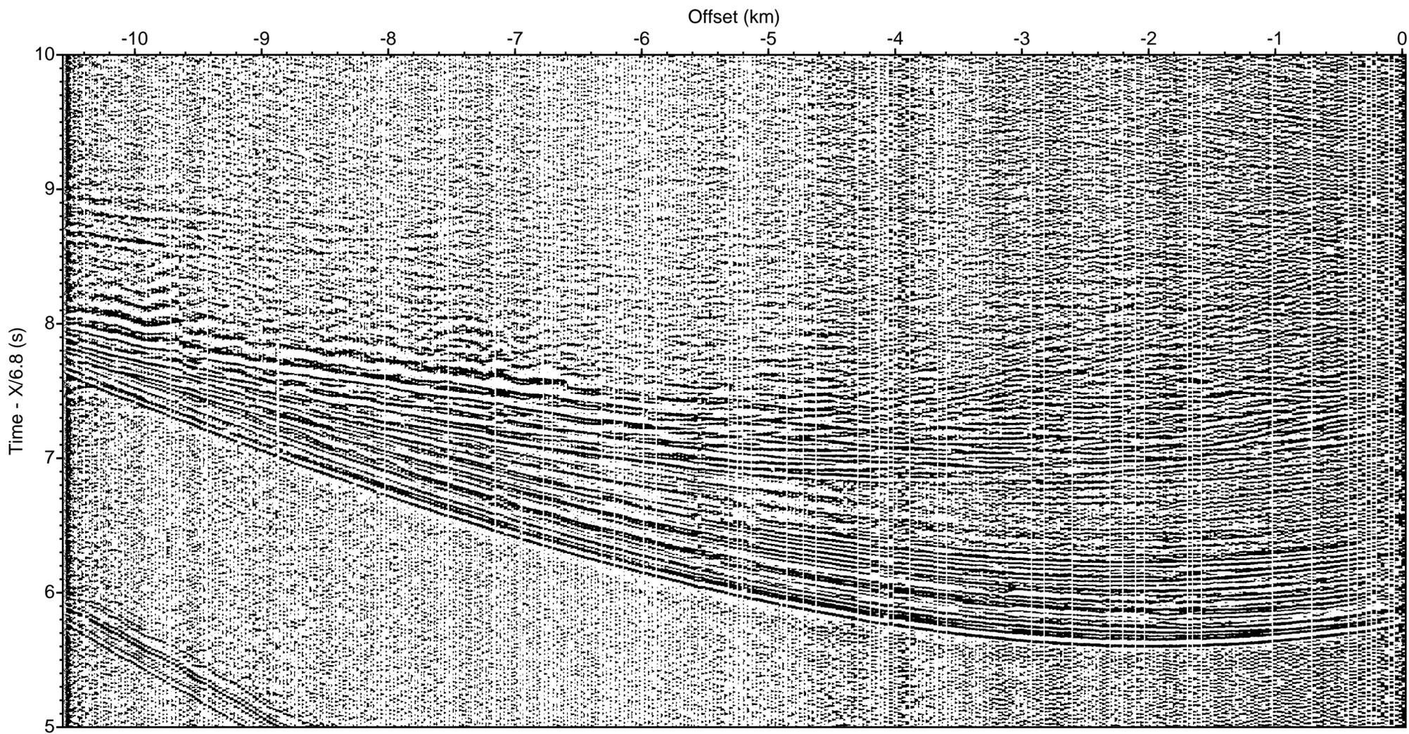
LOMROG III (2012) - Line 2 Sonobuoy 2-10 aux ch 3 (drift correction, deconv., bpf 5-40 Hz)
