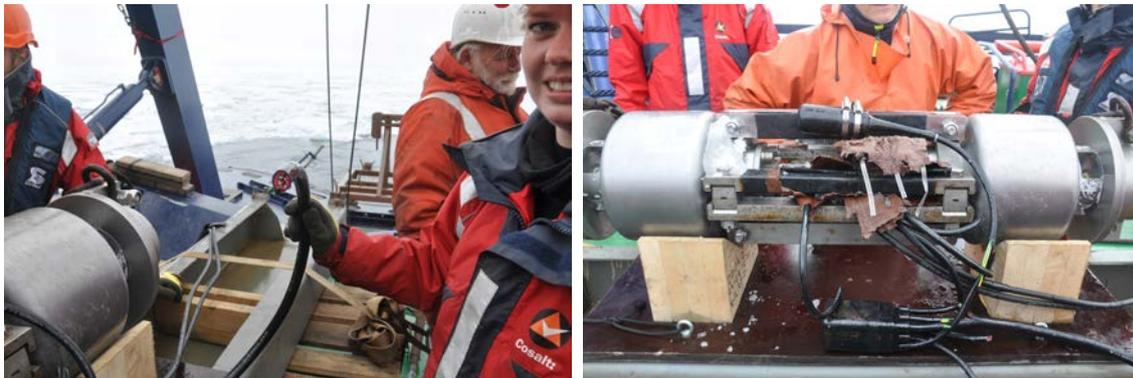
**Figure 20.** Pictures of the airgun array after the encounter with a large piece of ice. A chunk of the ice is still visible on the left side of the airgun array; also notice the clean cut of the cable.
