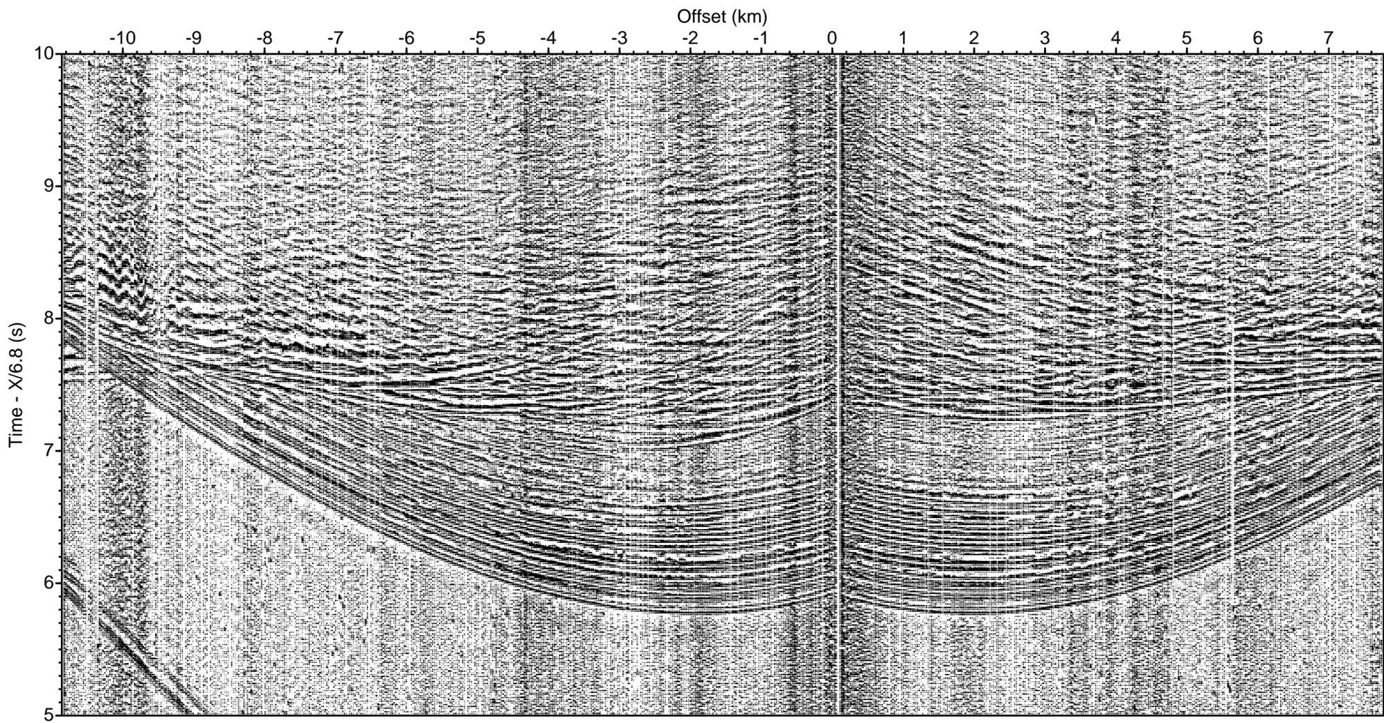
LOMROG III (2012) - Line 16 Sonobuoy 16-57 aux ch 4 (drift correction, deconv., bpf 5-40 Hz)
