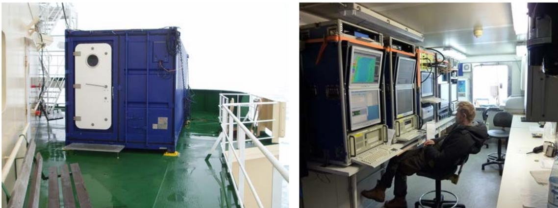
**Figure 10.** Recording container on deck 4 (left) and interior of the container (right).
