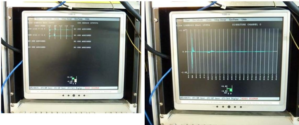
**Figure 3.** The Macha TGS-8 software running on its own dedicated computer. Display showing the timing of the two air guns in the array (left) and on the right the display showing the nearfield pulse from the air gun array.
