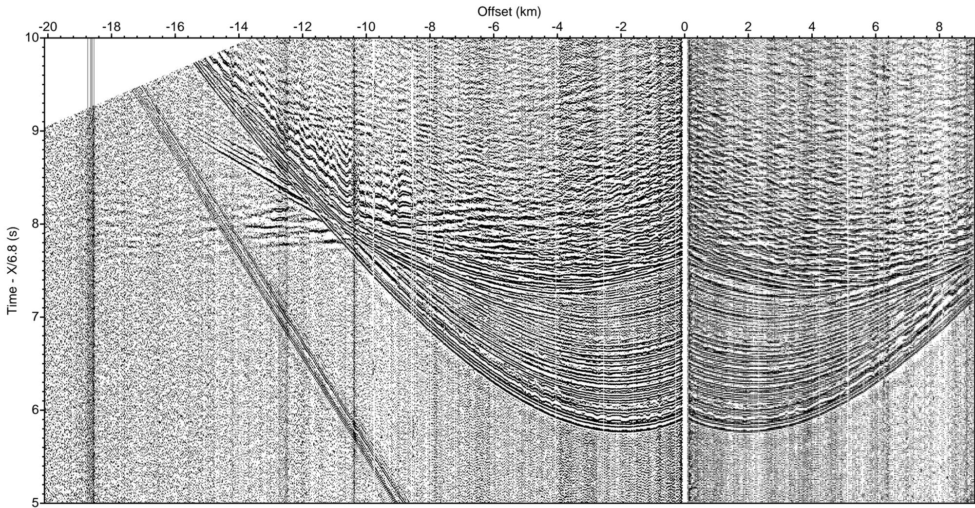
LOMROG III (2012) - Line 9 Sonobuoy 9-28 aux ch 4 (drift correction, deconv., bpf 5-40 Hz)
