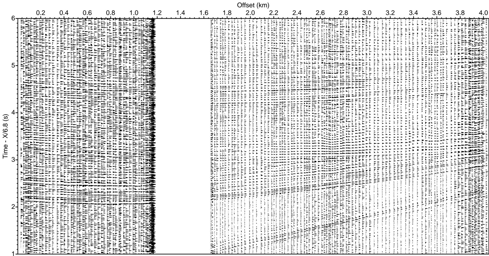
LOMROG III (2012) - Line 5 Sonobuoy 5-14 aux ch 1 (drift correction, deconv., bpf 5-40 Hz)
