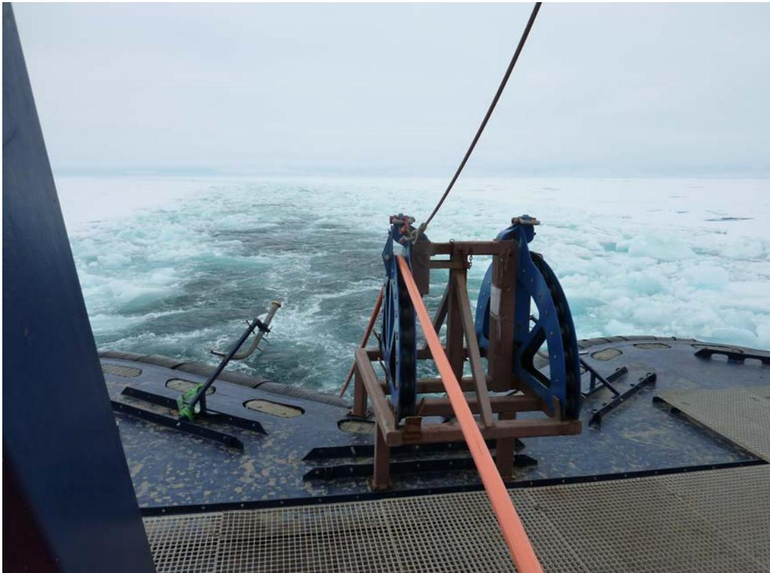
**Figure 20.** Photo from the aft deck during seismic data acquisition with the seismic equipment deployed.
