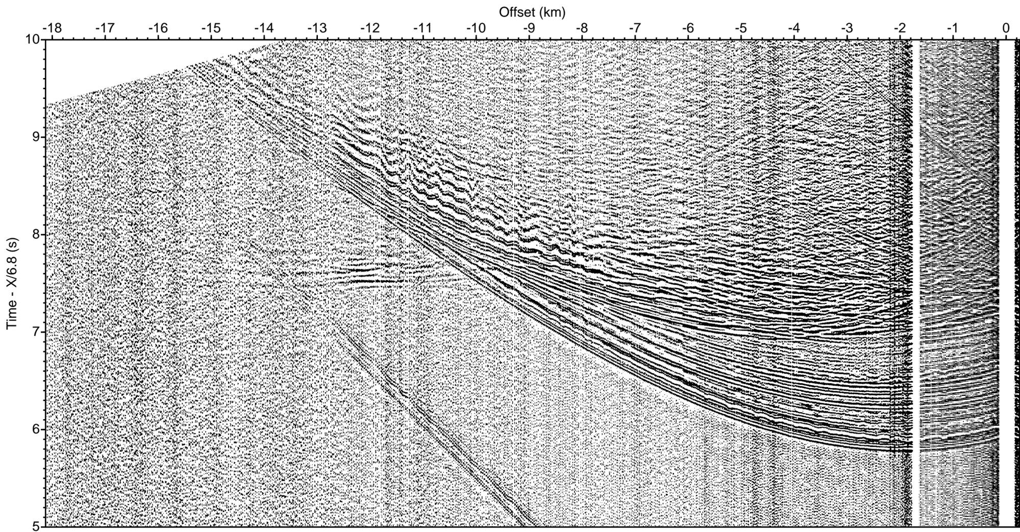
LOMROG III (2012) - Line 8 Sonobuoy 8-26 aux ch 3 (drift correction, deconv., bpf 5-40 Hz)
