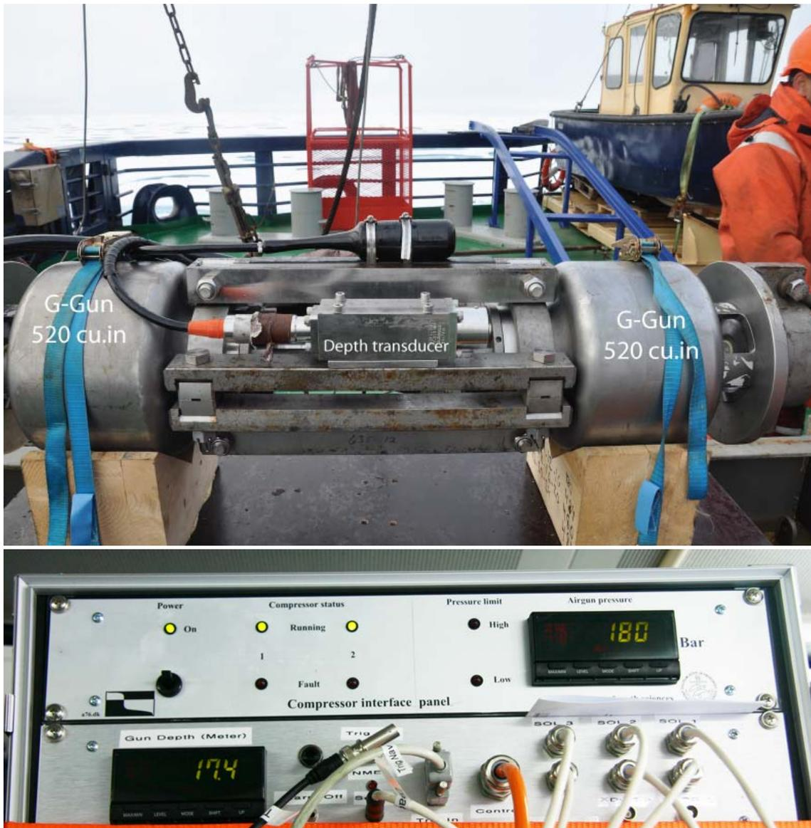
**Figure 2.** Sercel 1040 cu.in. linear airgun cluster (top). (Bottom) TGS-8 gun trigger unit (cables right side of lower panel), gun depth monitor (left side of lower panel). Compressor monitor and air gun pressure (upper panel).
