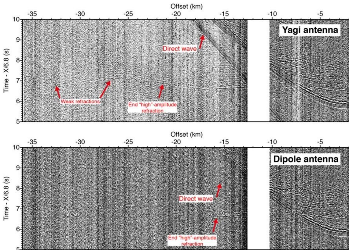
**Figure 36.** Comparison of the Yagi (top) and dipole (bottom) antenna for the signals transmitted by sonobuoy 1-2 on Line 1. The records are displayed with a reduction velocity of 6.8 km/s. Processing includes debias, deconvolution, bandpass filter (5-40 Hz) and scaling by true amplitude.
