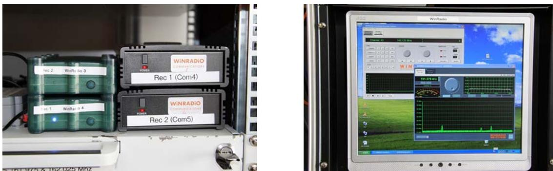
**Figure 25.** Sonobuoy receiving system. The two older Winradios (type WR-2902e; black boxes) are controlled by Winradio software (upper left window on computer display). The two newer Winradios (type WR-G39WSB; green boxes) were controlled by the Winradio software in the lower right window on the computer display.
