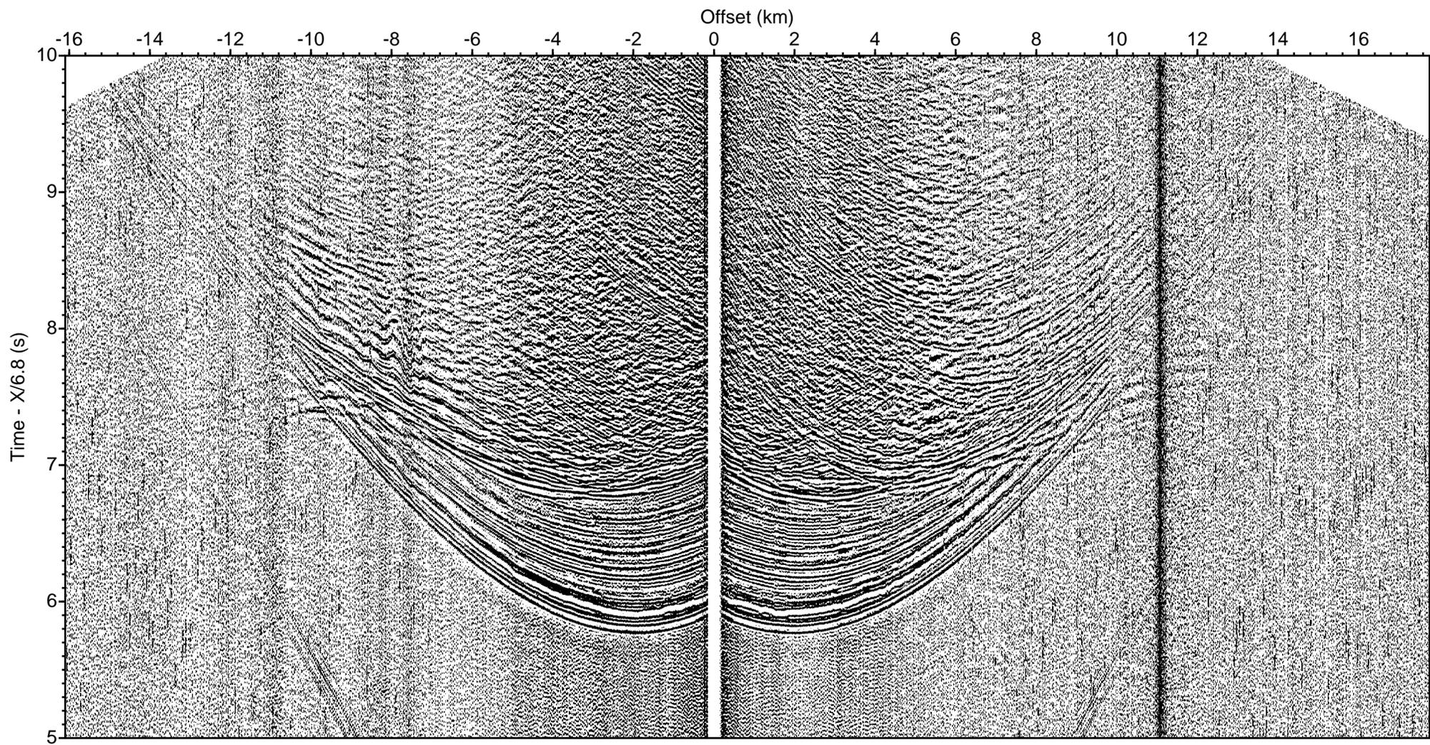
LOMROG III (2012) - Line 7 Sonobuoy 7-21 aux ch 2 (drift correction, deconv., bpf 5-40 Hz)
