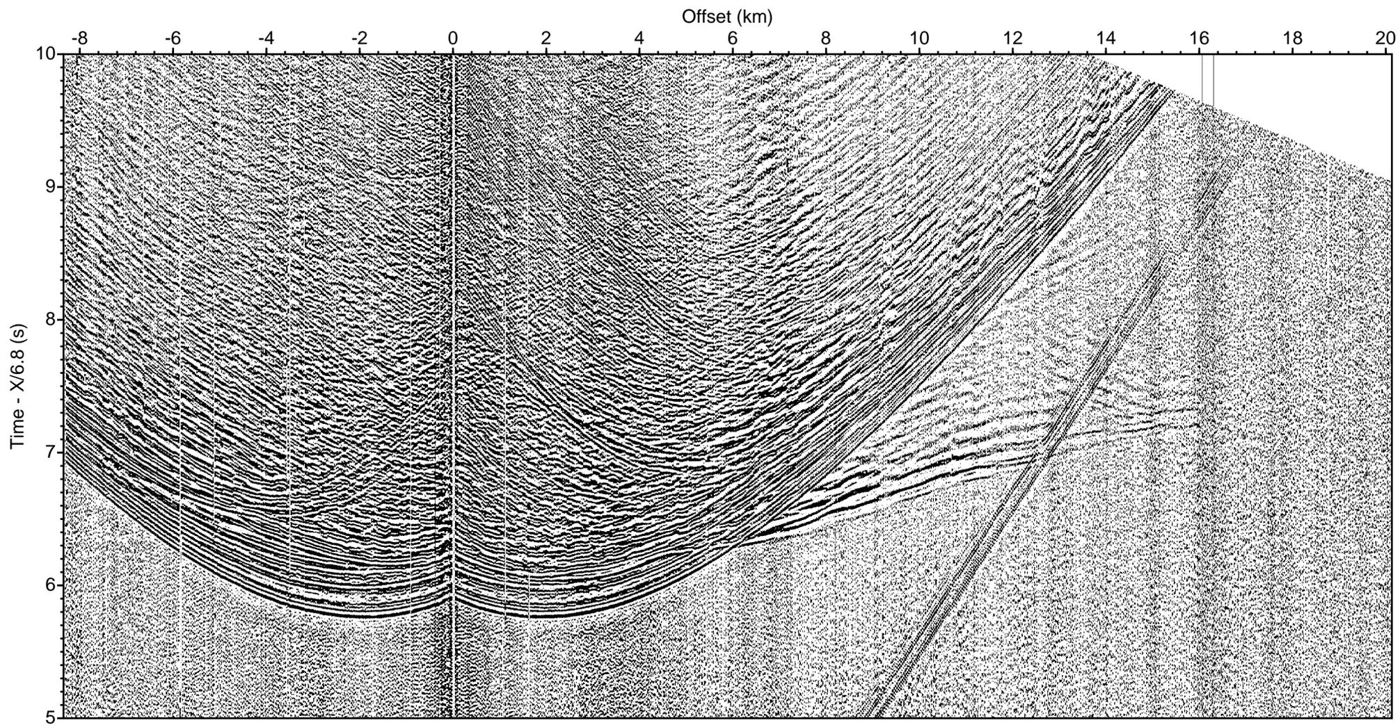
LOMROG III (2012) - Line 15 Sonobuoy 15-53 aux ch 4 (drift correction, deconv., bpf 5-40 Hz)
