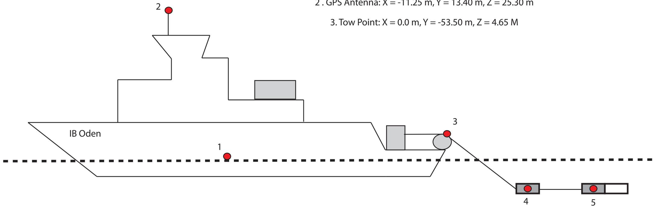
4. Airgun midpoint relative to tow point:  $X = 0.0 \text{ m}, Y = -17.85 \text{ m}, Z = -20.00 \text{ m}$
