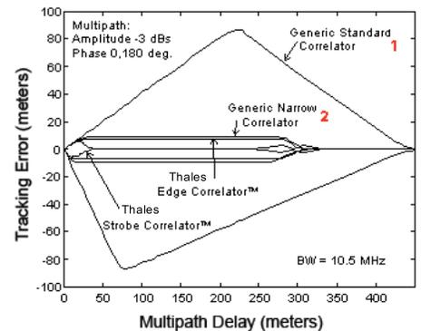
The horizontal axis of the plot shows the multipath delay, this is the extra distance that the reflected signal travels compared to the direct signal. The vertical axis shows the induced range error caused by a multipath signal with the indicated delay.
