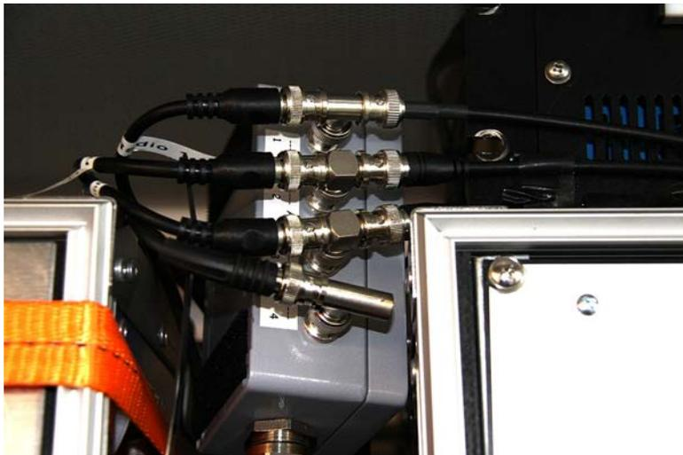
**Figure 27.** The output signal of the Winradio was split to go to the auxiliary channels (1 through 4) on the Geometrics recording system and to the Taurus seismometer (cables to the right). Note: The fourth Winradio is not recorded on the Taurus.
