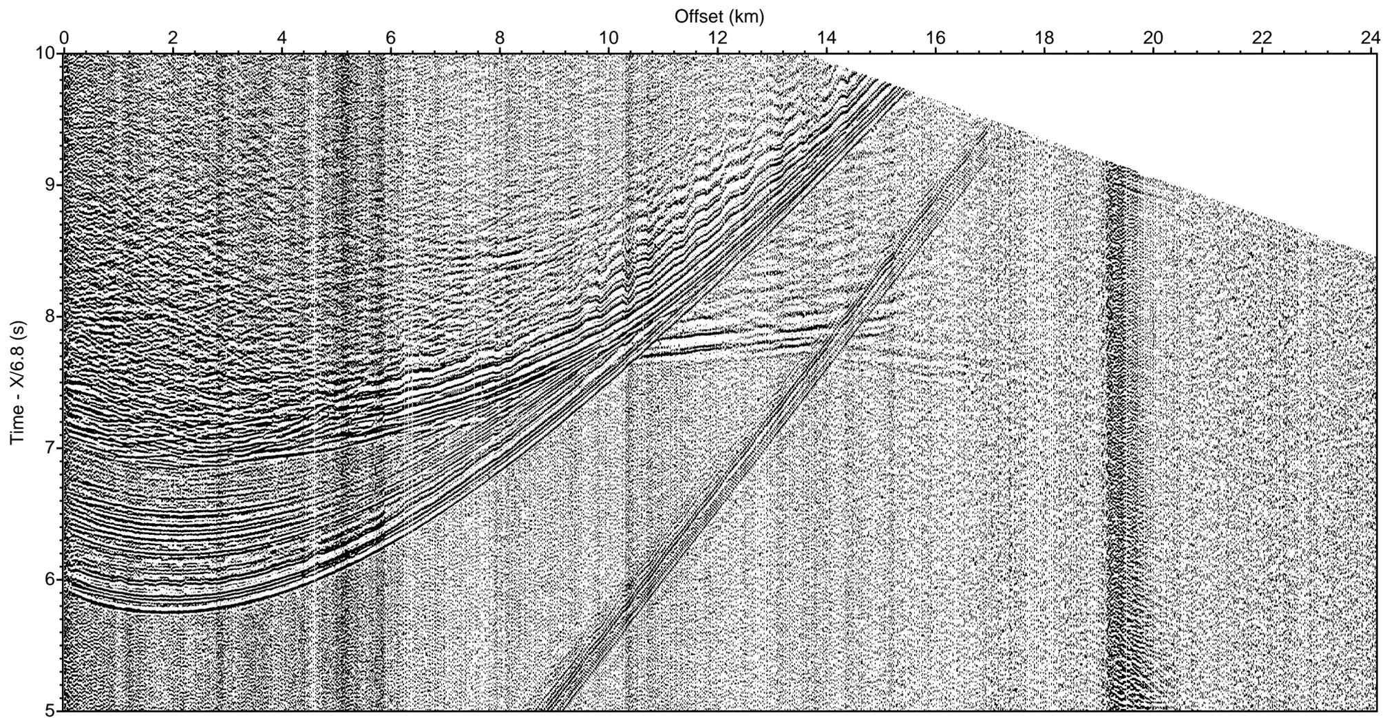
LOMROG III (2012) - Line 8 Sonobuoy 8-23 aux ch 1 (drift correction, deconv., bpf 5-40 Hz)
