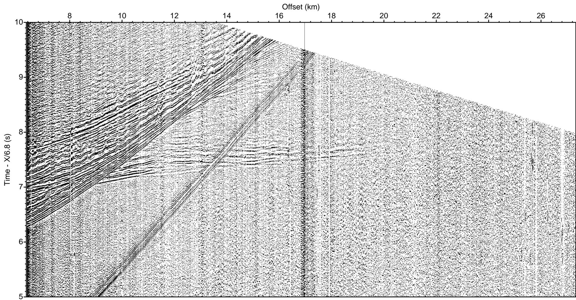
LOMROG III (2012) - Line 2 Sonobuoy 2-9 aux ch 1 (drift correction, deconv., bpf 5-40 Hz)
