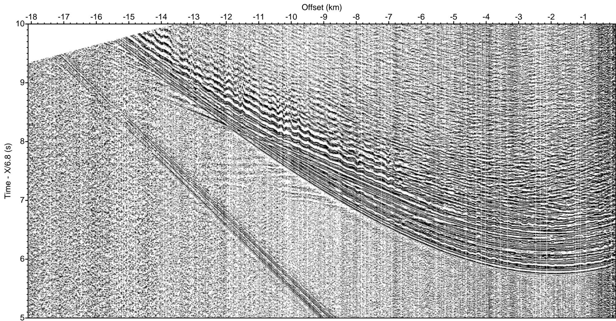
LOMROG III (2012) - Line 13 Sonobuoy 13-47 aux ch 3 (drift correction, deconv., bpf 5-40 Hz)
