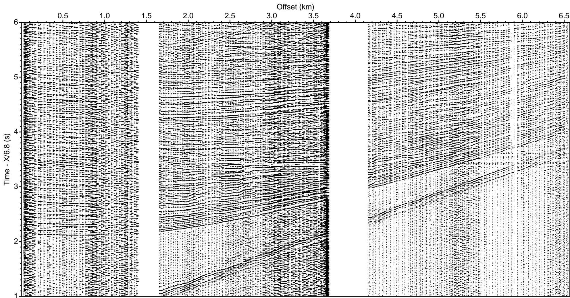
LOMROG III (2012) - Line 5 Sonobuoy 5-13 aux ch 1 (drift correction, deconv., bpf 5-40 Hz)
