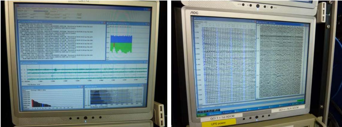
**Figure 5.** Seismic controller display facilities: noise window, trigger window and log window (left) and shot gather window, brute stack window and a streamer depth window (right).
