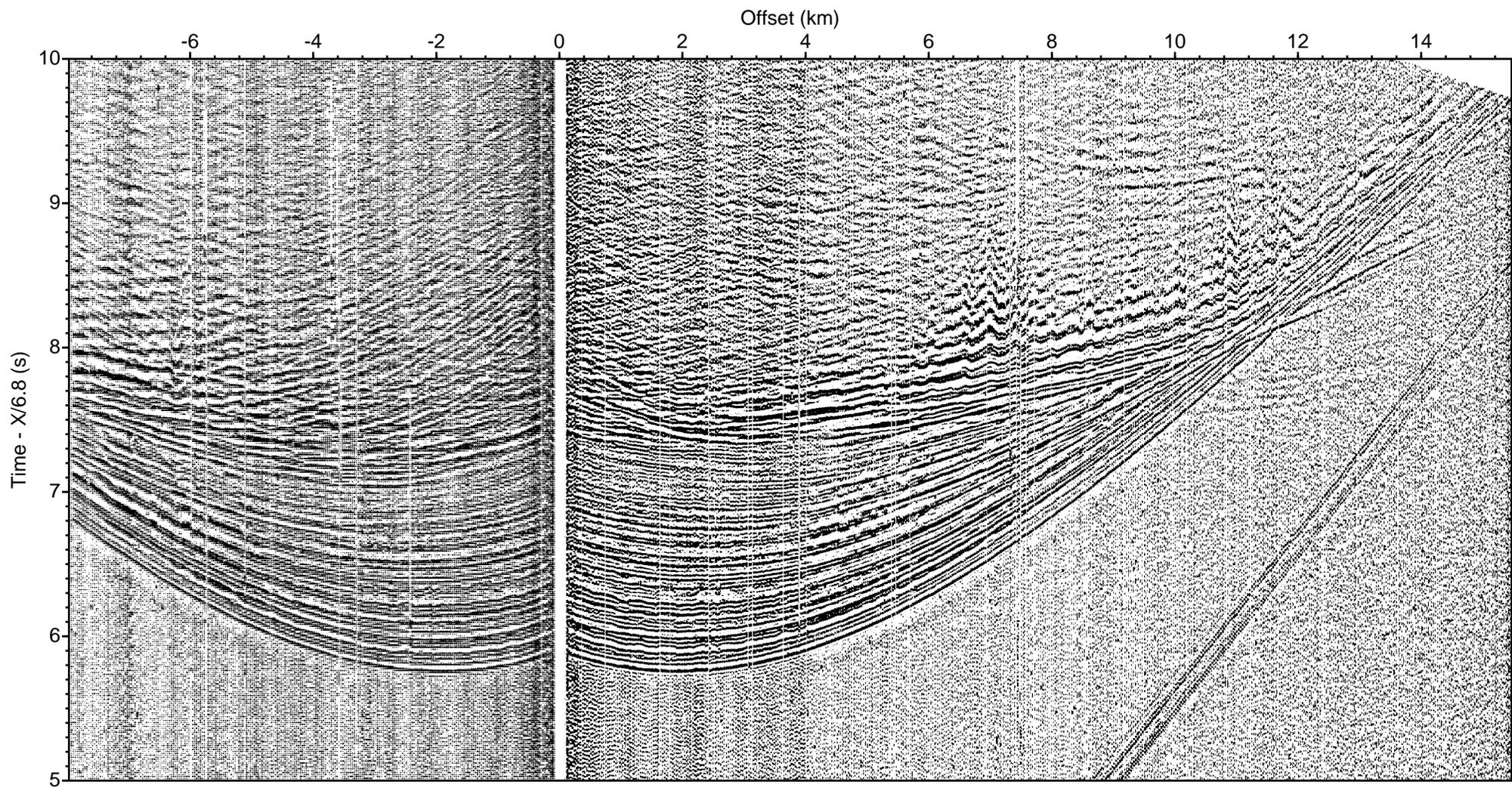
LOMROG III (2012) - Line 13 Sonobuoy 13-45 aux ch 4 (drift correction, deconv., bpf 5-40 Hz)
