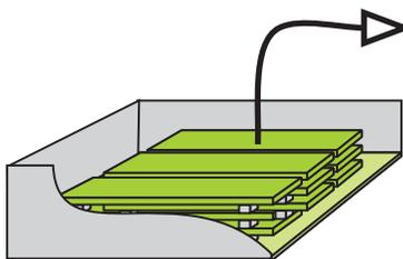
When its time to replace your old analog sections, the GeoEel boards are redeployed in the waterproof canisters used in the in-water digital streamer
