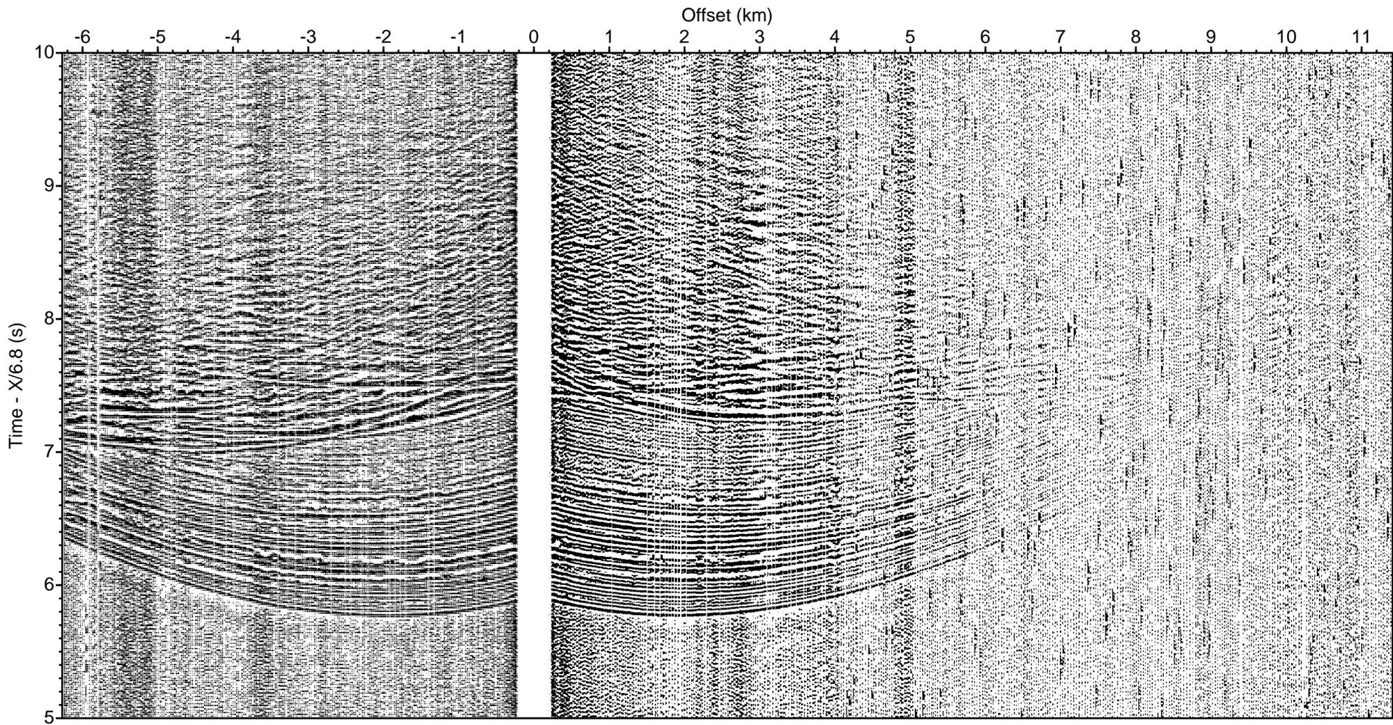
LOMROG III (2012) - Line 16 Sonobuoy 16-58 aux ch 2 (drift correction, deconv., bpf 5-40 Hz)
