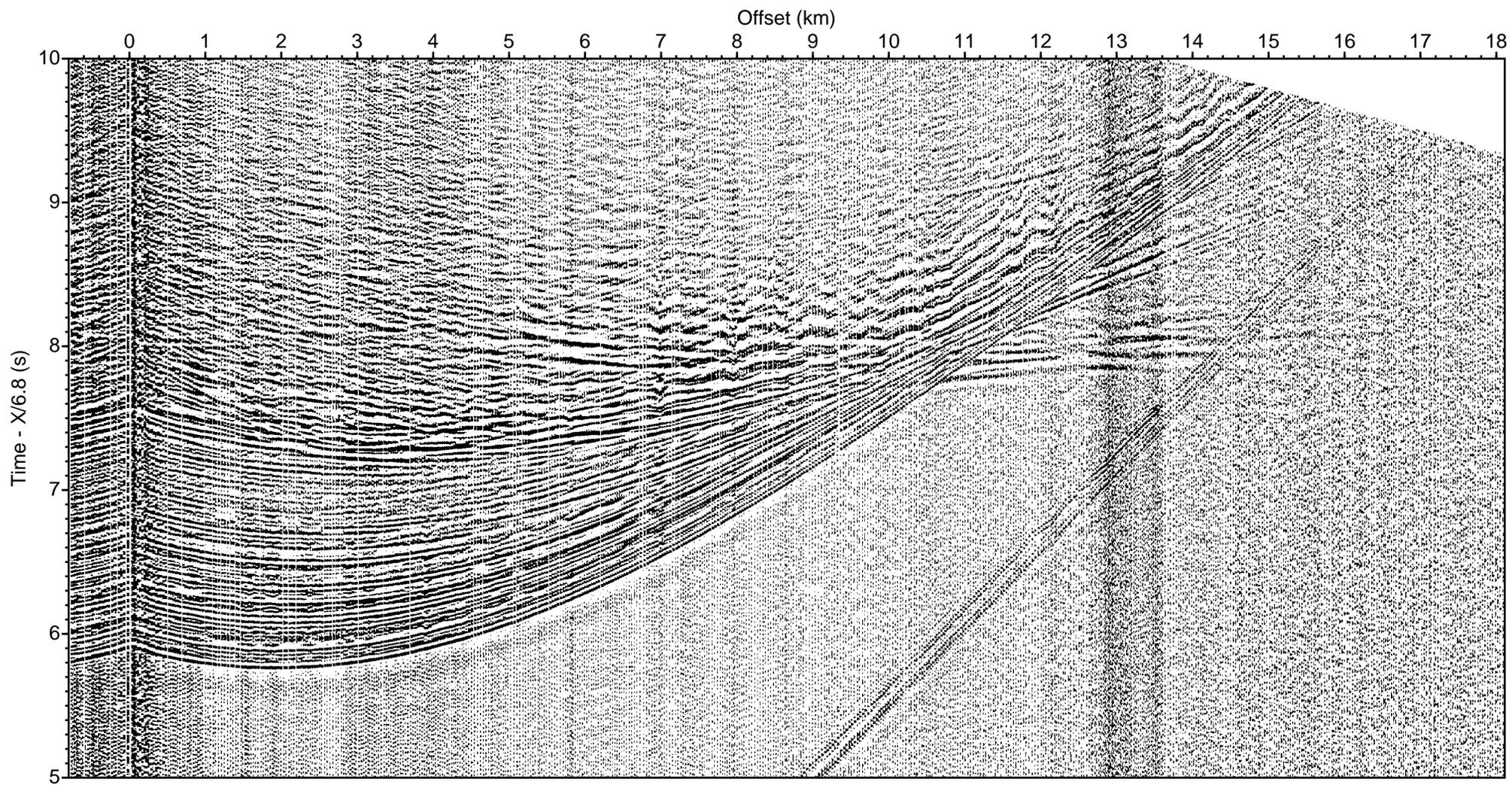
LOMROG III (2012) - Line 14 Sonobuoy 14-51 aux ch 3 (drift correction, deconv., bpf 5-40 Hz)
