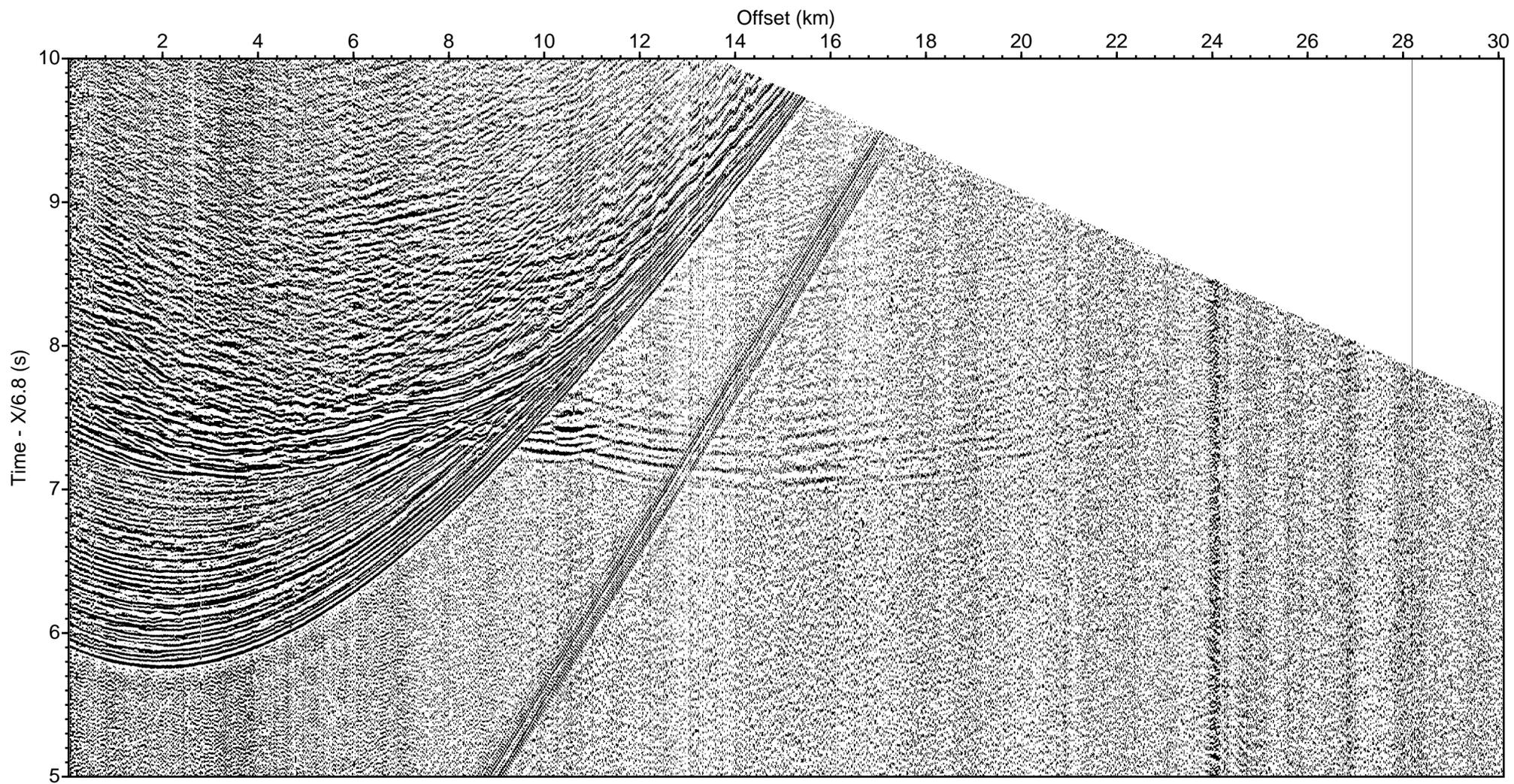
LOMROG III (2012) - Line 15 Sonobuoy 15-52 aux ch 1 (drift correction, deconv., bpf 5-40 Hz)
