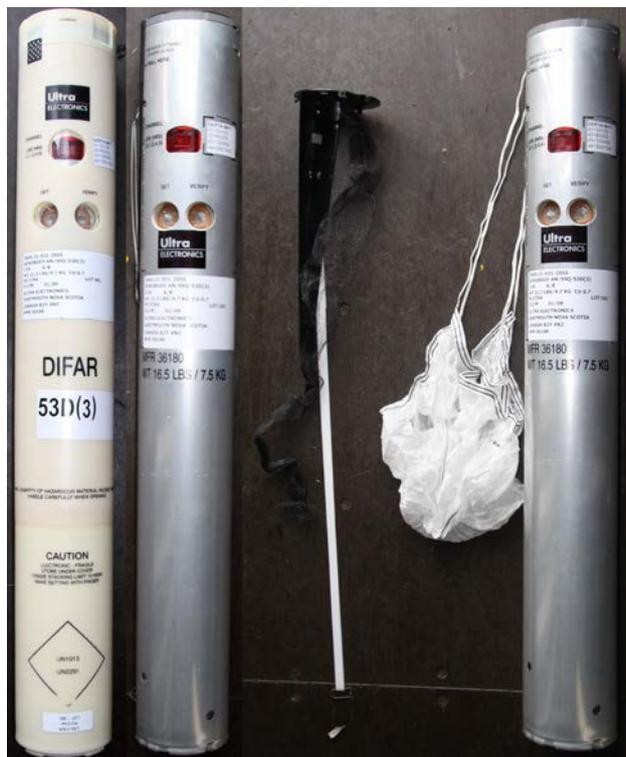
**Figure 23.** Sonobuoy type AN/SSQ-53D(3) from ULTRA Electronics. The left part of the image shows the sonobuoy in the hermetically sealed buoy launch container. In the centre, the buoy is shown after removal of the storage container. The right part of the picture provides a view on the sonobuoy with the top cap (lanyard) removed, where the parachute is stored. The buoy is deployed in this state.
