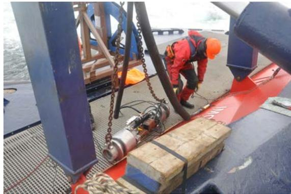
**Figure 14.** Air gun array on aft deck. Streamer sheave in the background (port side).
