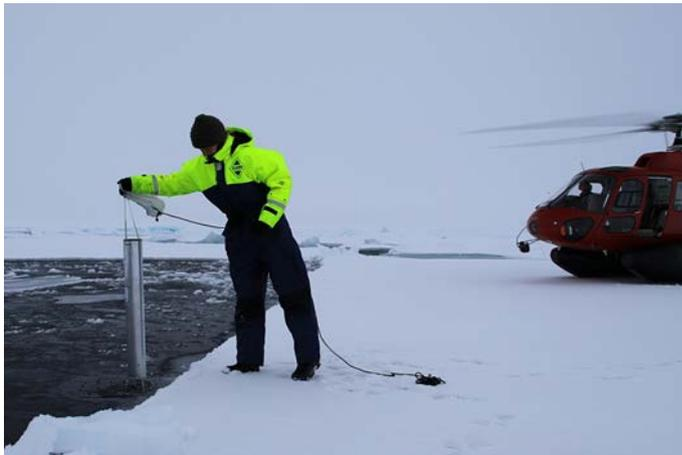
**Figure 31.** Deployment of a sonobuoy close to the prepared track for the seismic line. The helicopter is used for transportation and for finding suitable open water. A rope is attached to the parachute of the sonobuoy.
