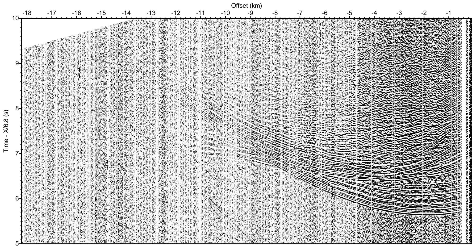
LOMROG III (2012) - Line 2 Sonobuoy 2-8 aux ch 2 (drift correction, deconv., bpf 5-40 Hz)
