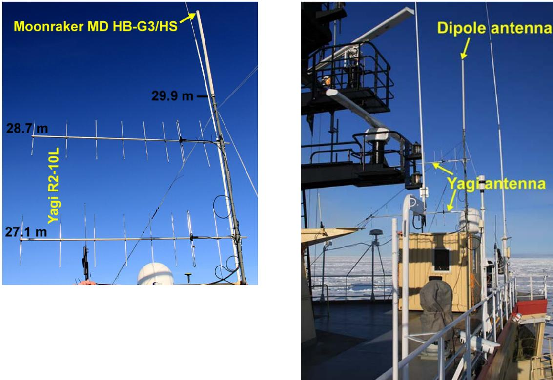
**Figure 24.** Dipole antenna MD HB-G3/HS and Yagi antenna R2-10L mounted on top of the bridge of Oden on the port side. Numbers on the left indicate the antenna heights above sea level.
