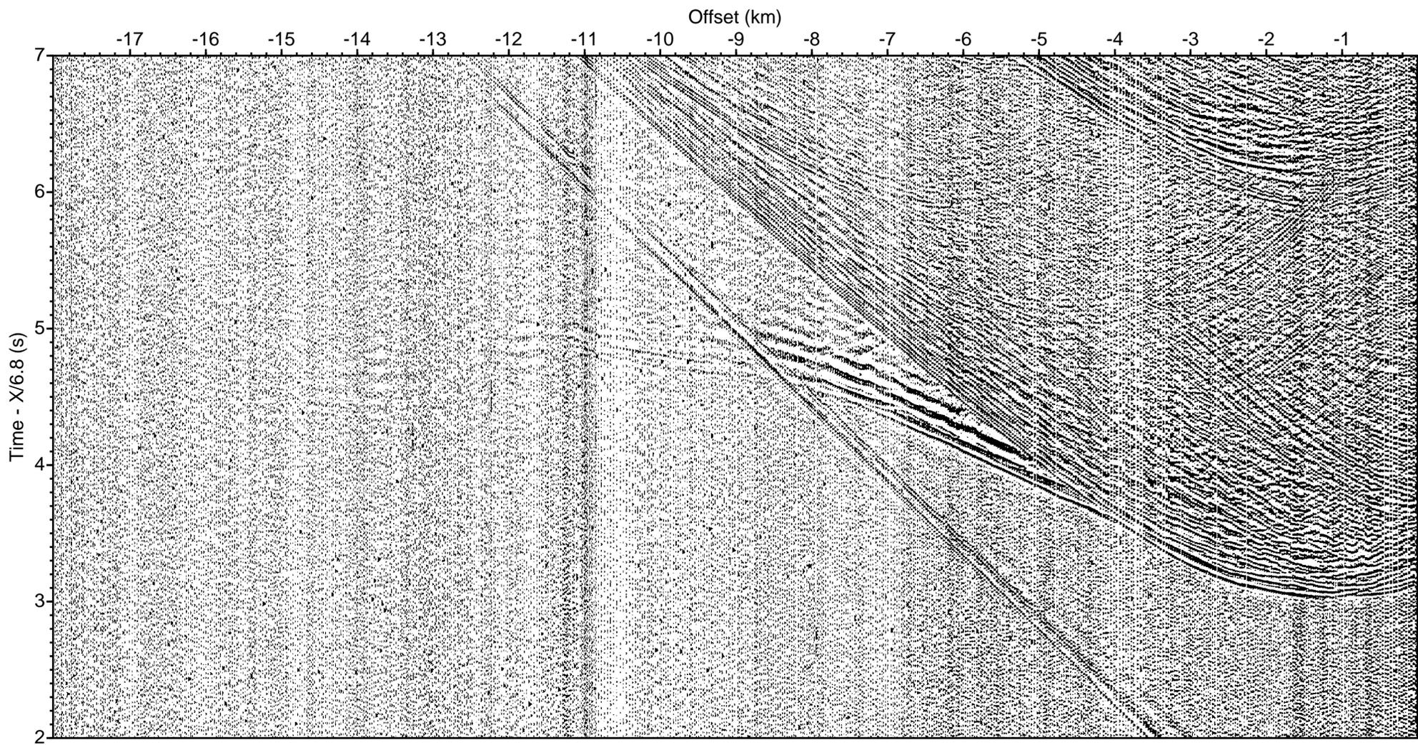
LOMROG III (2012) - Line 6 Sonobuoy 6-15 aux ch 1 (drift correction, deconv., bpf 5-40 Hz)
