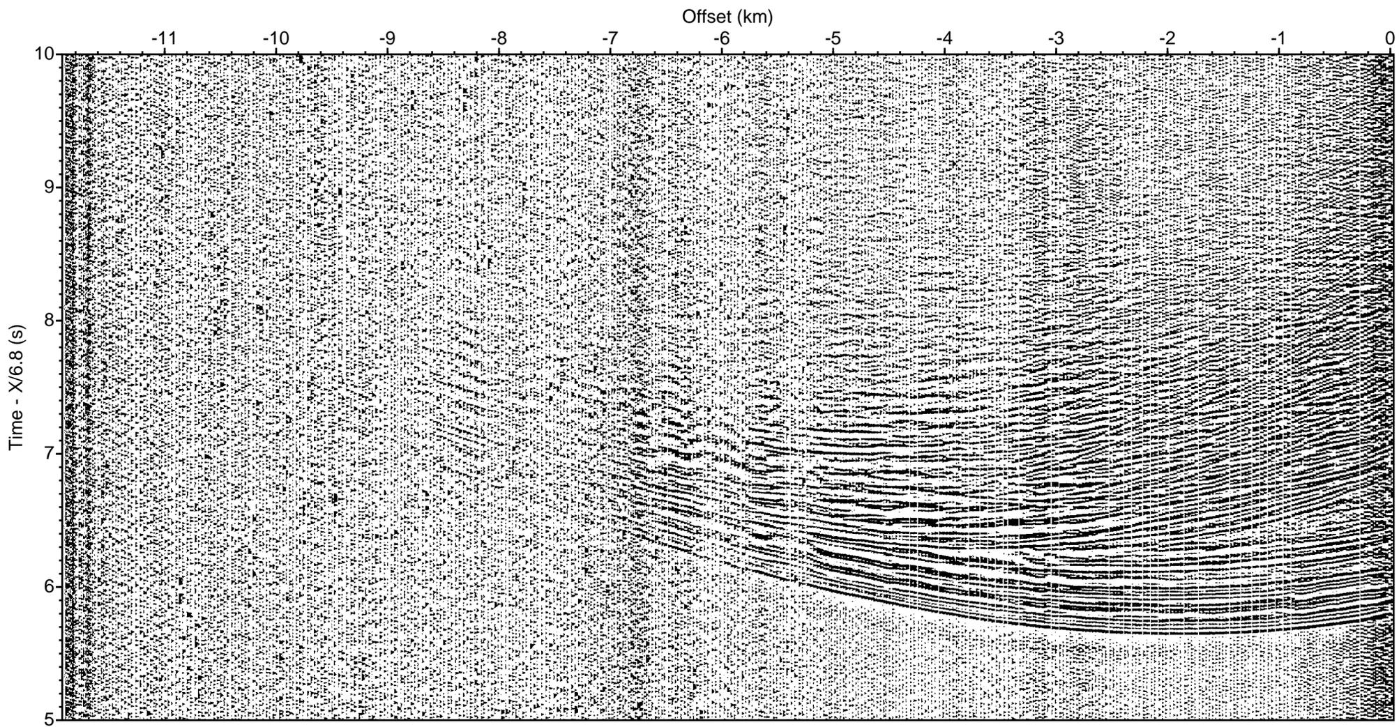
LOMROG III (2012) - Line 1 Sonobuoy 1-5 aux ch 4 (drift correction, deconv., bpf 5-40 Hz)
