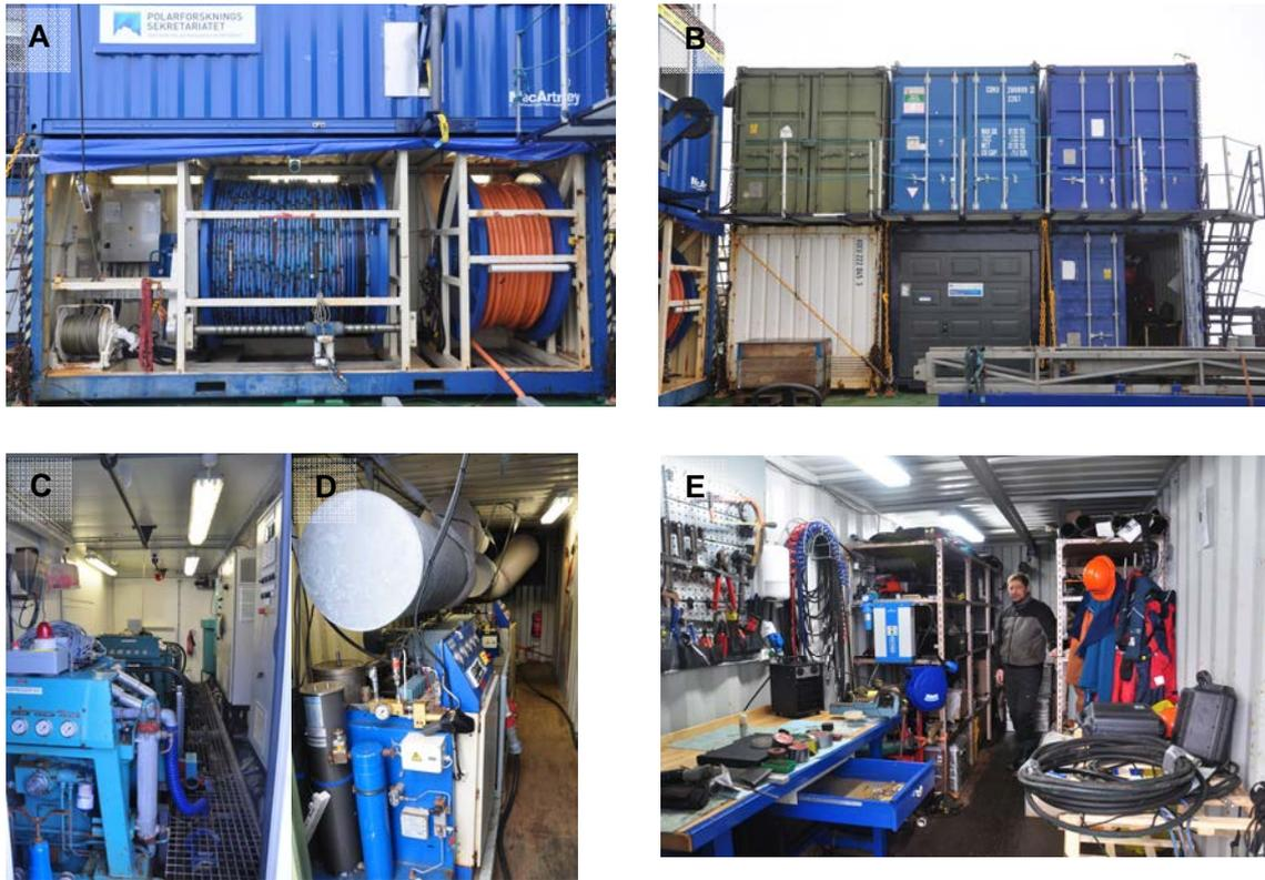
**Figure 9.** Containers on aft deck: (A) winch container; (B) compressor containers (white and green), storage containers (blue) in the upper layer and workshop container (blue) in the lower layer to the right; interior of compressor container: (C) Hamworthy and (D) Bauer compressors; (E) interior of workshop container.
