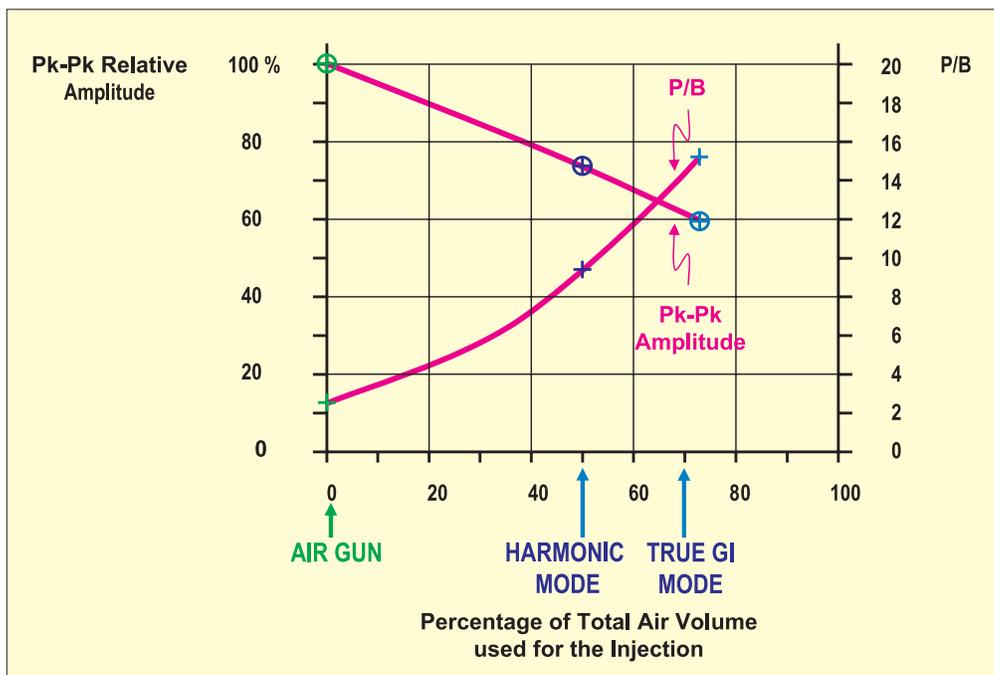
When the Injector has about the same volume as the Generator, the oscillation of the bubble created:
