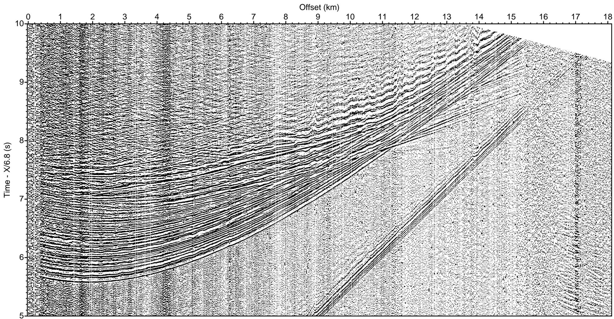
LOMROG III (2012) - Line 13 Sonobuoy 13-44 aux ch 1 (drift correction, deconv., bpf 5-40 Hz)
