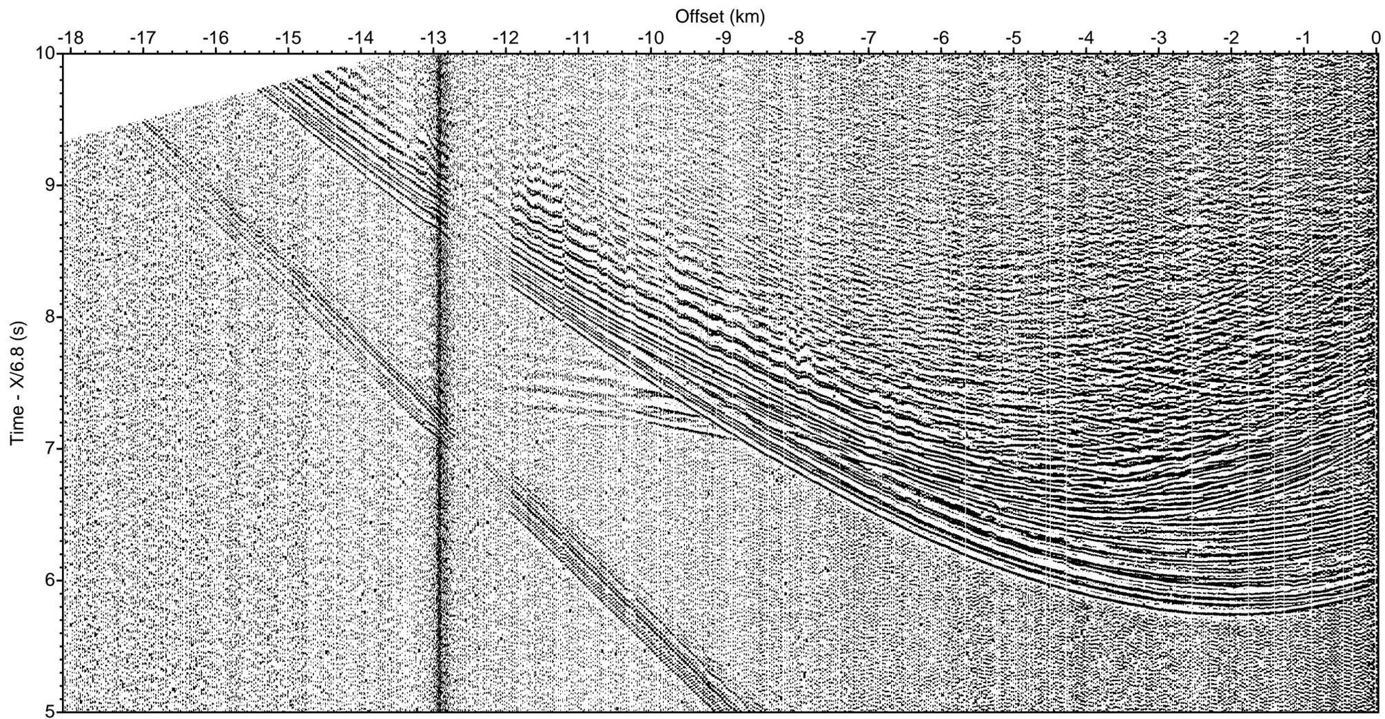
LOMROG III (2012) - Line 7 Sonobuoy 7-19 aux ch 1 (drift correction, deconv., bpf 5-40 Hz)
