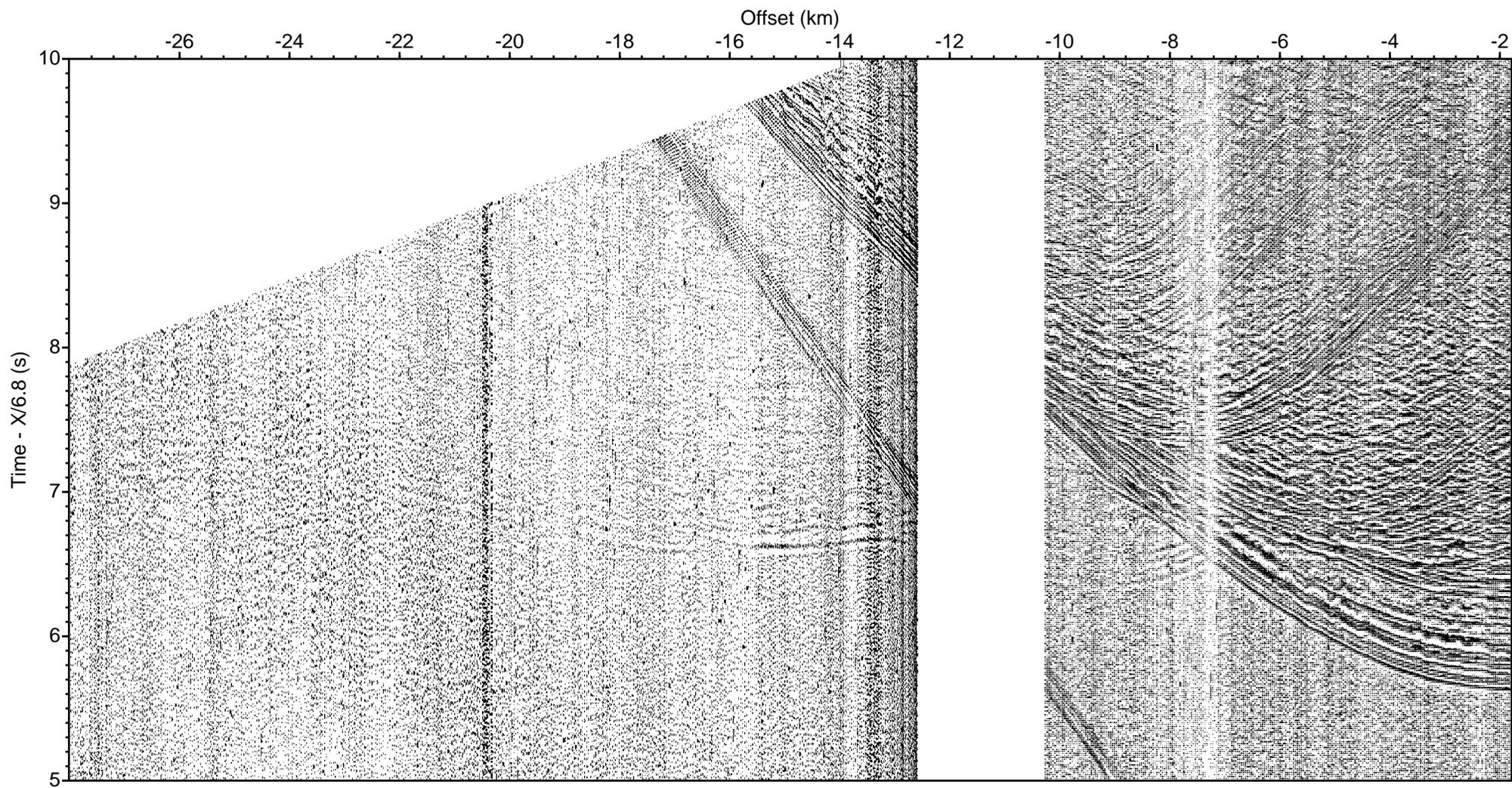
LOMROG III (2012) - Line 1 Sonobuoy 1-2 aux ch 1 (drift correction, deconv., bpf 5-40 Hz)
