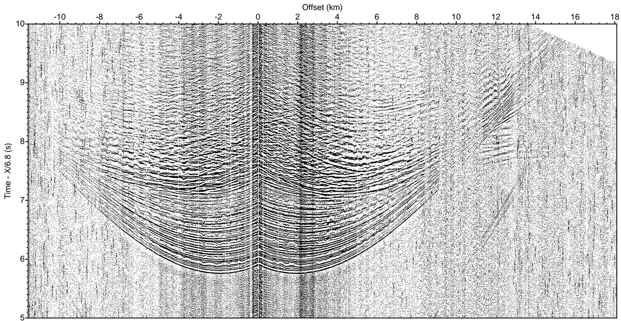
LOMROG III (2012) - Line 14 Sonobuoy 14-50 aux ch 2 (drift correction, deconv., bpf 5-40 Hz)
