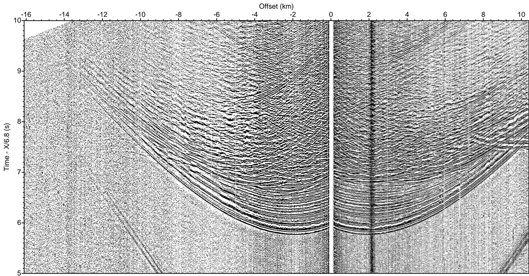
LOMROG III (2012) - Line 7 Sonobuoy 7-20 aux ch 4 (drift correction, deconv., bpf 5-40 Hz)
