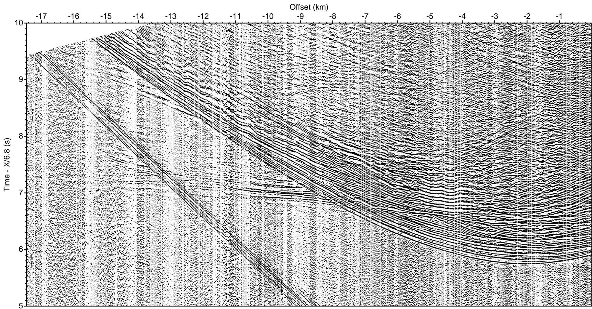
LOMROG III (2012) - Line 17 Sonobuoy 17-60 aux ch 1 (drift correction, deconv., bpf 5-40 Hz)
