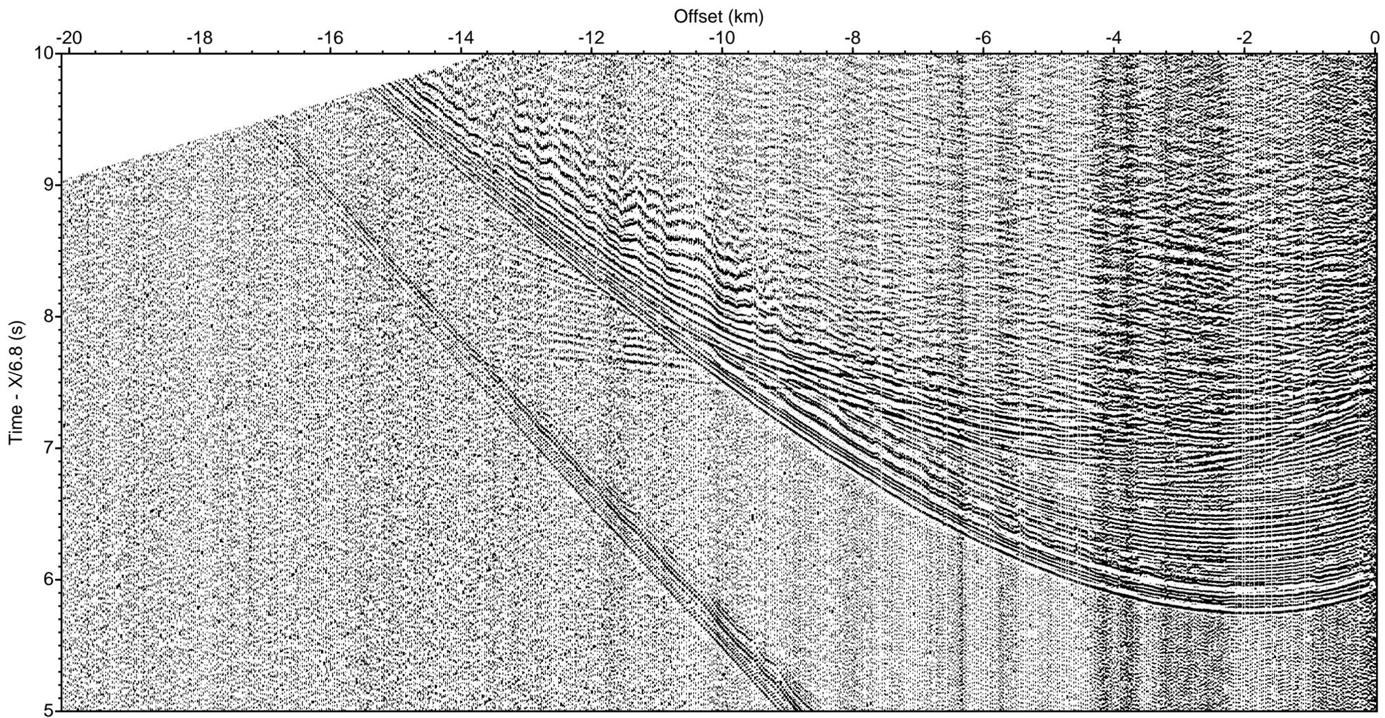
LOMROG III (2012) - Line 9 Sonobuoy 9-27 aux ch 1 (drift correction, deconv., bpf 5-40 Hz)
