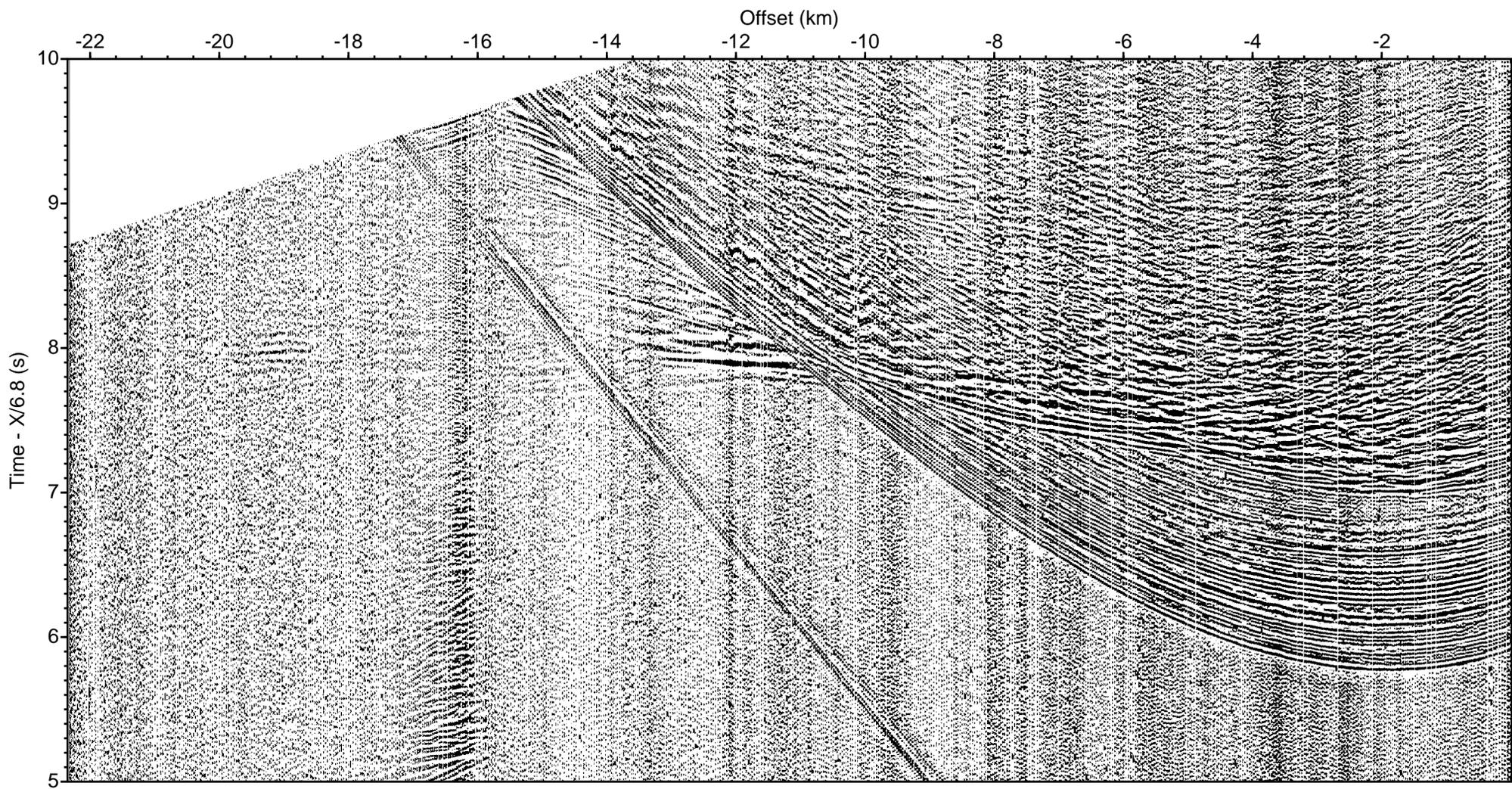
LOMROG III (2012) - Line 16 Sonobuoy 16-56 aux ch 1 (drift correction, deconv., bpf 5-40 Hz)
