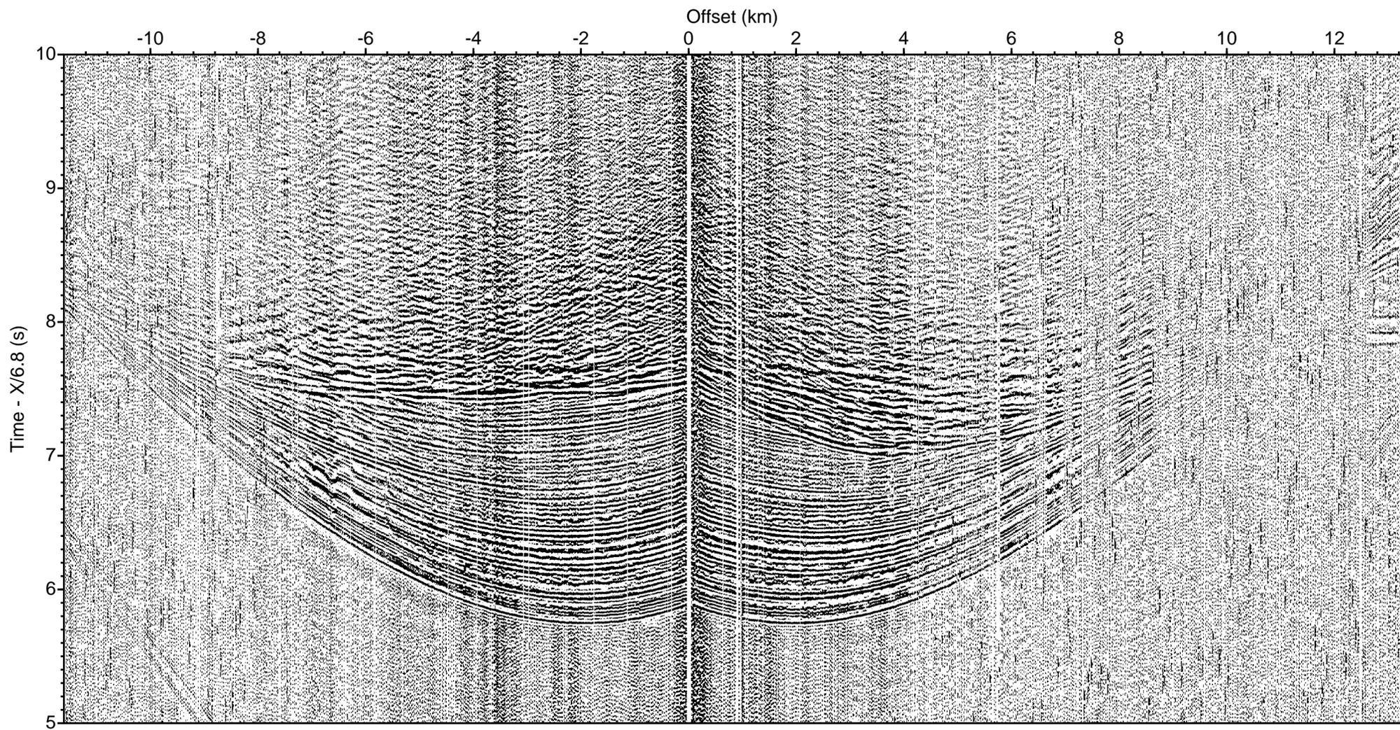
LOMROG III (2012) - Line 11 Sonobuoy 11-38 aux ch 2 (drift correction, deconv., bpf 5-40 Hz)
