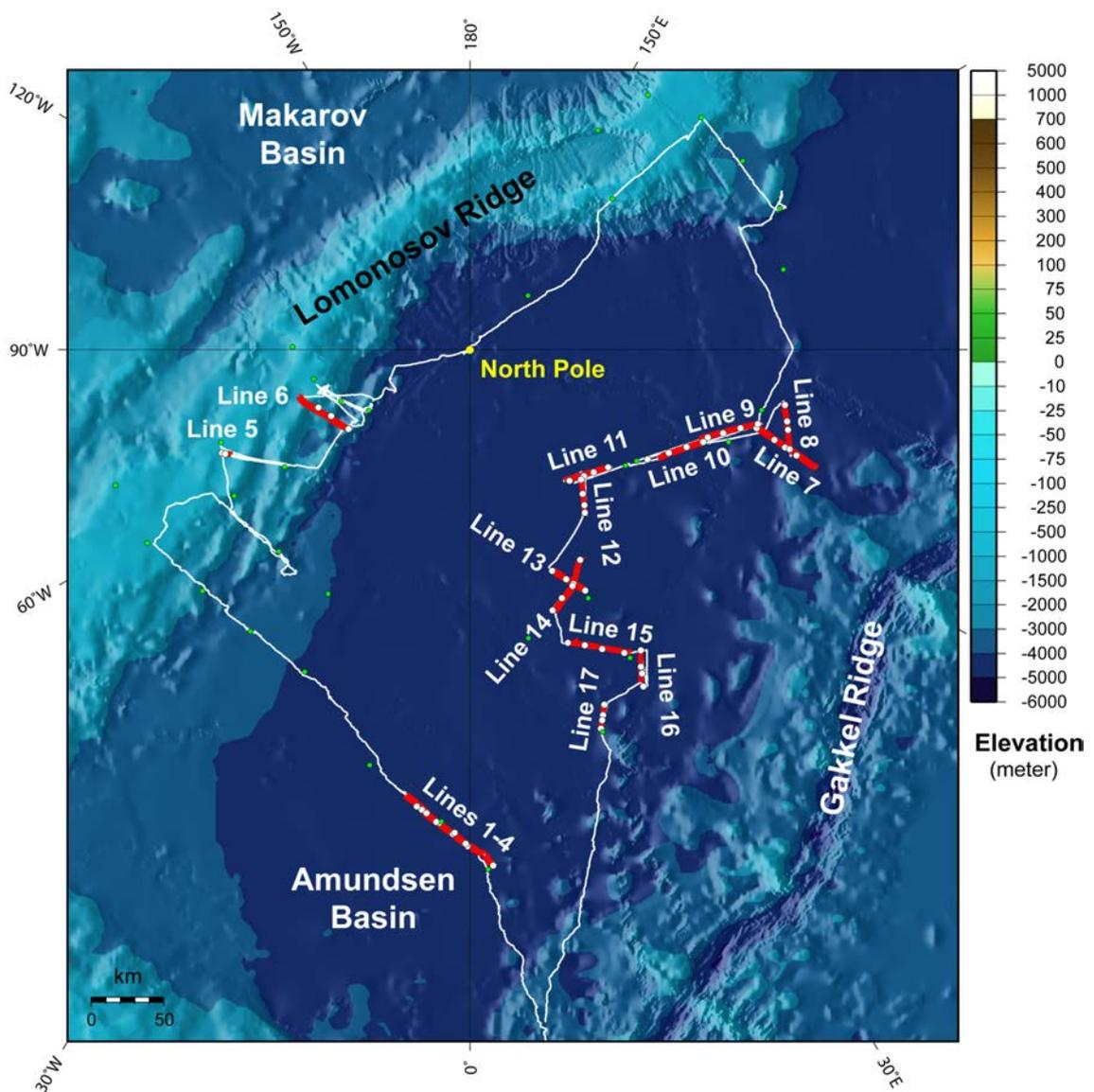
**Figure 33.** Bathymetric map (IBCAO 3.0, Jakobsson et al. 2012) with the location of the LOMROG III (2012) seismic reflection lines (red lines). The ship track is marked as white line. White circles indicate the deployment positions of functional sonobuoys. Green circles show the location of CTD measurements. Detailed location maps for individual lines are shown in Appendix V-B.
