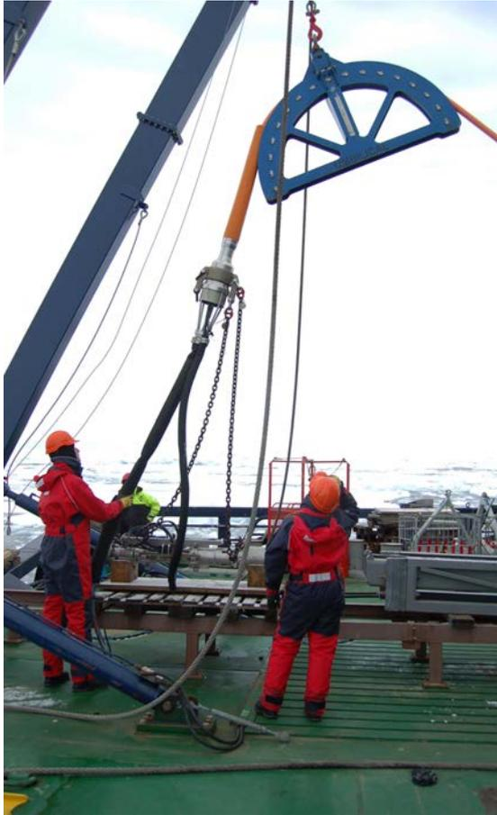
**Figure 13.** Umbilical and air guns lifted in the umbilical sheave.
