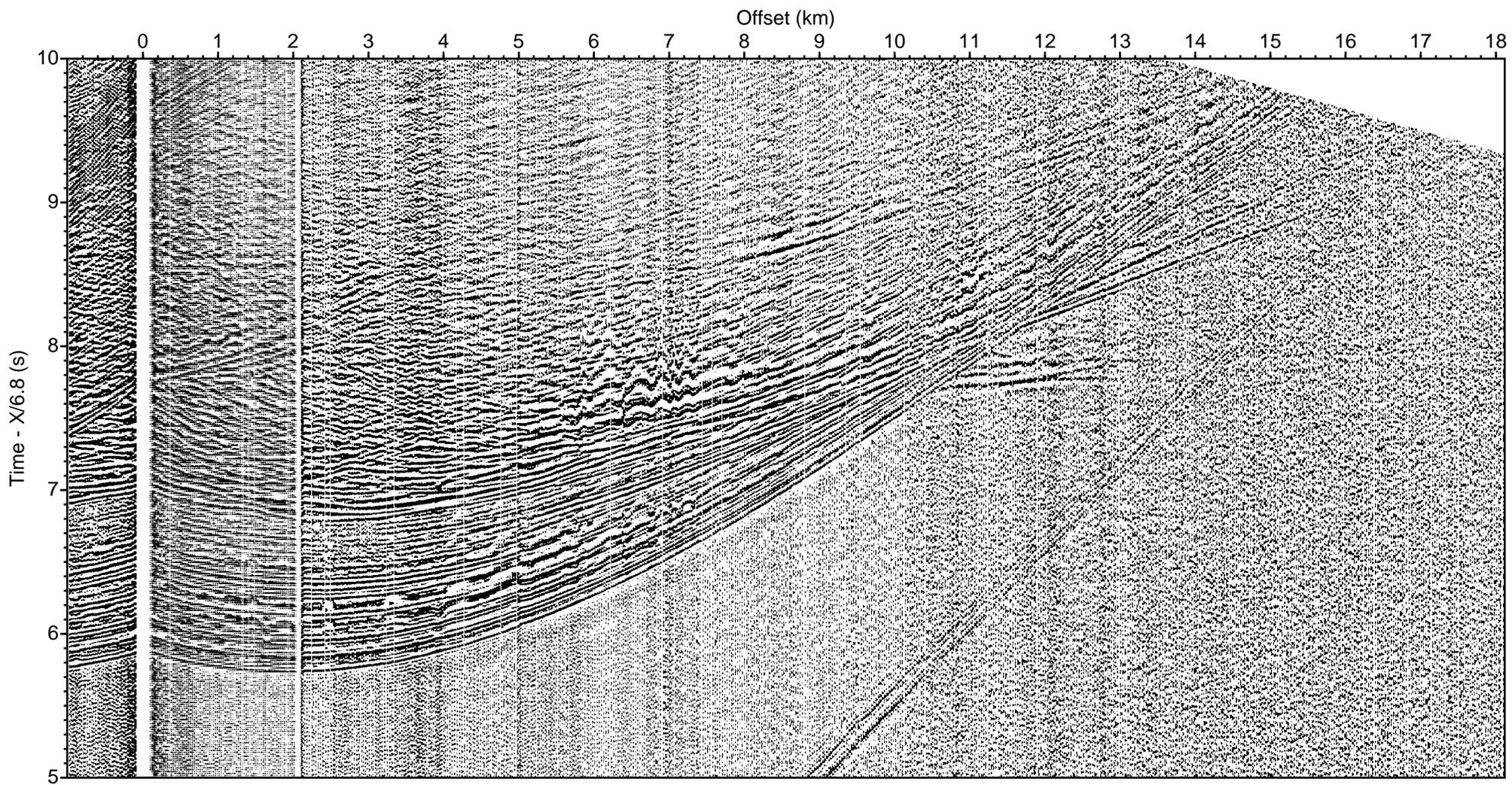
LOMROG III (2012) - Line 11 Sonobuoy 11-39 aux ch 3 (drift correction, deconv., bpf 5-40 Hz)
