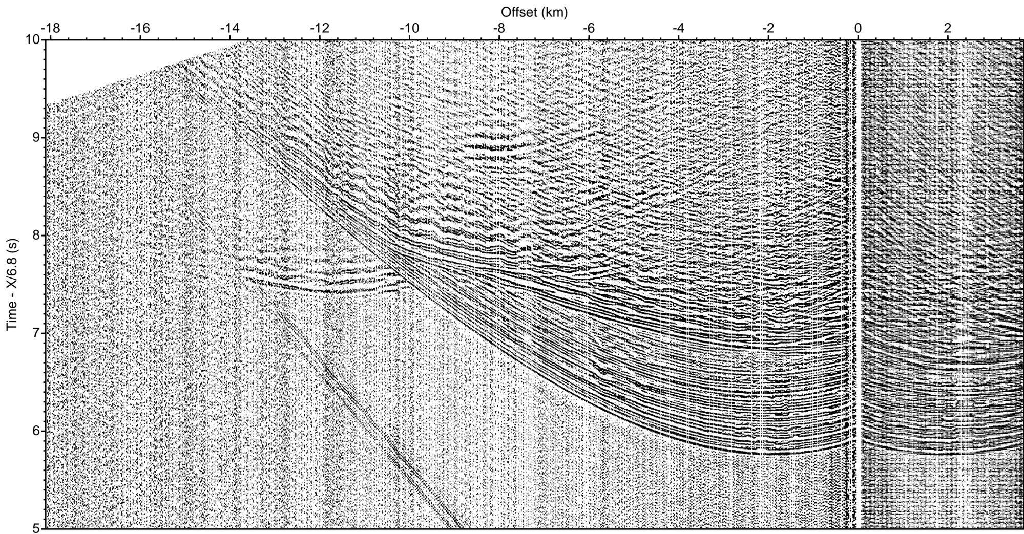
LOMROG III (2012) - Line 15 Sonobuoy 15-55 aux ch 3 (drift correction, deconv., bpf 5-40 Hz)
