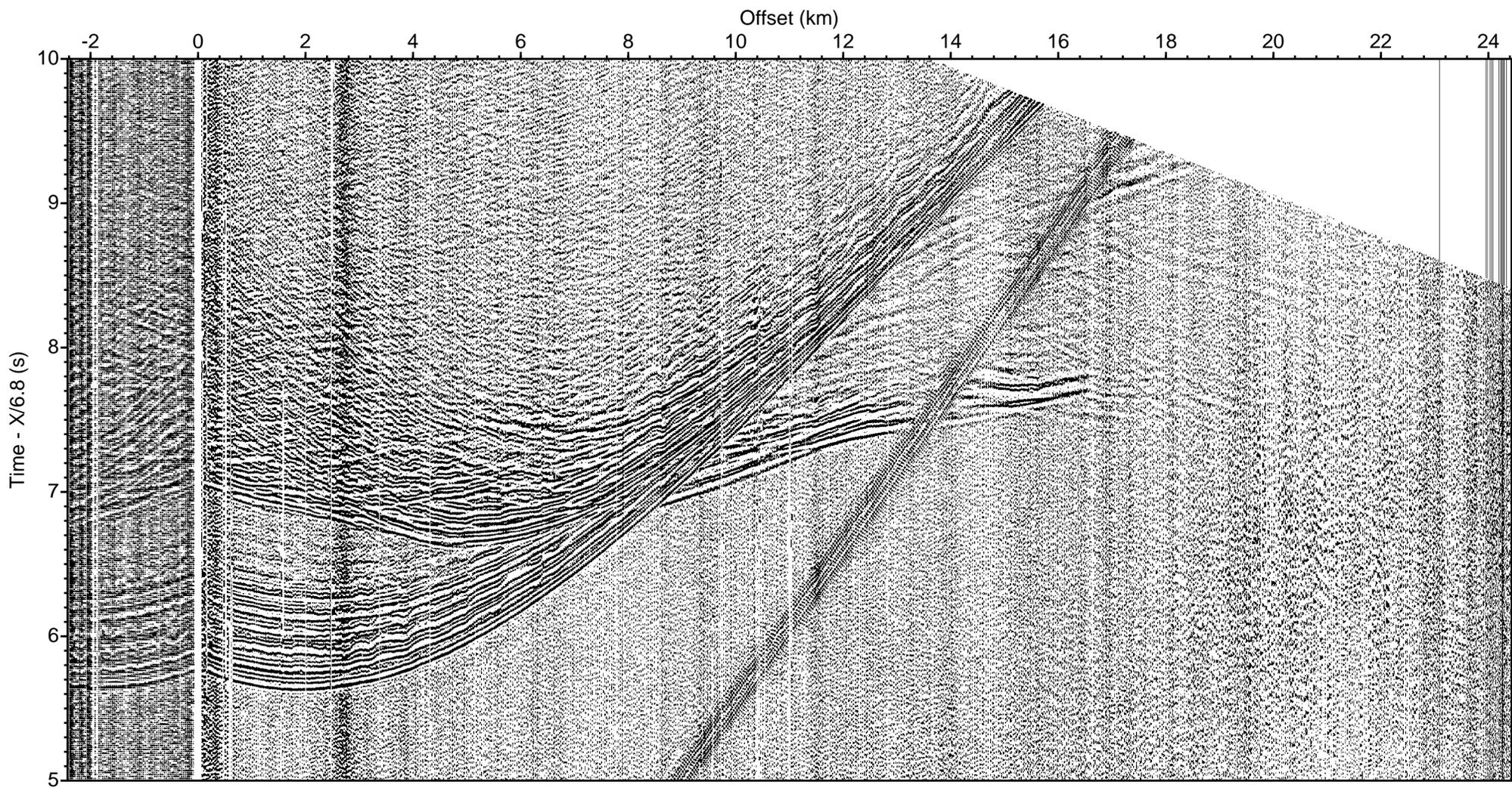
LOMROG III (2012) - Line 1 Sonobuoy 1-3 aux ch 3 (drift correction, deconv., bpf 5-40 Hz)
