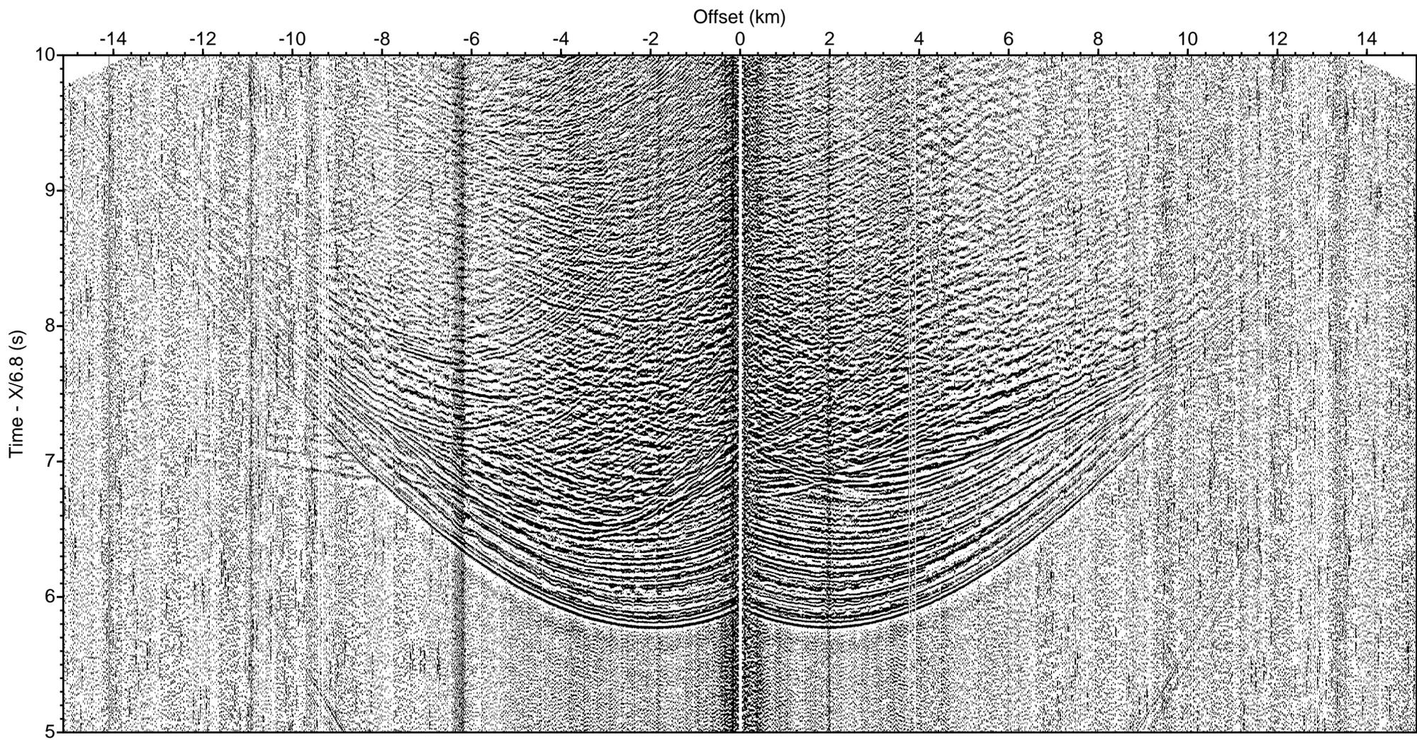
LOMROG III (2012) - Line 9 Sonobuoy 9-29 aux ch 2 (drift correction, deconv., bpf 5-40 Hz)
