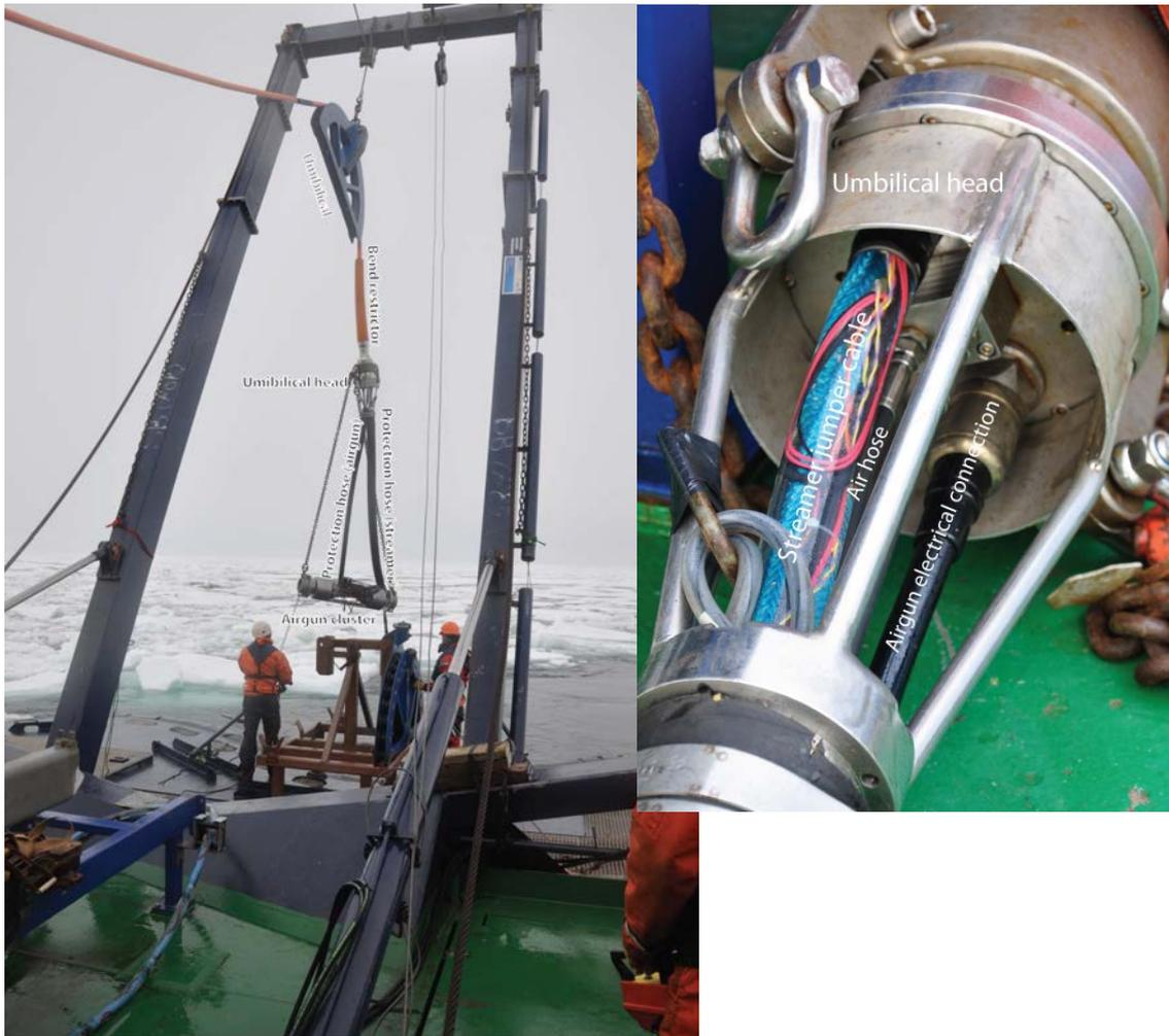
**Figure 12.** The sea end of the umbilical hanging in the A-frame (left) and close-up photo of the umbilical head (right).
