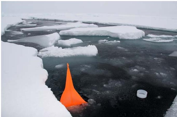
**Figure 32.** Sonobuoy that was deployed in a refrozen open water pond. The weight of the sonobuoy was sufficient to create the hole in the ice.
