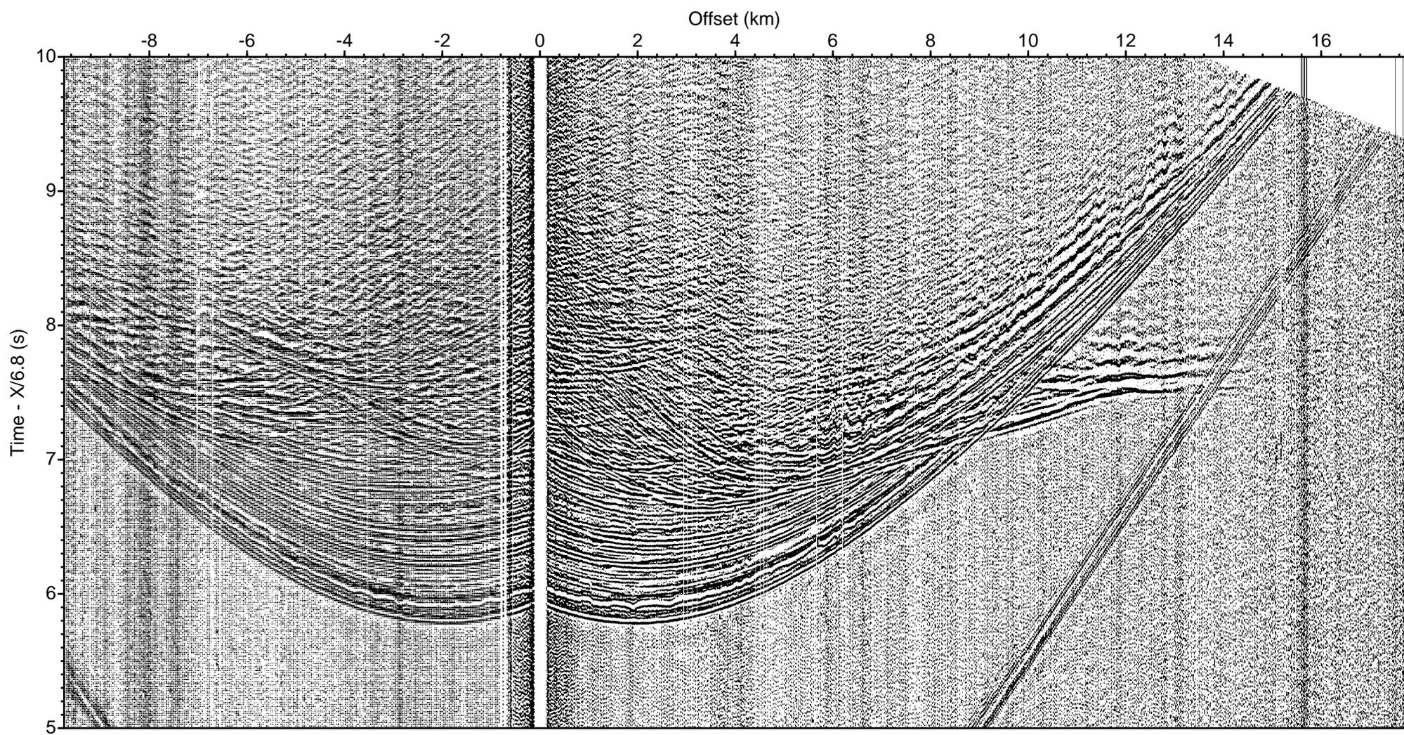
LOMROG III (2012) - Line 8 Sonobuoy 8-24 aux ch 4 (drift correction, deconv., bpf 5-40 Hz)
