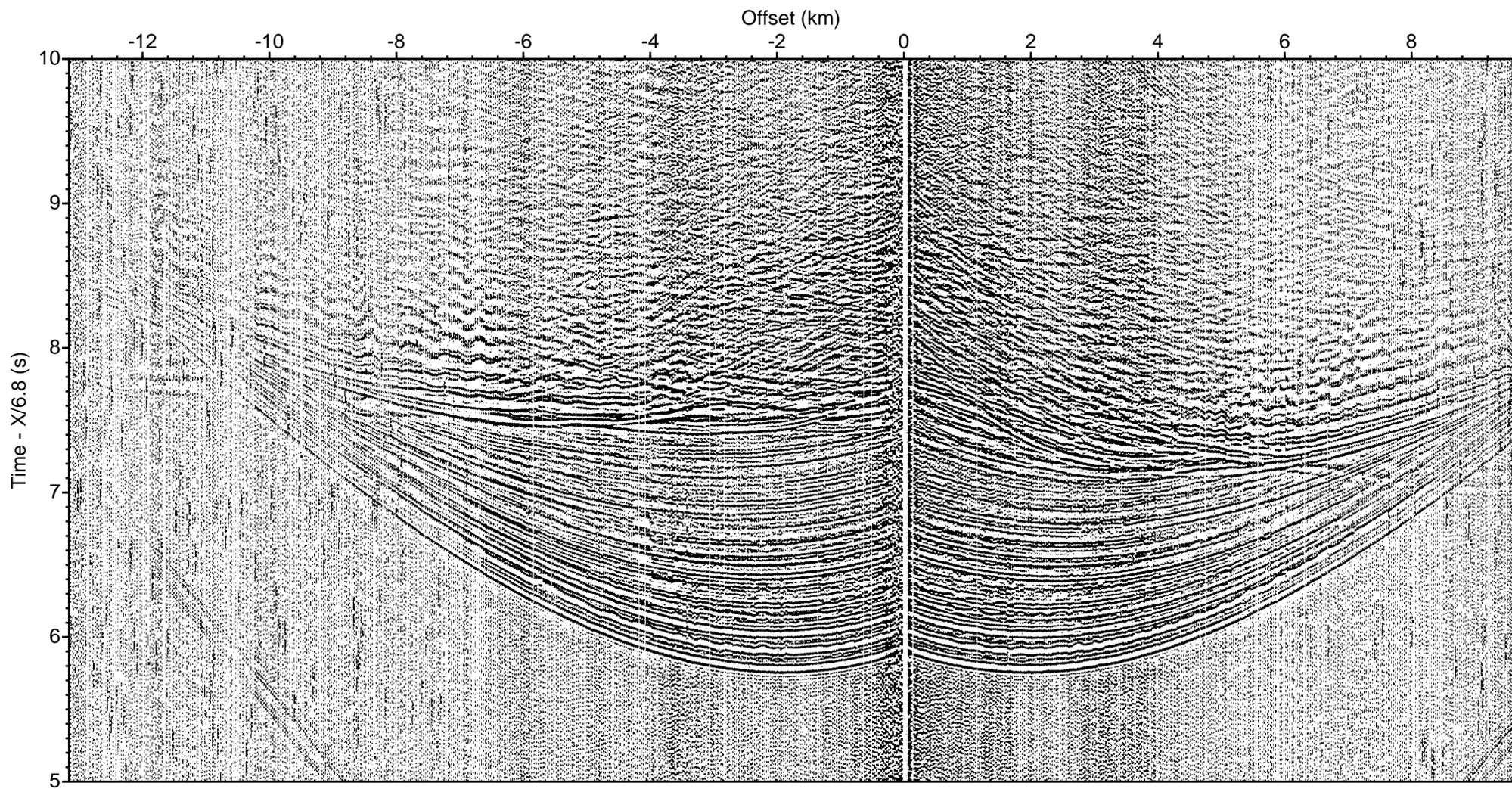
LOMROG III (2012) - Line 13 Sonobuoy 13-46 aux ch 2 (drift correction, deconv., bpf 5-40 Hz)
