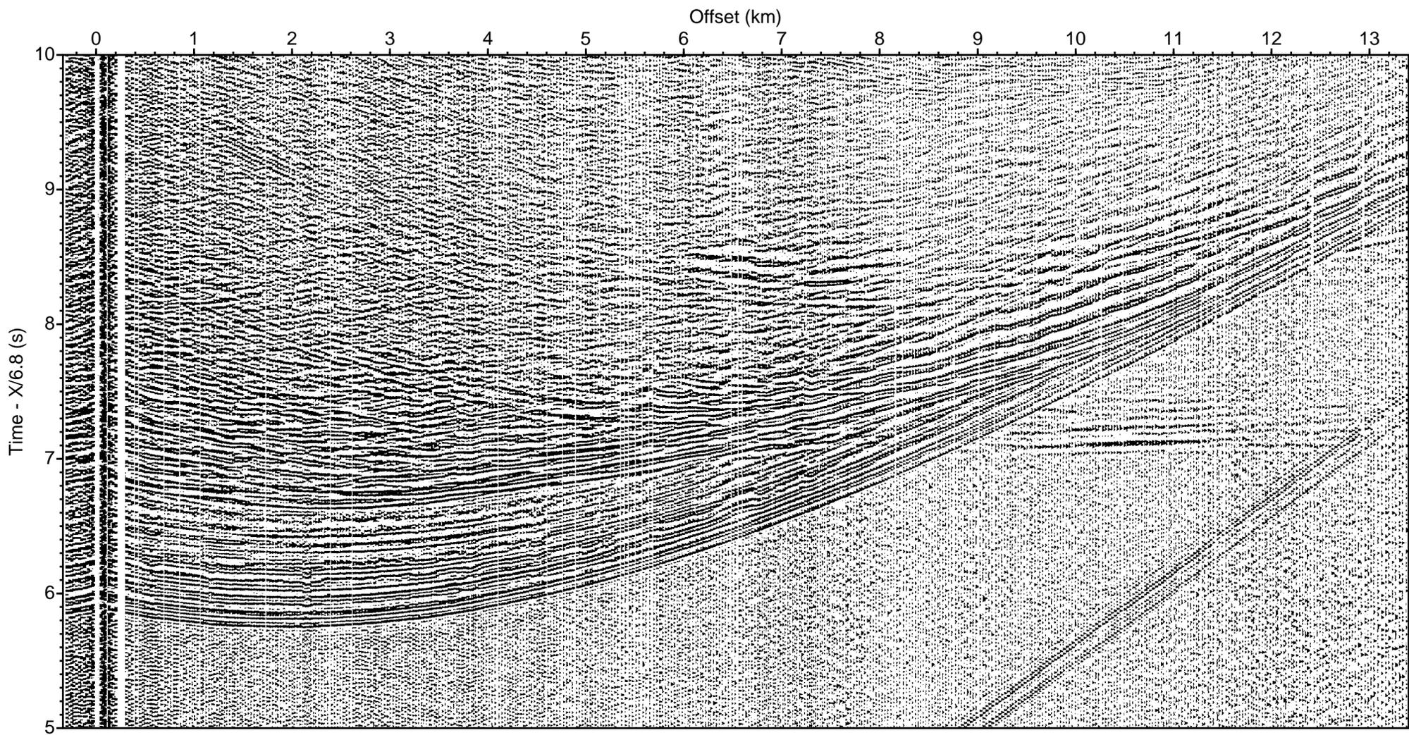
LOMROG III (2012) - Line 17 Sonobuoy 17-63 aux ch 3 (drift correction, deconv., bpf 5-40 Hz)
