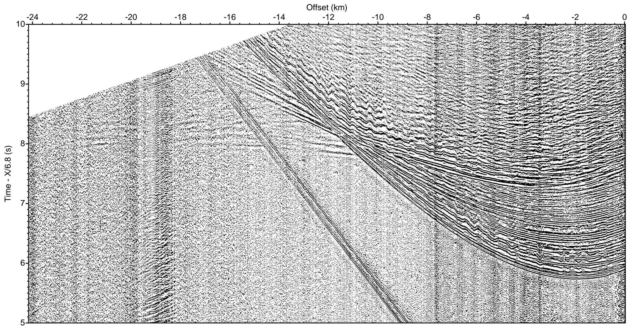
LOMROG III (2012) - Line 12 Sonobuoy 12-40 aux ch 1 (drift correction, deconv., bpf 5-40 Hz)
