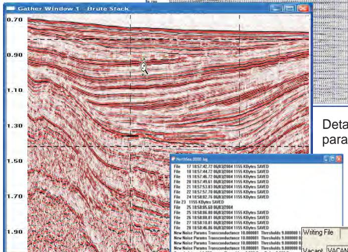
Detailed observer's log is kept with GPS location, parameter changes, exceeded thresholds and errors
