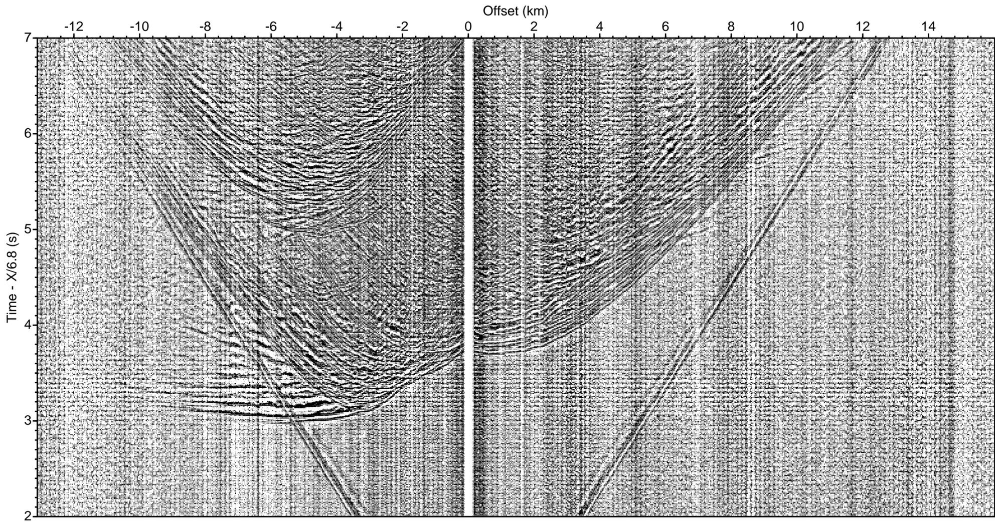
LOMROG III (2012) - Line 6 Sonobuoy 6-17 aux ch 3 (drift correction, deconv., bpf 5-40 Hz)
