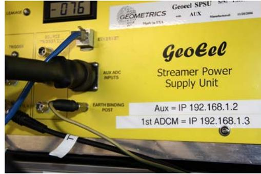
**Figure 28.** Connectors at the Taurus seismometer (left). The green-yellow cable at the far left connects to the ground plug (Earth Binding Post) of the GeoEel streamer power supply unit (right).
