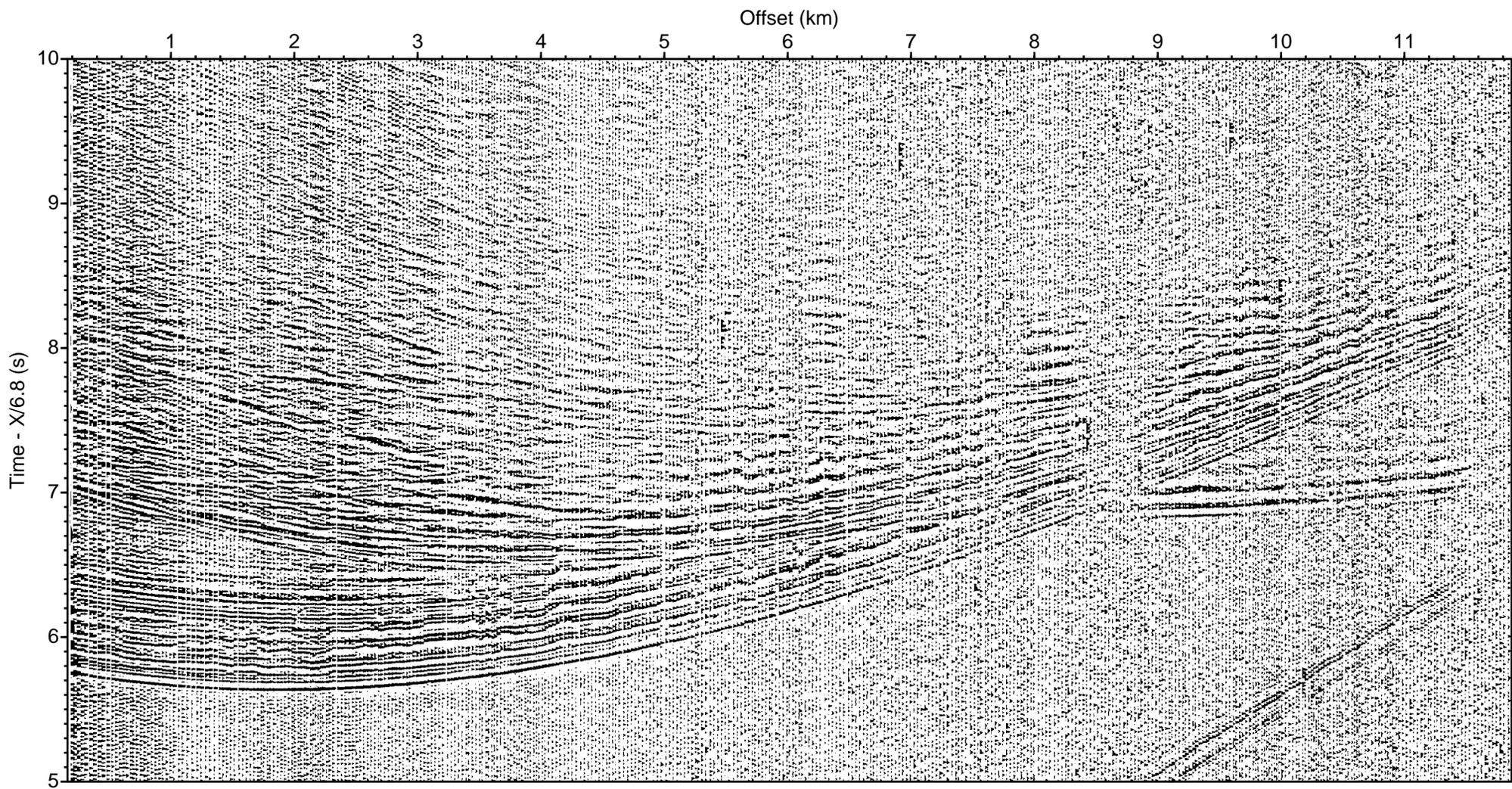
LOMROG III (2012) - Line 2 Sonobuoy 2-7 aux ch 3 (drift correction, deconv., bpf 5-40 Hz)
