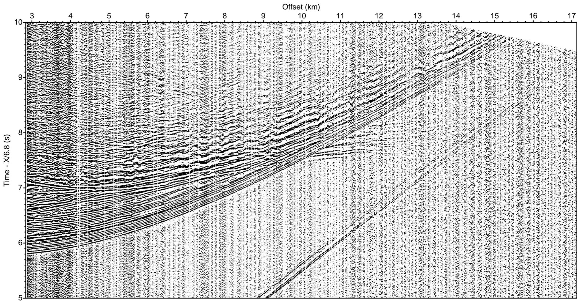
LOMROG III (2012) - Line 16 Sonobuoy 16-59 aux ch 3 (drift correction, deconv., bpf 5-40 Hz)
