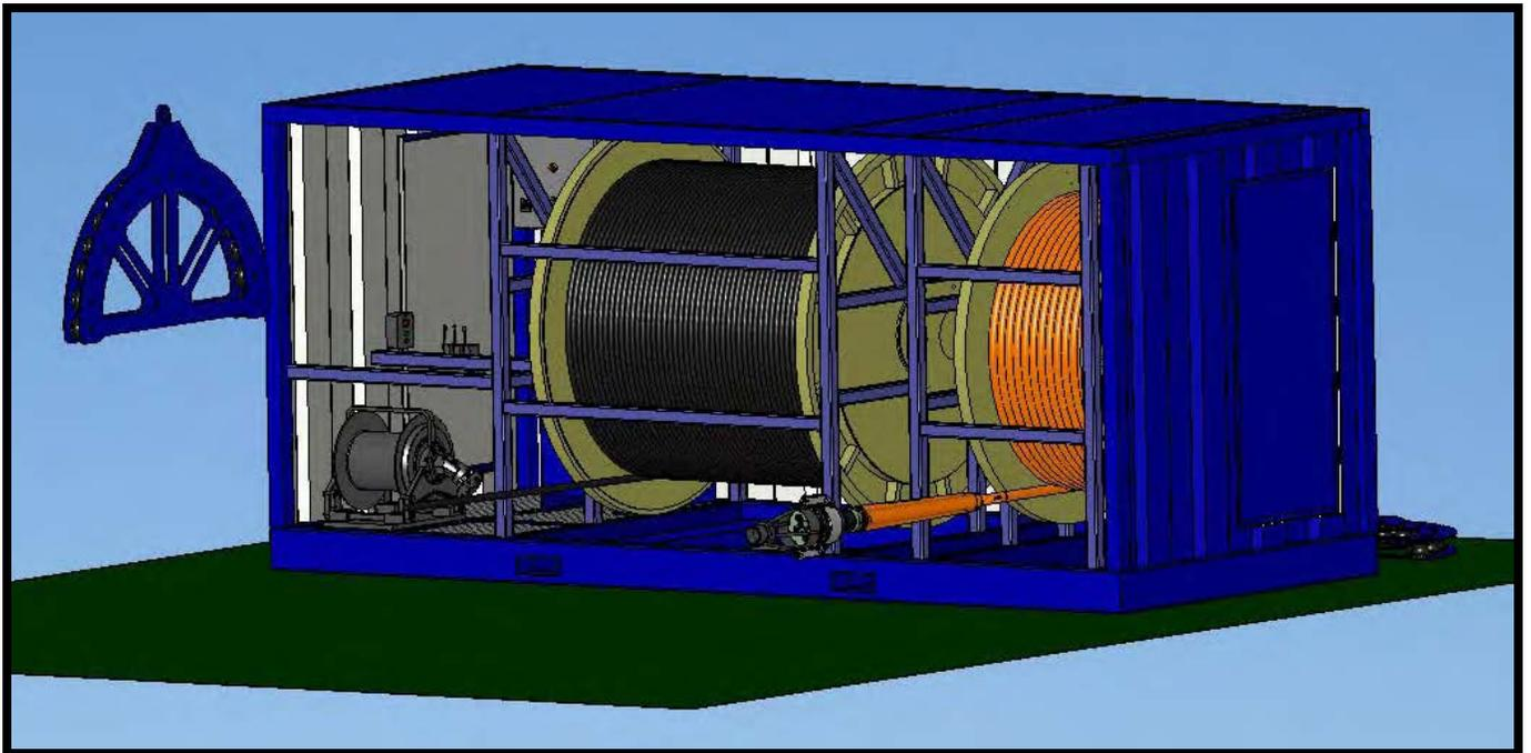
The Container is to be installed on the back deck of a vessel (e.g. Oden) and support the load of other equipment on top of the container. The winches are operated from the winch, via a sheave block mounted in connection with the vessel A-frame, over the stern of the vessel.
