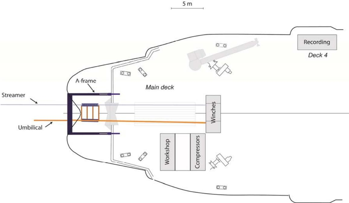
**Figure 8.** Plan view showing location of main equipment components on aft deck and deck 4.
