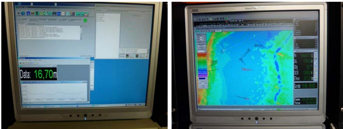
**Figure 7.** *NaviPac setup window (left) and NaviPac Helmsman's display for survey control (right).*
