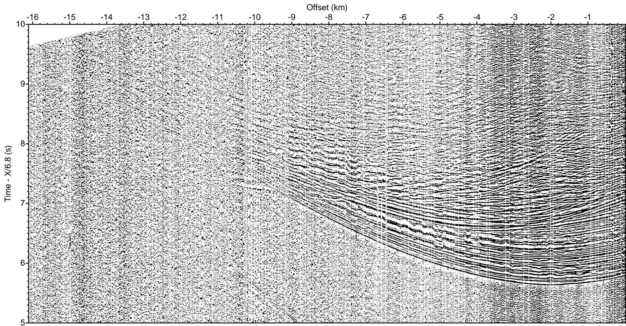
LOMROG III (2012) - Line 4 Sonobuoy 4-11 aux ch 1 (drift correction, deconv., bpf 5-40 Hz)
