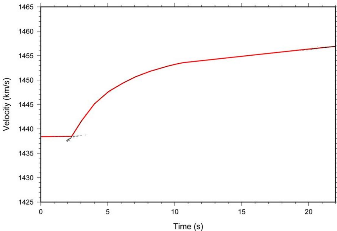
**Figure 35.** Average water velocity (offset divided by travel time) as a function of travel time of the direct wave obtained from one-dimensional ray tracing using the velocity function shown in Figure 34 (CTD S02). A complete set of all these curves relevant to the seismic data can be found in Appendix V-C.
