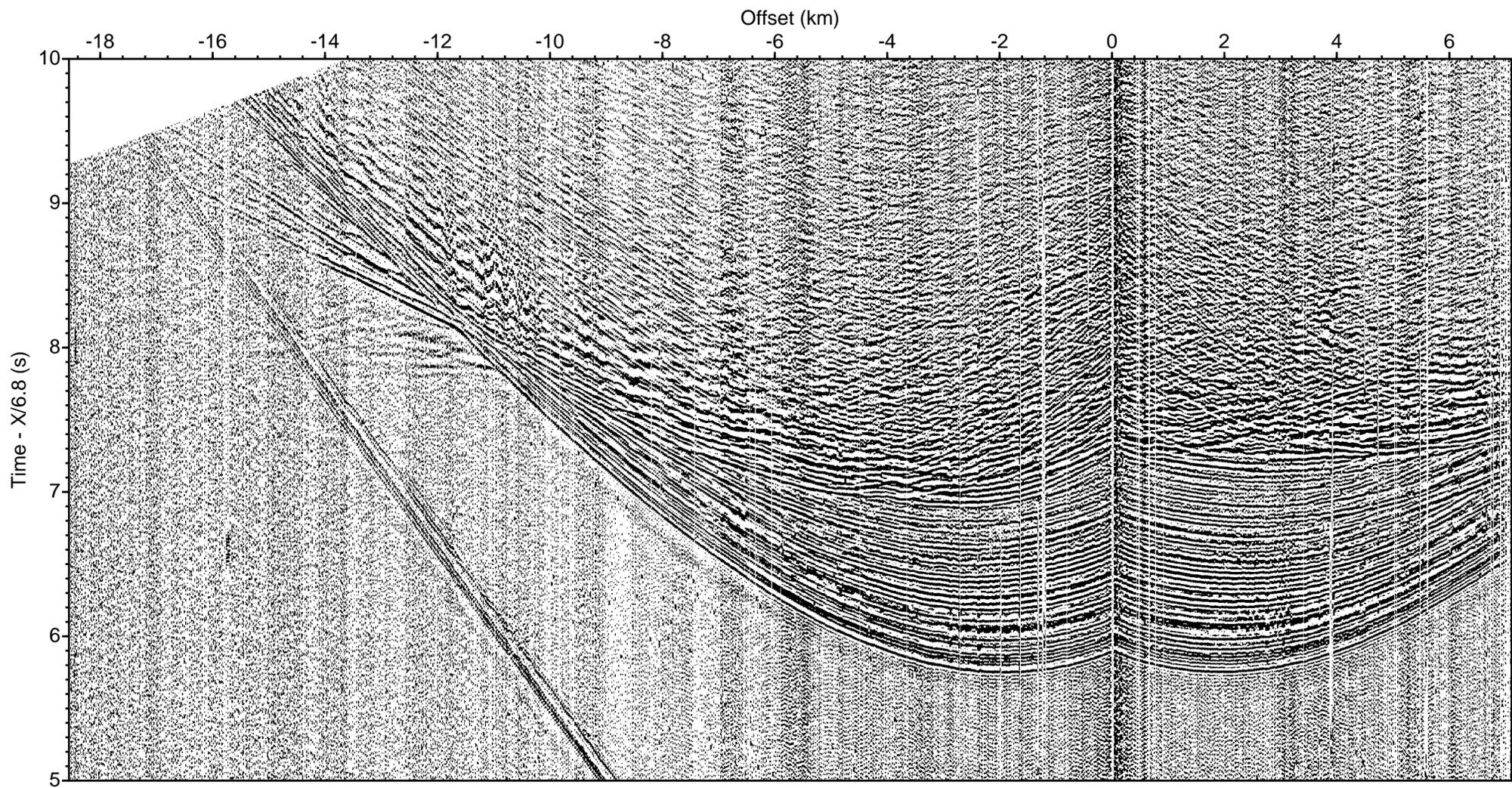
LOMROG III (2012) - Line 11 Sonobuoy 11-37 aux ch 4 (drift correction, deconv., bpf 5-40 Hz)
