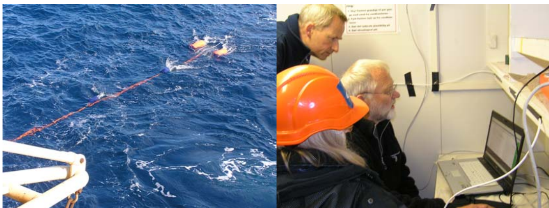
Figure 2 Left - the Sparker in the water; Right – the seismic control room
