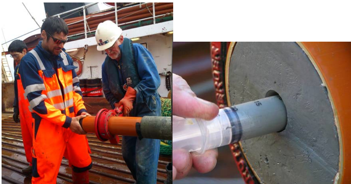
Figure 4 Left - Cutting the core into 1 m sections; Right - sediment sampling at the end of the section immediately after the cutting
