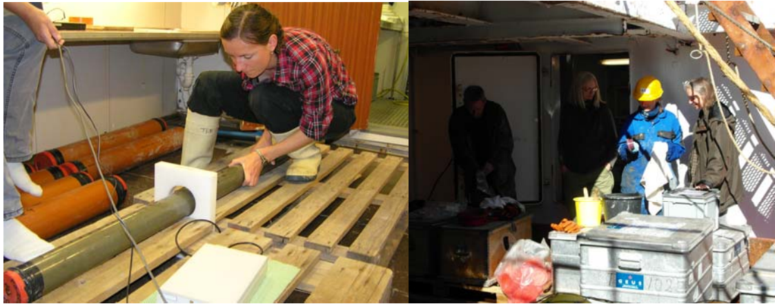
Figure 5 Left - Onboard measurement of magnetic susceptibility on Rumohrlot cores Right – Sub-sampling for foraminiferal analysis
