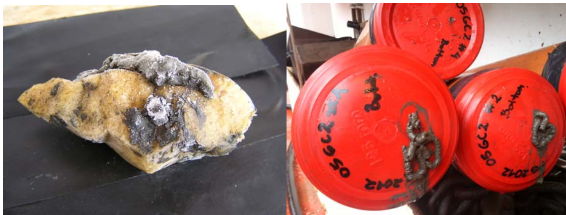
Figure 8 A ca. 6 cm long lkaite crystal was found in the core catcher of gravity core PG2012-05GC2, and sediments and gas was seeping out of the holes in the end caps of core sections 1 and 2
