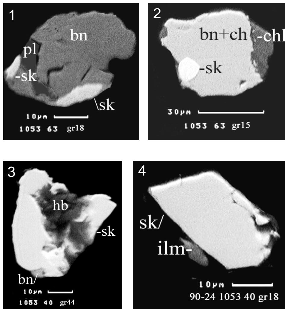
PGM grains attached to gangue or to gangue and sulphides
