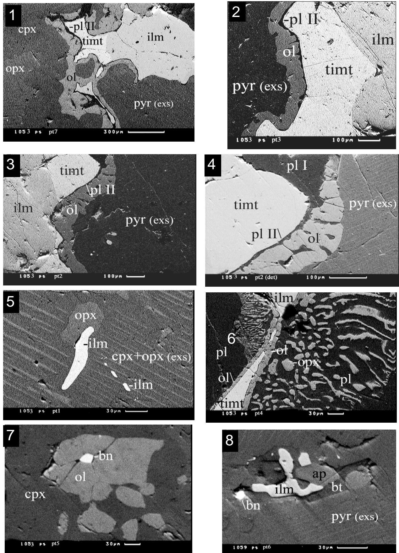
Relationships of rock-forming minerals, Fe-Ti oxides and sulphides in sample 90-24 1053; polished section, SEM-image (BIE).
