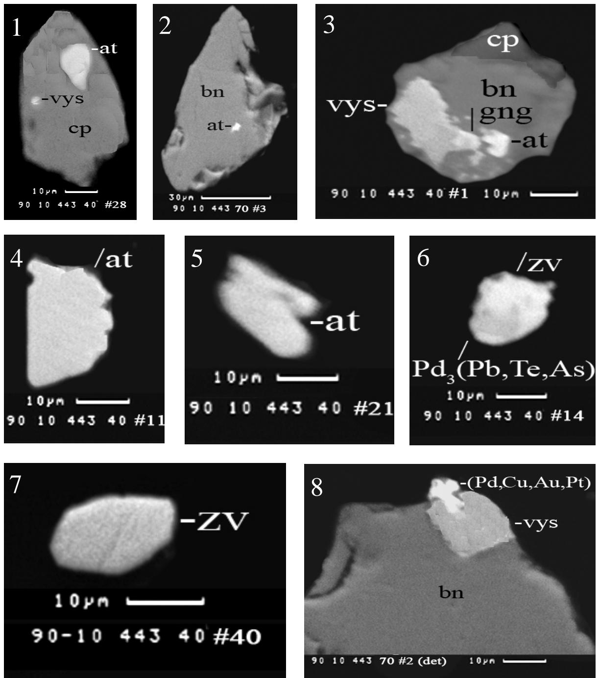
Grains of atokite (at), zvyagintsevite (zv) and (Pd,Cu,Au,Pt) alloy in the heavy mineral HS-concentrates of sample 90-10 443; polished sections; SEM-images (BIE).
