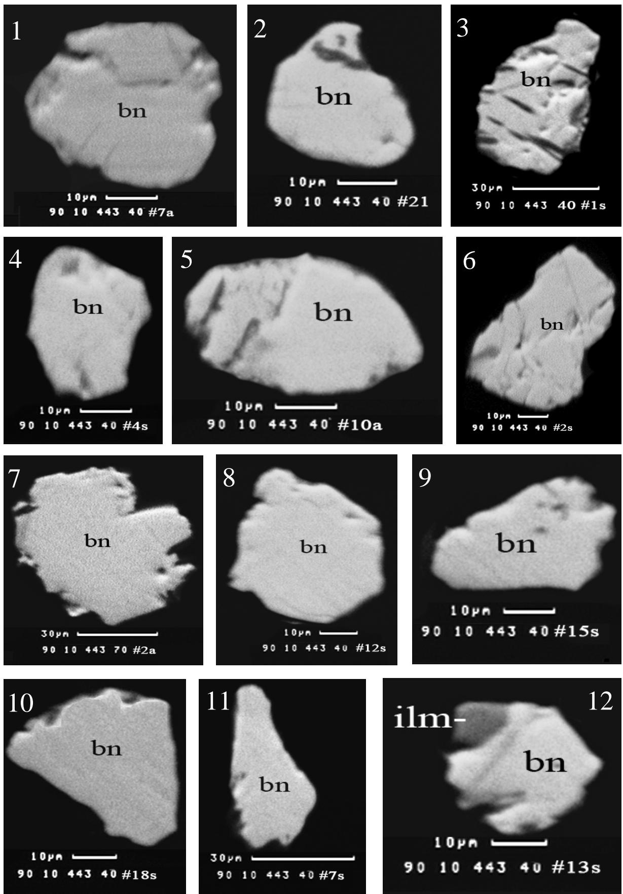
Grains of bornite (bn) in the heavy concentrates of sample 90-10 443 (1-12); polished sections; SEM-images (BIE). Abbreviations: bn: bornite; ilm: ilmenite
