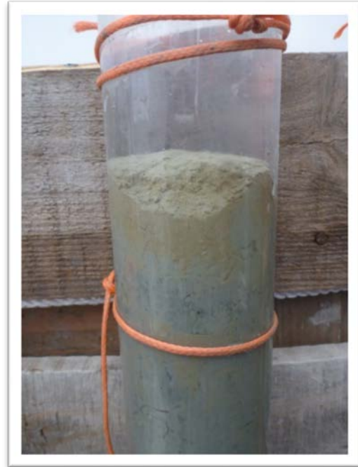
Fig. 3. Top of core liner showing an undisturbed sediment-water interface
