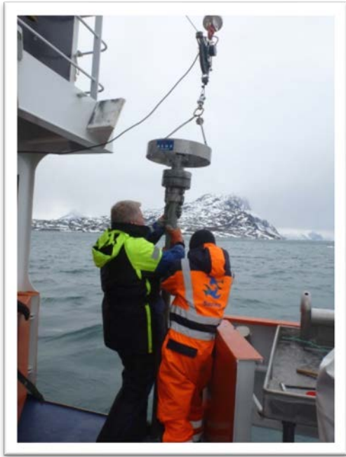
Fig 2: The Rumohr corer is deployed from R.V. Sanna
