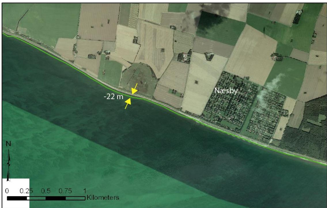
**Fig 18.** *The coast line at Næsby. In front of the summer cottage village Næsby coastal defence structures and beach nourishment protects the coast line from erosion (Green line: Digitized coast line from 1942).*
