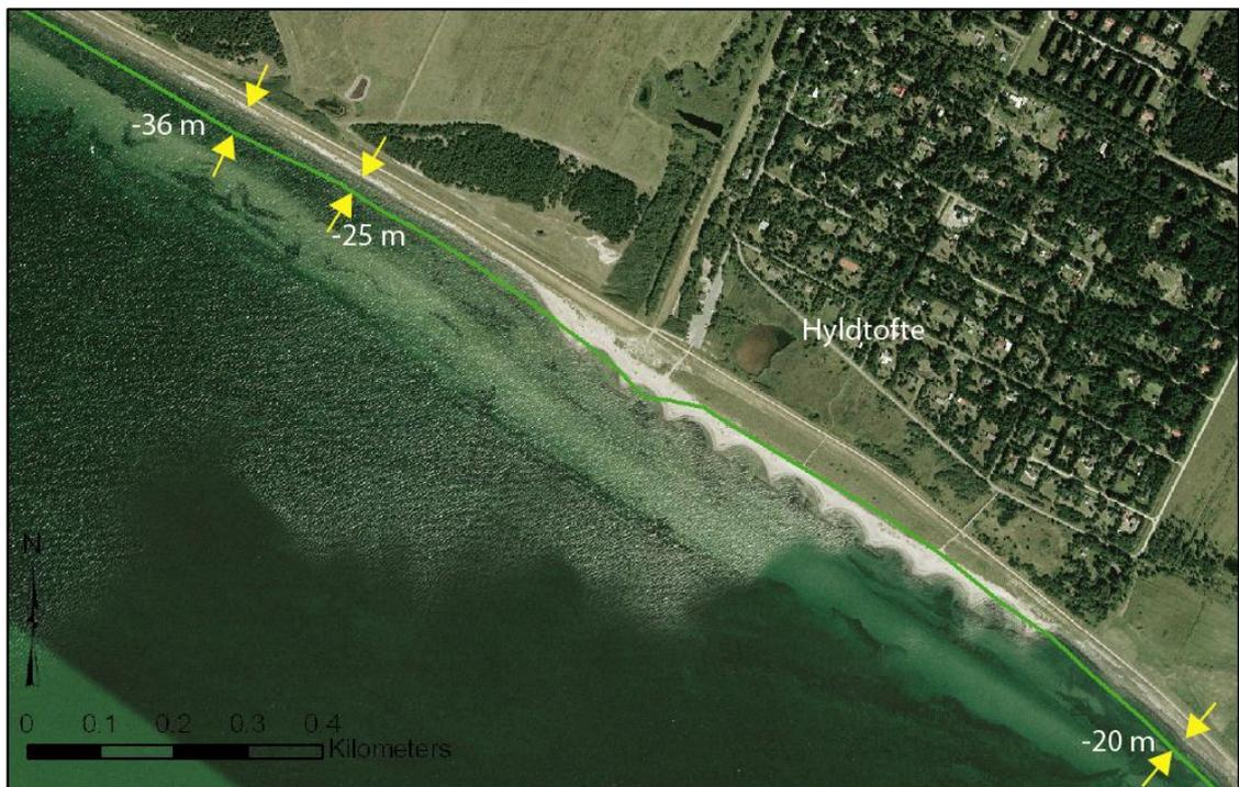
**Fig. 20.** At the coast line at Hyldtofte there is also coastal defence structures and beach nourishment is carried out to protect the coast line from erosion in front of the summer cottage village.
