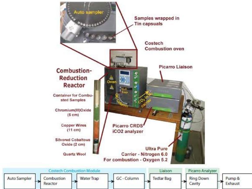
**Figure 2.** Top: Picture of the setup. Insets show closeup of the combustion/oxidation reactor and autosampler. Bottom: Flow chart showing the processing of the sample (after Balslev-Clausen, 2011)
