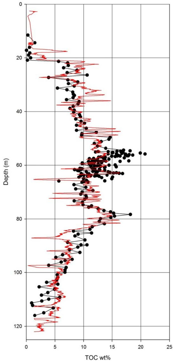
**Figure 19.** Comparison between measured TOC profile in the Fågeltofta-2 well and TOC calculated from the GR curve (red line). The majority of the gamma ray energy is associated with uranium and the difference between measured and calculated TOC content can be interpreted as a quick estimate of the U/TOC ratio.
