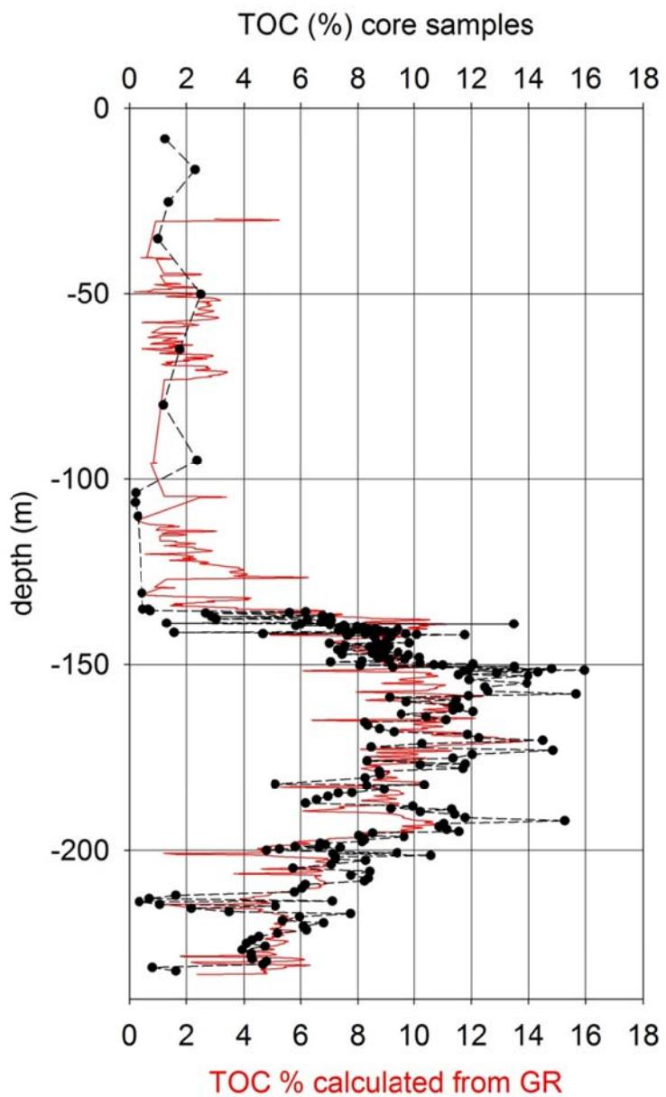
**Figure 20.** Comparison between measured TOC profile in the Albjära-1 well and TOC calculated from the GR curve (red line). The majority of the gamma ray energy is associated with uranium and the difference between measured and calculated TOC content can be interpreted as a quick estimate of the U/TOC ratio.
