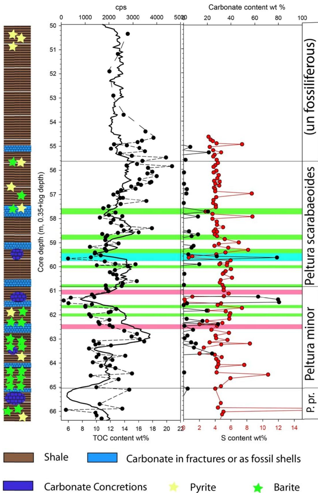
**Figure 17.** Same figure as Figure 16. Colour bars indicate the presence of more oxygen demanding faunal types in the core (after Christensen 2003). Colours, green: brachiopod; red: *Parabolina* type trilobites and light blue: agnostid trilobites.
