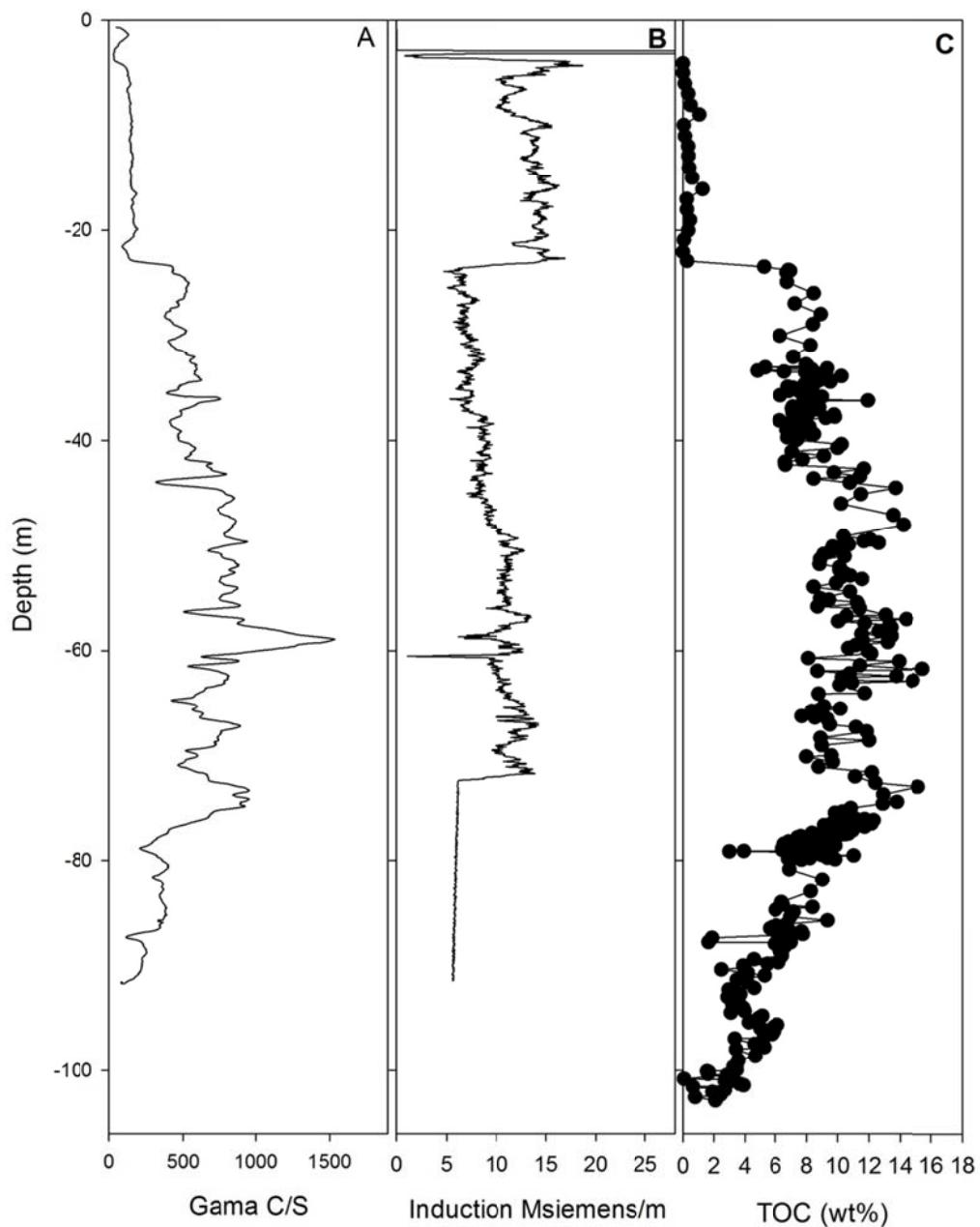
**Figure 9.** (A) Gamma ray log, (B) induction log and (C) TOC analysis in the Gislövshammar-2 well. The well was logged when it was drilled to 92 m. No logs were obtained for the deepest part of the well. The induction log ceased to function below 72 m.
