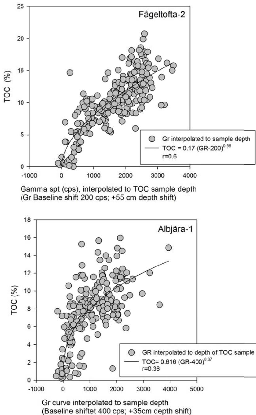
**Figure 18.** Relationship between TOC and gammay ray for (top) the Fågeltofta-2 well and (base) the Albjära-1 well. The relationship between gamma ray and TOC is controlled by the enrichment of uranium and is modelled using a power function.
