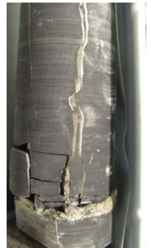
Two generations of fracture formation. First generation was cemented with calcite. Subsequently fractures were formed and clay was injected from clay layer into the fracture.
