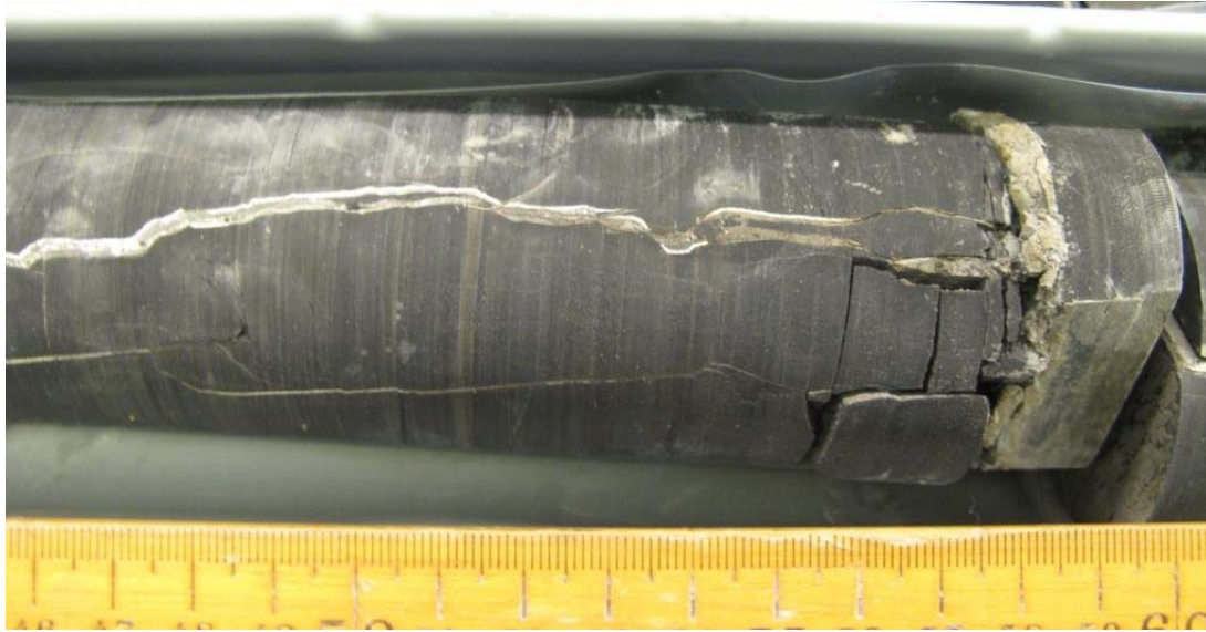
Figure 5. Clay injected into a fracture from a bentonite rich layer in the shale at 49.6 m.
