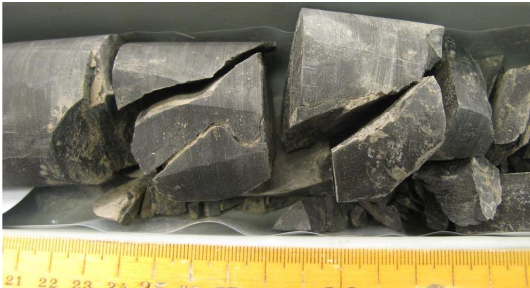
Figure 15. Irregular fractures at 51.3 m from which the largest inflow of water (33% of the total inflow) occur.
