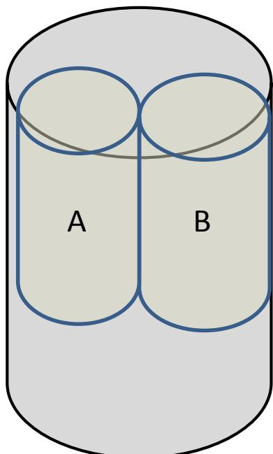
*Figure 1 Sketch of coring orientation and placement of specimens for unconfined compression tests in the plug samples.*
