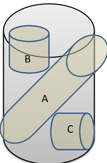
*Figure 2 Sketch of coring orientation for specimens prepared for acoustic measurements (A: 45°, B: vertical, C: horizontal).*
