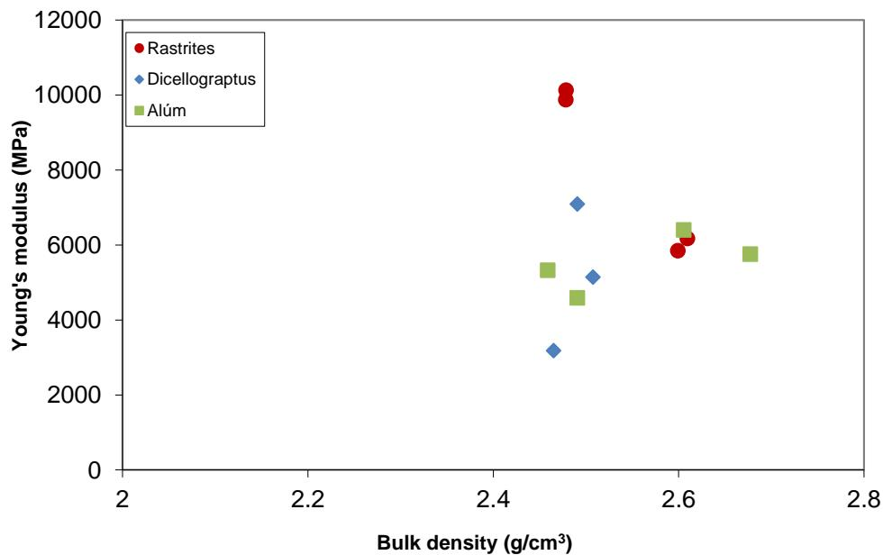
Figure 4 Results of Young's Modulus of elasticity from unconfined compression tests.
