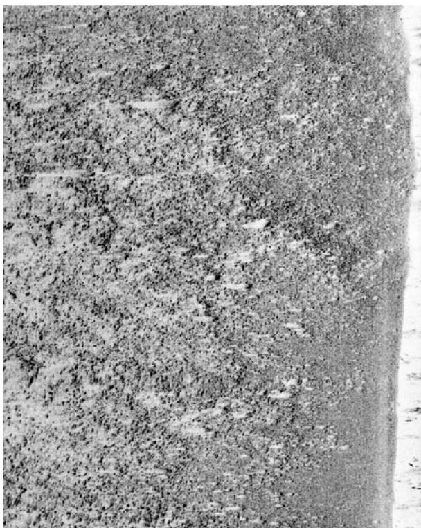
Station s12. Sidescan picture showing a seabed with a dense cover of boulders with average heights of less than 1.0 m. A few scattered large stones of 2-3 m height have been registered. The blurred outline of the boulders most likely is due to vegetation.
