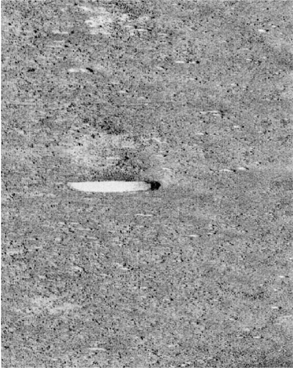
Station s7. Single, very large object lying on a gravelly to stony seabed. The height of the stone is measured to 3 – 4 m in height. The blurred outline of the surrounding seabed is most likely due to vegetation. Approximate dimension of the sections: Height 150 m and width 50 m.
