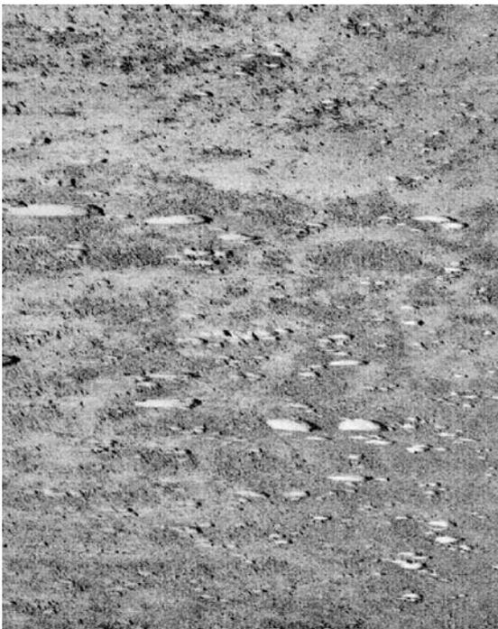
Sidescan picture of paravane 6. The picture shows the paravane start position with a transition from a sandy seabed type at the top via a sharp boundary to a gravelly seabed with a
