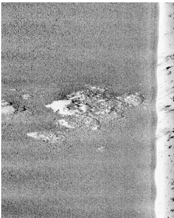
Station s14: Sidescan picture showing the structure of high reflectivity anticipated as a 'bubbling reef' surrounded by a level sandy seabed. The transition is sharp. Some topography within the feature is recognised by the shadows indicating a rough surface. These features are found scattered within an area of 600 m x 200 m.
