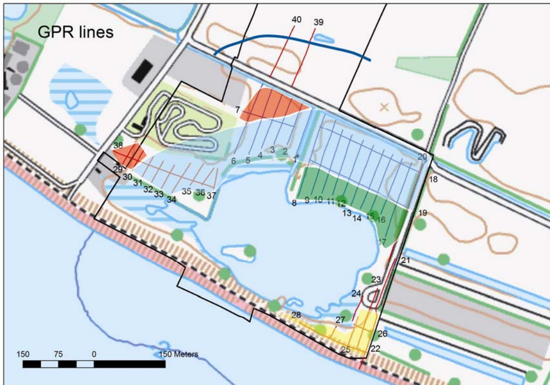
Figure 15. Conclusions from the interpretation of the GPR survey. The red shade shows the outline of the declining till surfaces. They are probably connected underneath the go-kart track. There are probably several older shorelines on this declining surface, belonging to different stages of the rising sea level since about 6500 to 7000 years ago. The green shade shows the outline of the sand unit with wash over fan structures, representing an old surface at about level -1m. The yellow shade shows the outline of dunes and cover sand on top of a barrier island or spit. The blue shade shows the outline of the lagoon basin. The blue line shows the youngest and highest shore line.
