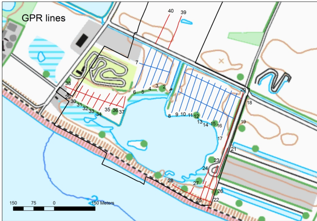
Figure 2. The investigation area where the blue and red lines are the measured GPR lines. The black line is the tunnel ramp area.
