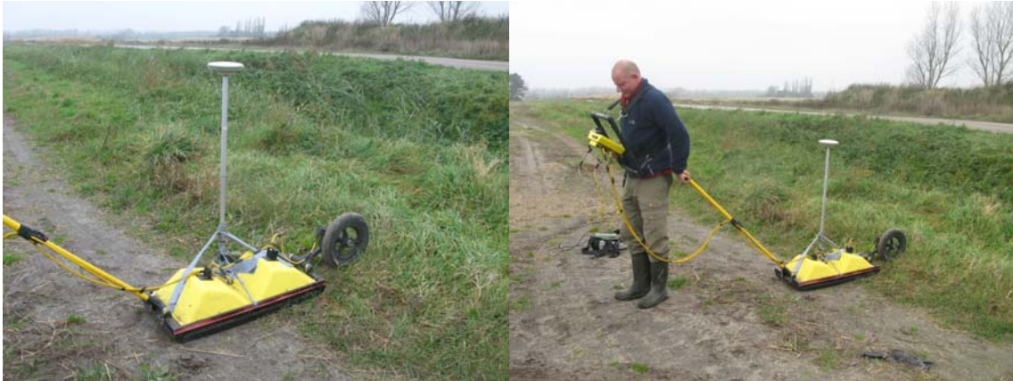
Figure 4: The left picture show the GPR acquisition system. The two yellow boxes are the transmitter and receiver transducers and the wheel behind is the odometer that measures the distance. The DGPS is placed between the GPR antennas. The right picture shows how it works. The GPR is pulled slowly and the operator can look at the data displayed on a screen during the data acquisition. The operator is also carrying the battery for the GPR system. The GPS measurement is managed of another person who is carrying a backpack with the antenna, cell phone and the computer all connected to the receiver.
