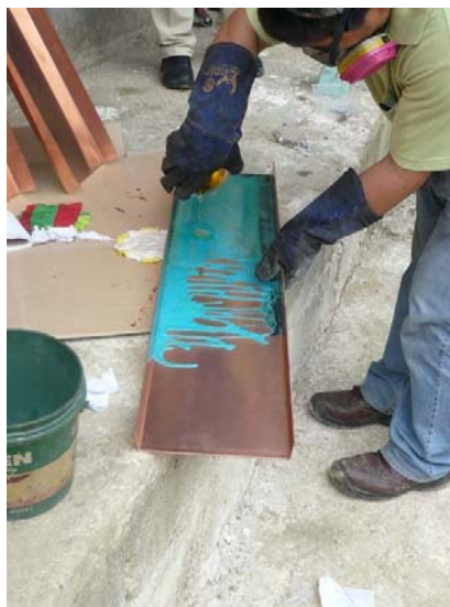
Figure 6. Mercury nitrate is added to the copper plate forming copper amalgam and blue green copper nitrate
