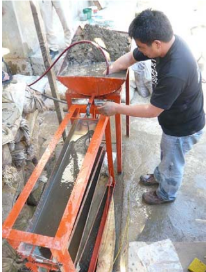
Figure 5. Peter Plates. Tailings being flushed down the plates and mercury is captured by copper amalgam on the plates. Scale 1 cm
