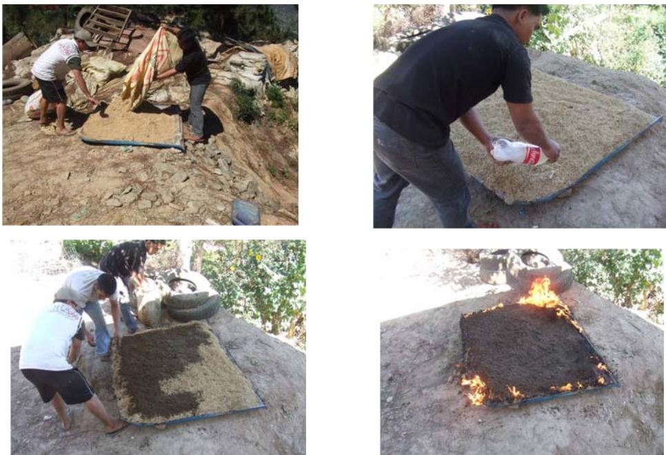
Figure 4. Rice hull spread over a metal plate. Kerosene is added. Tailings are spread over the rice hull and the kerosene is ignited. The mercury evaporates and gold can be recovered.
