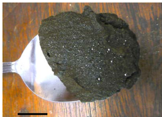
Figure 1. Mercury flour in tailings. The shiny mercury drops are less than a millimetre across. Scale 1 cm.
