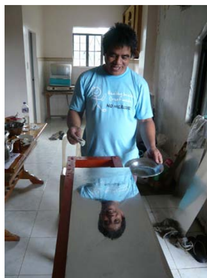
Figure 8. Perfect coating of a copper plate with activated mercury
