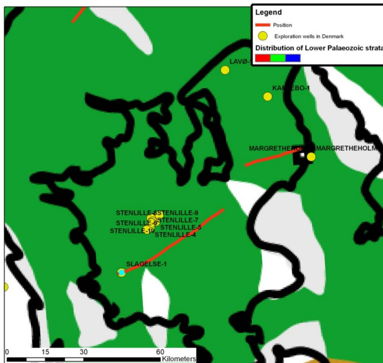
Figure 20. Location of the deep reflection line 72/001 in SW part of Zealand. The line is 49.1 km long and was recorded in 1972. Well control is from the Slagelse-1 well (highlighted with light blue colour). Yellow circles are exploration wells and the distribution of the Lower Palaeozoic strata is shown with green (Nielsen & Schovsbo 2011). For a larger view of the map see Figure 1.
