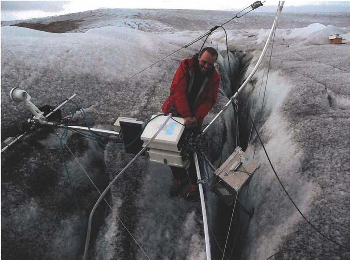
**Figure 25.** *Salvaging instruments from a station fallen into a crevasse on the Qassimiut lobe in South Greenland.*
