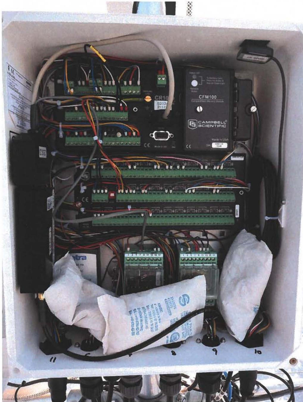
**Figure 2.** A look inside a data logger enclosure. Some instruments, such as the GPS and the barometer are actually inside the enclosure. The white bags contain dessicant to remove humidity inside the box, which could otherwise cause problems with the electronics.
