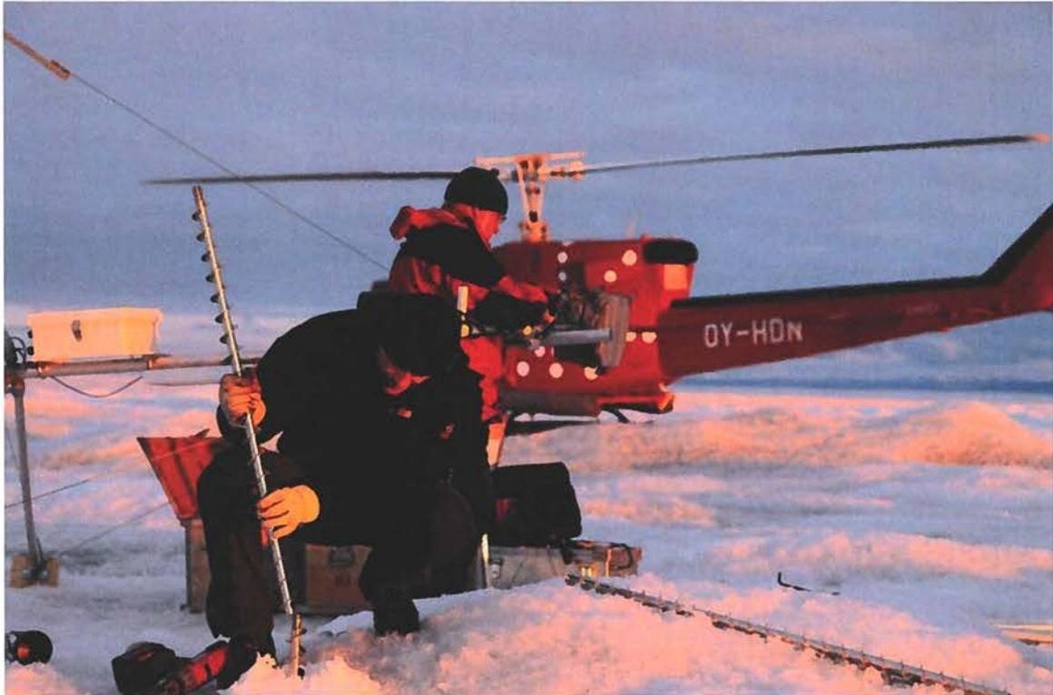
**Figure 23.** *Drilling with the Kovacs mechanical drill. Note the practical one metre auger pieces.*
