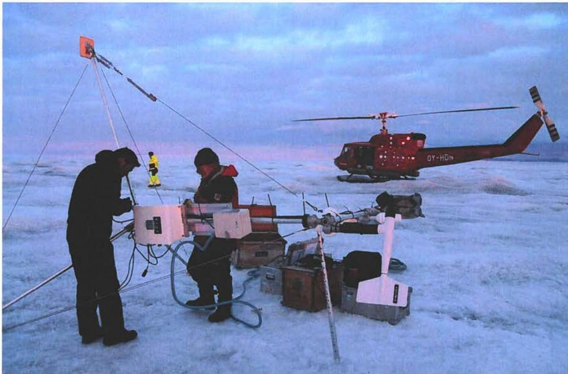
**Figure 22.** *Mounting of instruments and boom on a station tripod on the ice sheet. Note the practical, adjustable custom-made rest.*
