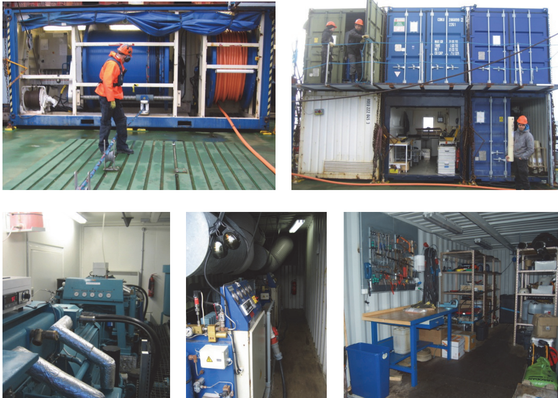
Figure 7. Containers on aft deck: winches (top left), compressors (white and green), storage (blue) and workshop containers (open) (top right), interior of compressor containers (bottom left) and interior of airgun workshop container (bottom right).
