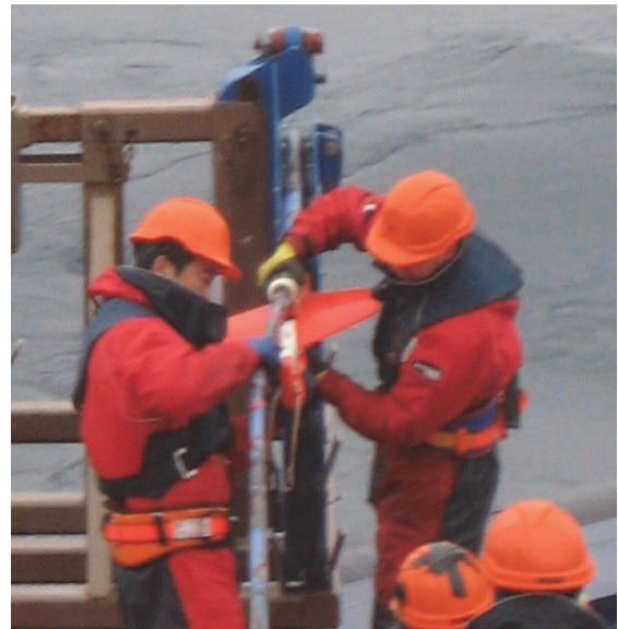
Figure 12. Roller ports for the streamer along the aft deck (left) and mounting of depth controller bird on streamer before deployment (right).
