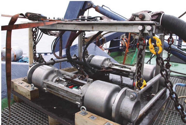
Figure 26. Large airgun array consisting of four 520 cubic inches Sercel G-guns. Photo: Thomas Funck
