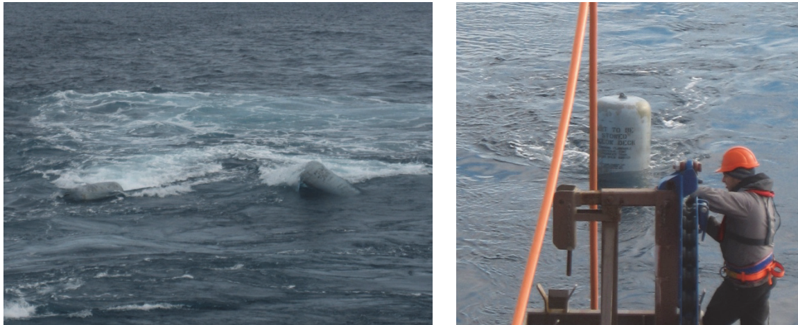
Figure 17. Towing airgun array in two US Fender buoys in ice free waters (left) and in one US Fender buoy in light ice conditions (right).
