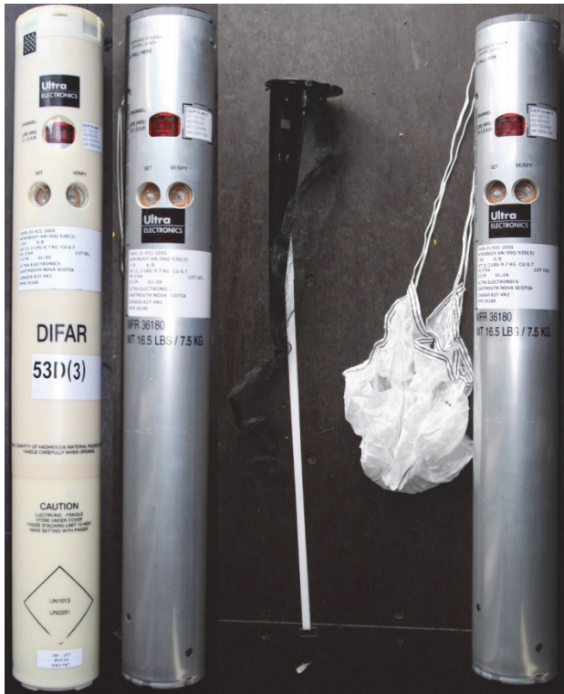
Figure 32. Sonobuoy type AN/SSQ-53D(3) from ULTRA Electronics. The left part of the image shows the sonobuoy in the hermetically sealed buoy launch container. In the centre, the buoy is shown after removal of the storage container. The right part of the picture provides a view on the sonobuoy with the top cap (lanyard) removed, where the parachute is stored. The buoy is deployed in this state. Photo: Thomas Funck.
