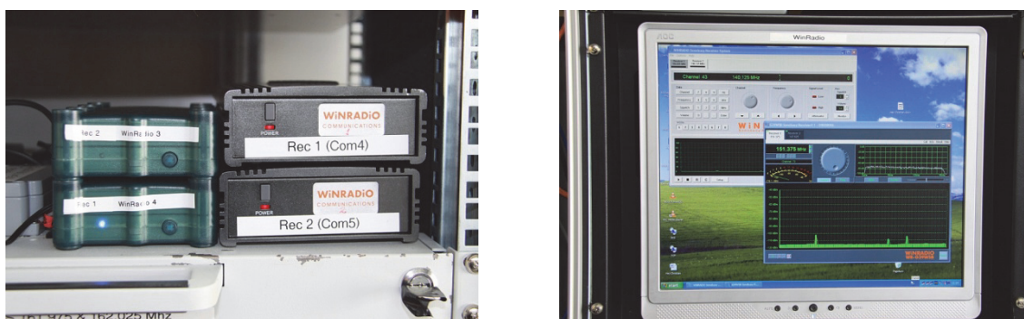
Figure 34. Sonobuoy receiving system. The two older Winradios (type WR-2902e; black boxes) are controlled by Winradio software (upper left window on computer display). The two newer Winradios (type WR-G39WSB; green boxes) were controlled by the Winradio software in the lower right window on the computer display. Photos: Thomas Funck.
