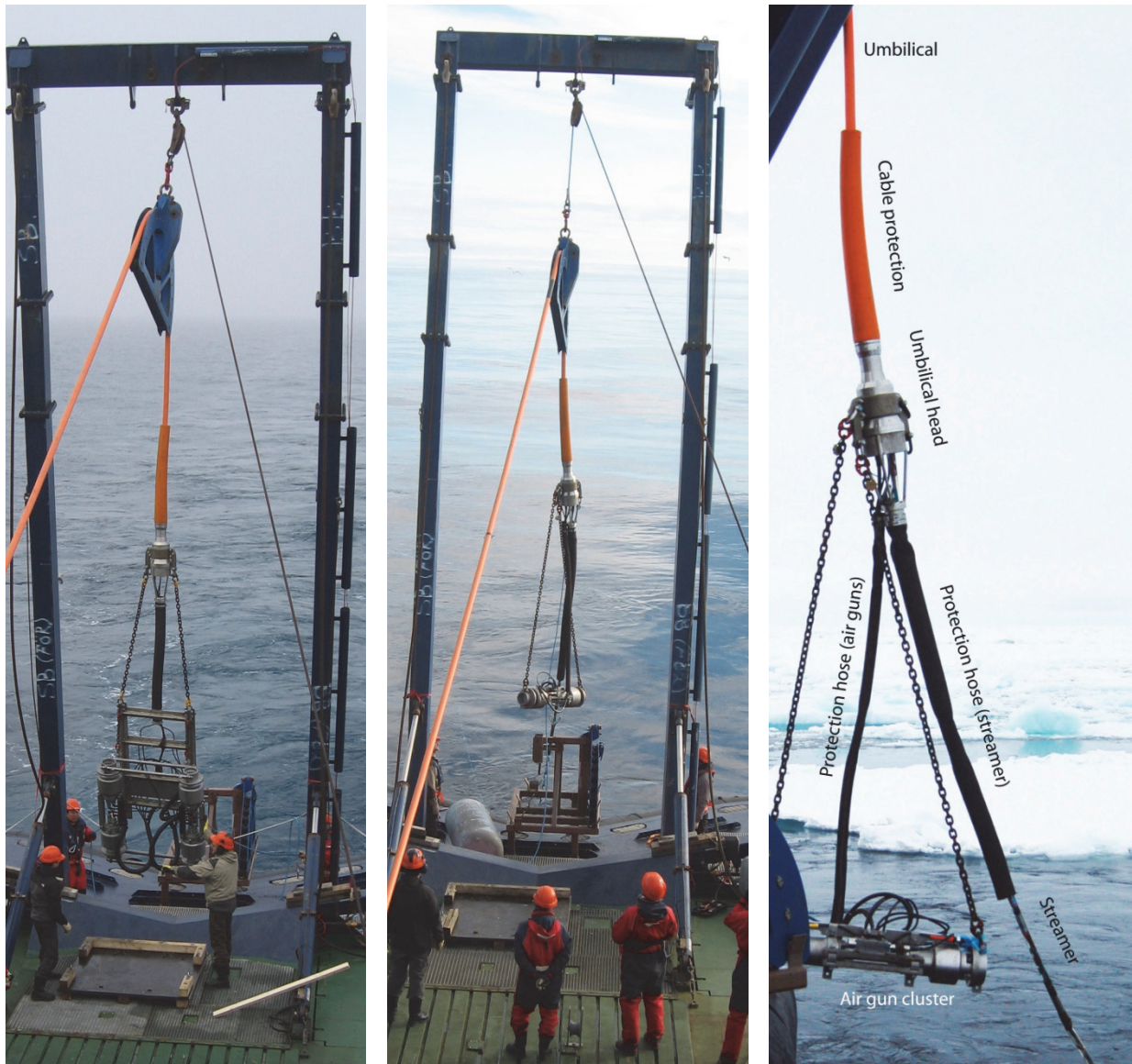
Figure 11. Deployment of array for ice free waters (left), for light ice conditions (middle) and close-up of the sea end of the umbilical in light ice conditions (right).
