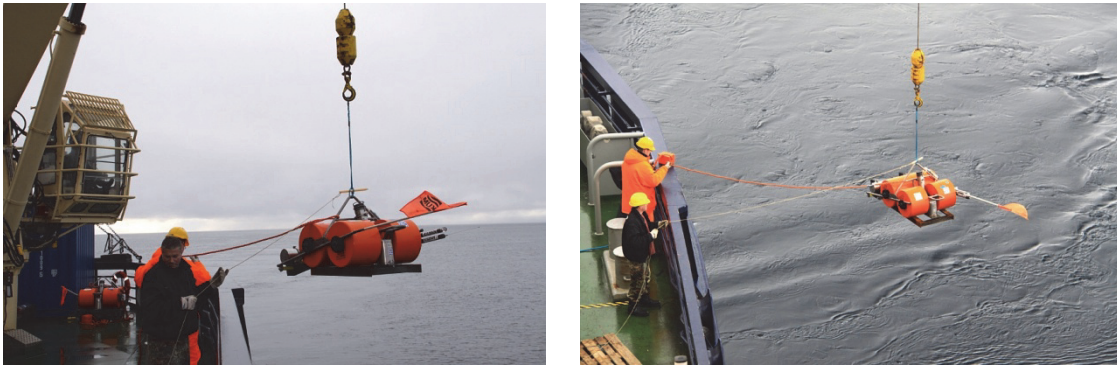
Figure 43. Deployment of the ocean bottom seismometers (OBS). Photos: Thomas Funck.
