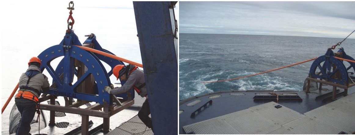
Figure 14. Umbilical sheave docking platform (left), guns and streamer in final position (right).
