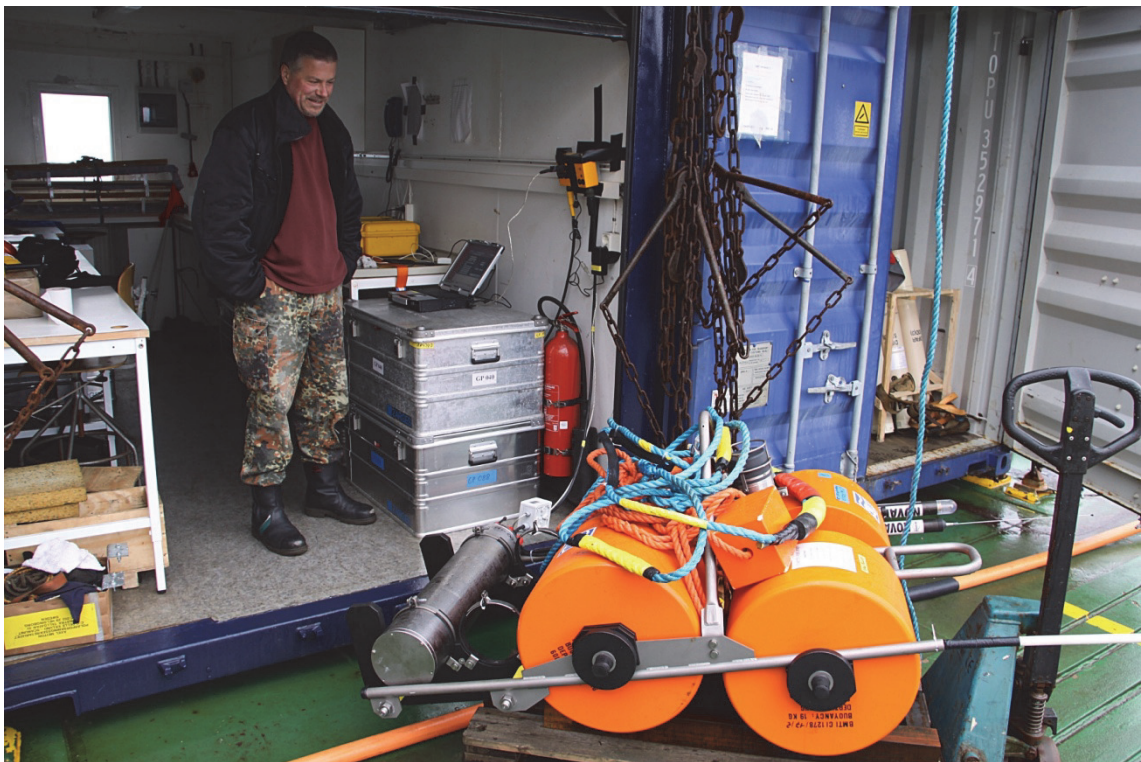
Figure 42. Connecting the LOBSTER via the yellow GPD30 box to an external GPS clock and a laptop computer to start or stop data acquisition. Photo: Thomas Funck.
