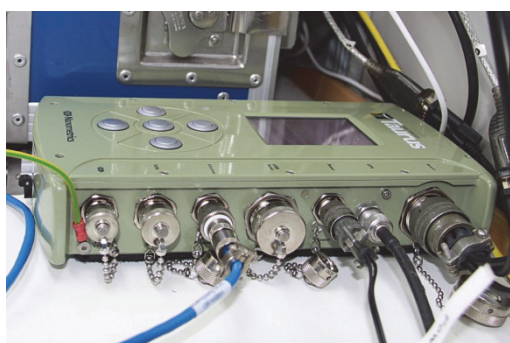
Figure 38. Connectors at the Taurus seismometer (left). The green-yellow cable at the far left connects to the ground plug (Earth Binding Post) of the GeoEel streamer power supply unit (right). Photos: Thomas Funck.
