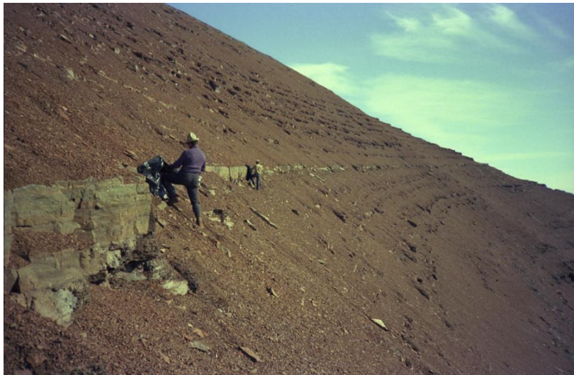
Figure 33. Chip sampling at Nordenskiöld Bjerg of sandstone beds with Redbed Copper type mineralizations. Photo from presentation made by B. Thomassen at the workshop.
