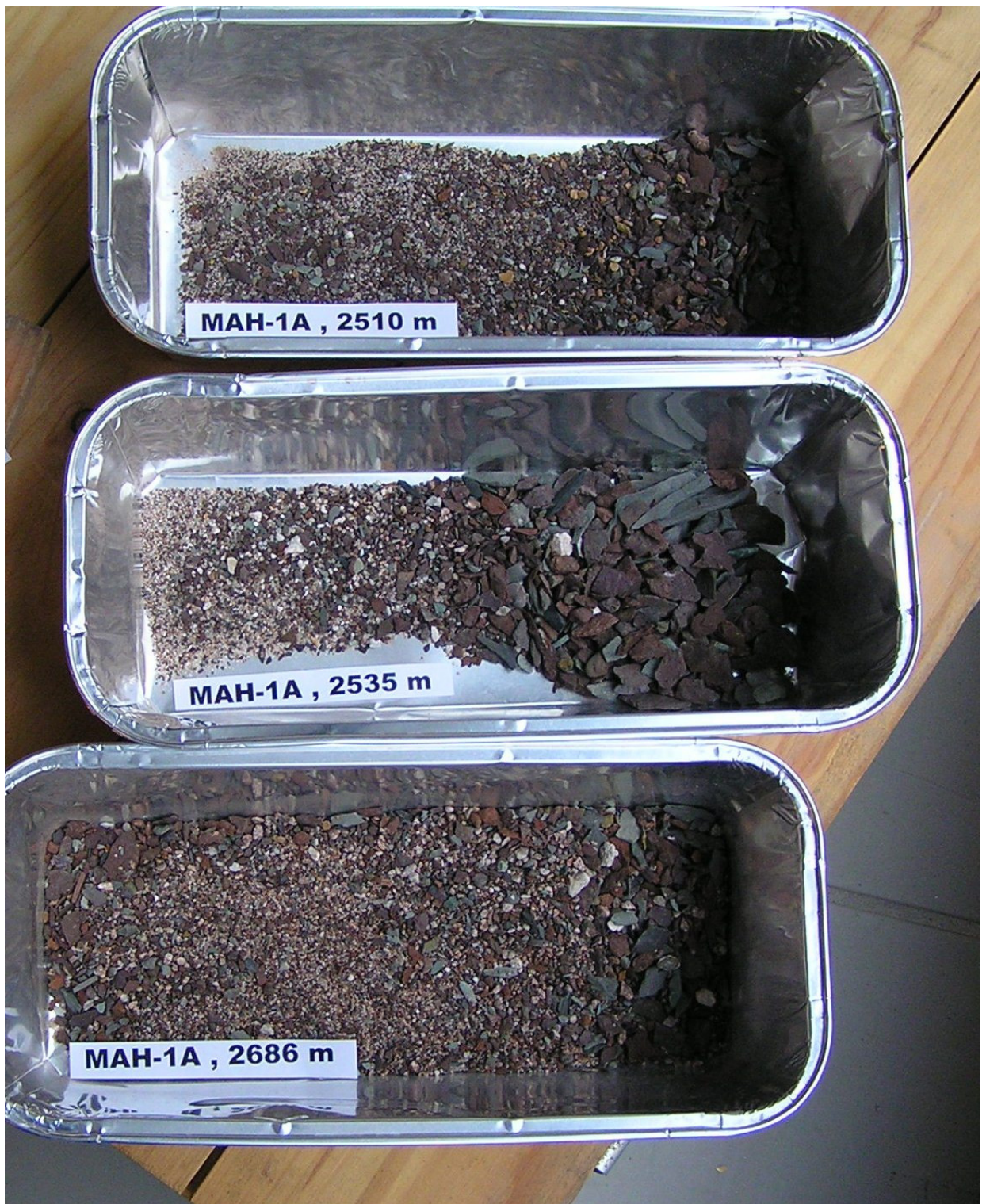
Figure 2. Three samples of washed and dried cuttings selected for acid experiments
