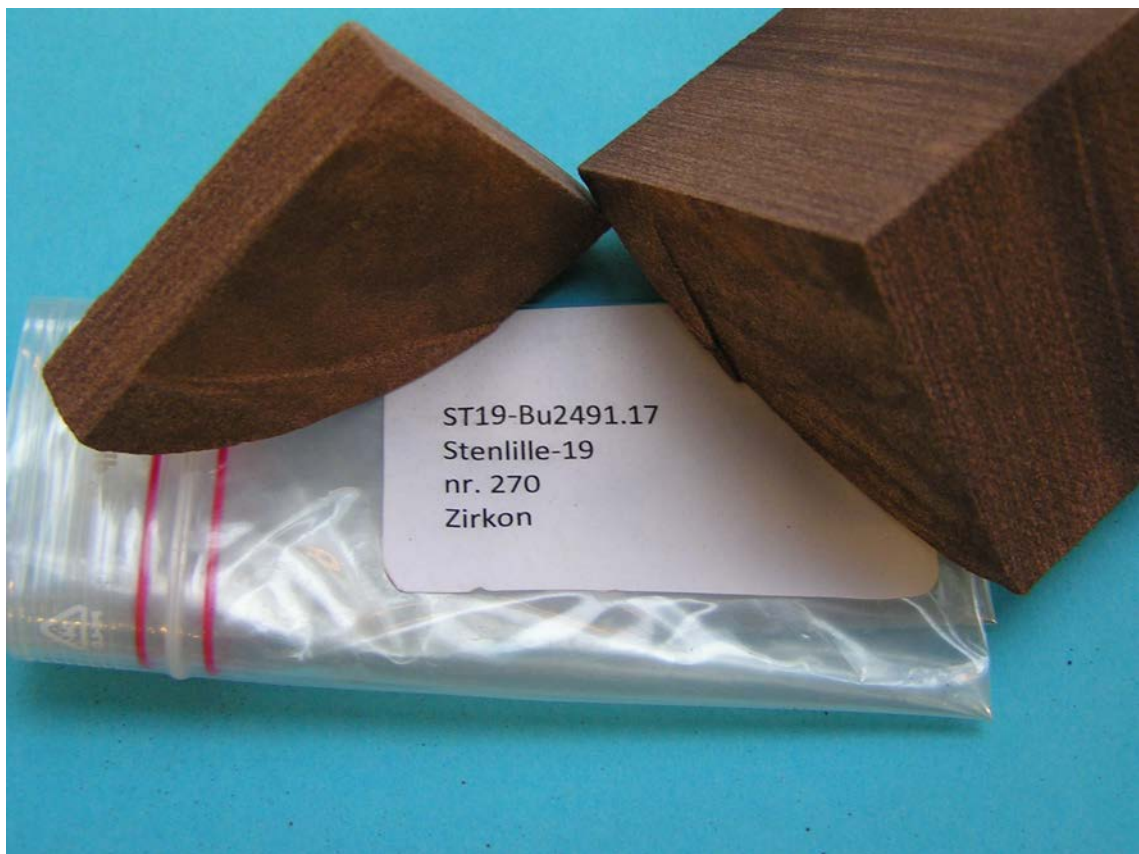
Figure 3. Subsample of St19 core selected for acid experiment.
