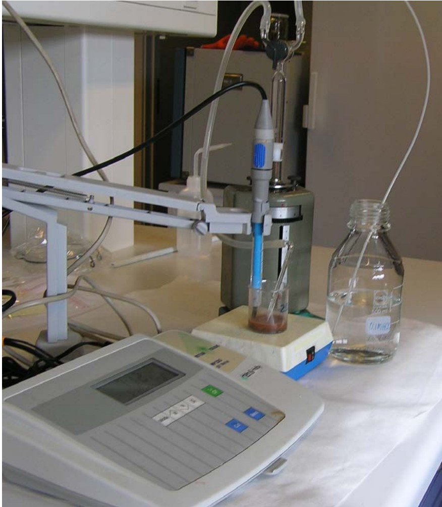
Figure 4. Laboratory set-up for acid titration experiment
