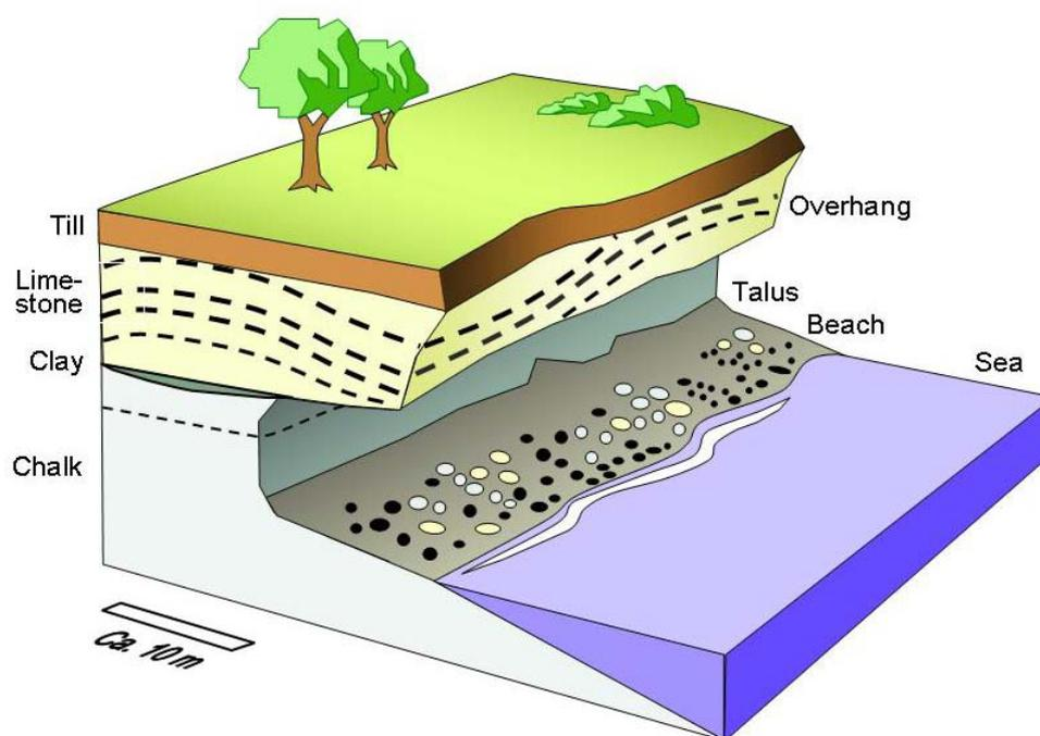
**Figure 2.** The block diagram illustrates the main geology and geomorphology of the coastal cliff at Stevns Klint. At the base of the geological succession the white chalk is soft and subjected to erosion. The hard Danian limestone forms the overhang above the Cretaceous/Tertiary boundary (C/T) at the base of the clay. Details about the lithostratigraphy are given in Fig. 3.
