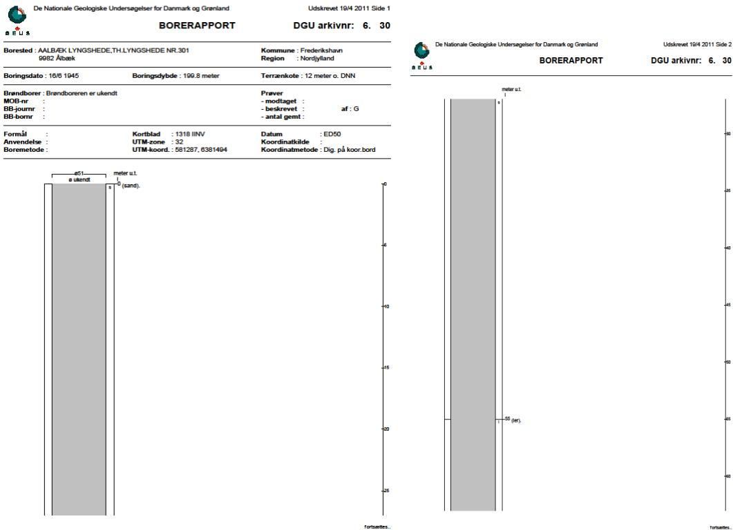
Figure 5. Example of borehole log from DGU no. 6.30. The upper approx. 135 m of the 199.8 m deep borehole. The log covers three pages. Legend: yg: Late Glacial marine deposits, dl: meltwater clay and silt, ds: meltwater sand and gravel, ql: marine interglacial clay, qs: Interglacial sand deposits, s: sand, l: clay, v: small layers.
