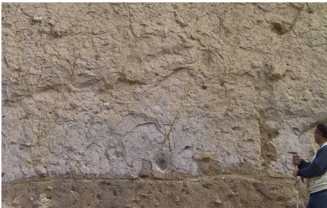
Figure 14. Example of fractures in clayey till (Photo: K.E.S. Klint).
