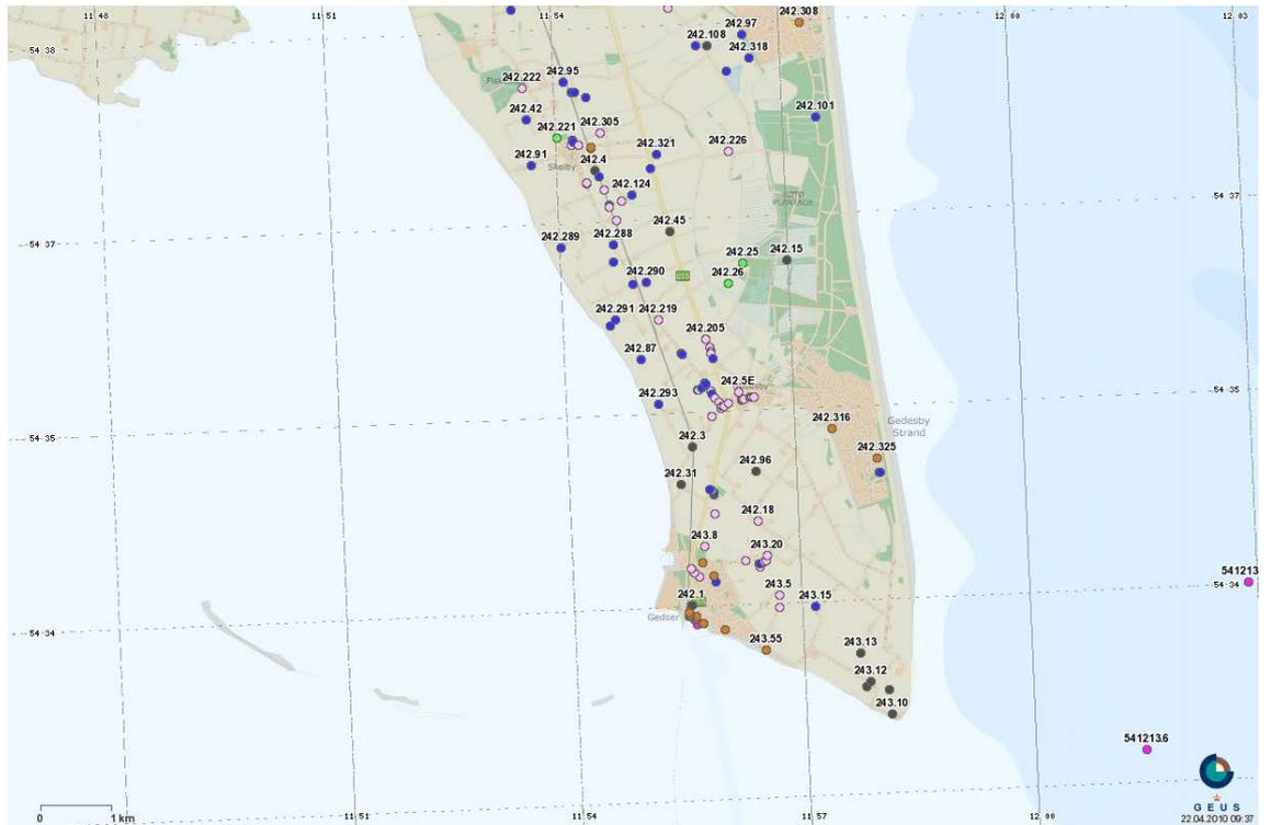
Figure 7. Map of the locations of boreholes from the Jupiter Database at GEUS. Legend: 242. 31: DGU no., Blue dot: Water supply well, Red dot: Geotechnical borehole, Pink dot: Raw material borehole, Green dot: Other borehole, Light red dot: Abandoned borehole, Black dot: Unknown purpose.
