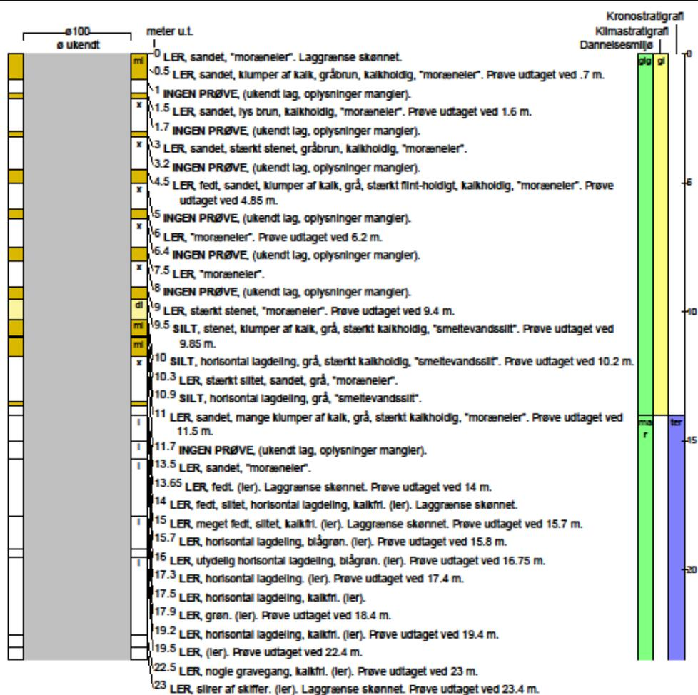
Figure 38. Geological log from borehole DGU no. 240.334 from the Jupiter Database. Upper parts of the 122 m deep borehole drilled for bentonite exploration.
