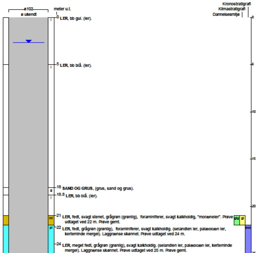
Figure 9. Geological borehole log of DGU No. 242.156. Upper part of the 44 m deep borehole. Legend: Brown: clayey till, Blue: Paleocene Clay.
