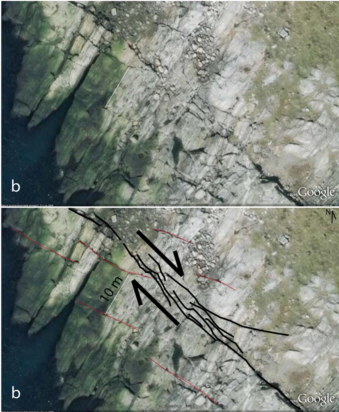
Figure 16. Enlargement-b from Figure 14. A coast parallel fracture system showing a brittle zone that could be interpreted as probably right-lateral fault zone. Such a brittle fabric could be related to recent movement along the contact.
