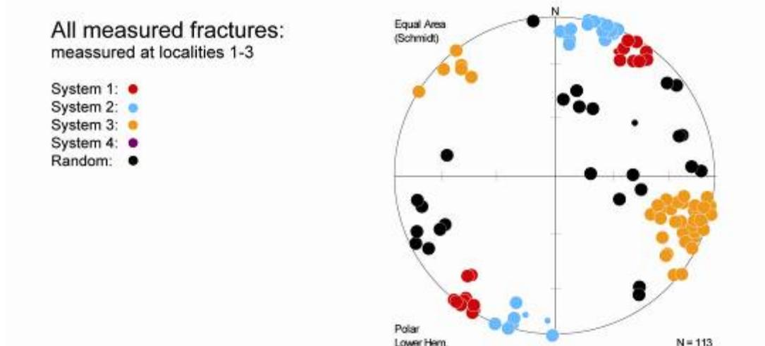
Figure 9. The map shows the SW part of Ukkusissat and adjacent area. Fractures are mapped from orthophotos along with faults and fracture systems. Fractures were measured along scanlines at three localities, and their orientation is shown on the stereonet below.
