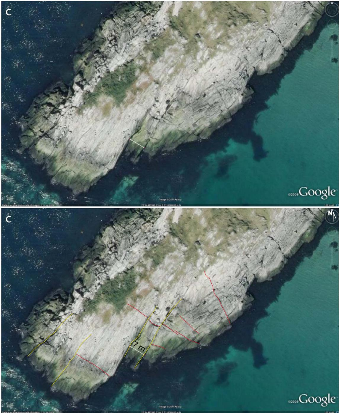
Figure 18. Enlargement-c from Figure 14. Fracture systems with orthogonal trends well developed along the coastline. The cross-cutting relationship between the two fracture system is not clear from orthophotos.
