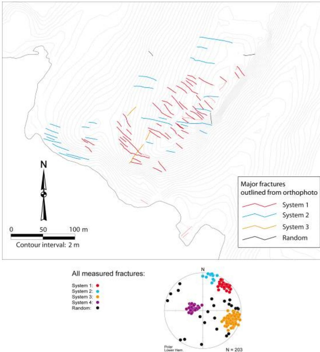
Figure 8. The Qinggorput locality. The map shows the fracture traces outlined from orthophoto. The stereonet below shows the orientation of all fractures measured along scanlines in the area. (from Jakobsen & Larsen, 2004)
