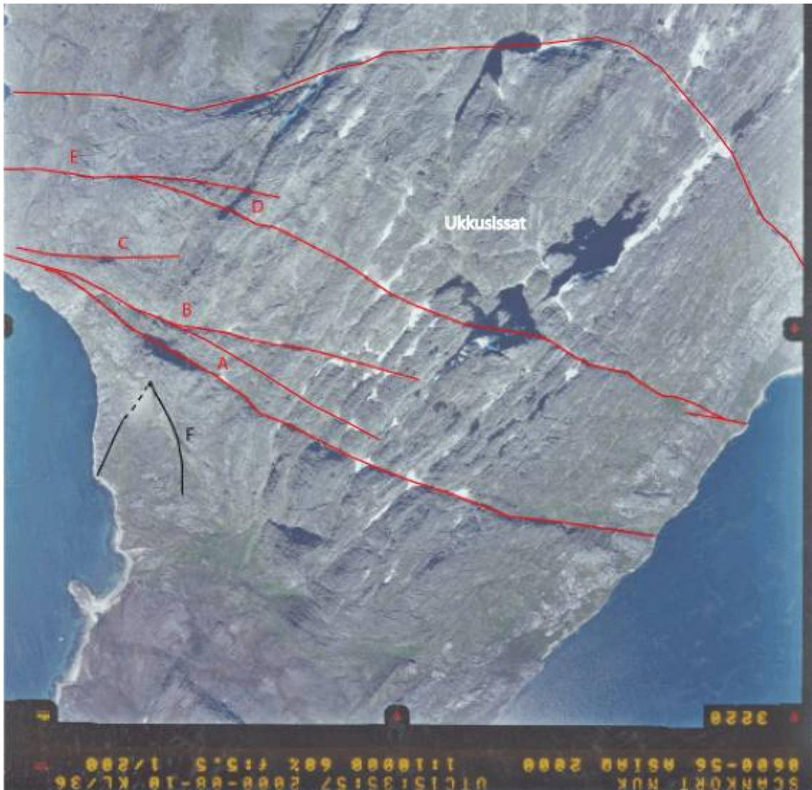
Figure 10. Aerial photo of the southern part of Ukkusissat. The red lines outline major fault/fracture systems cutting across the Ukkusissat ridge.
