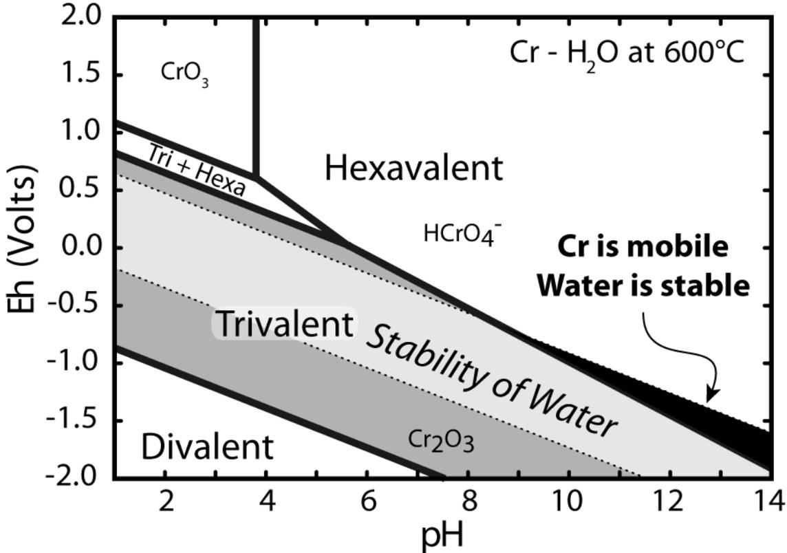
Fig. 12. Eh-pH diagram showing the valance and species of Cr along with the stability of water.
