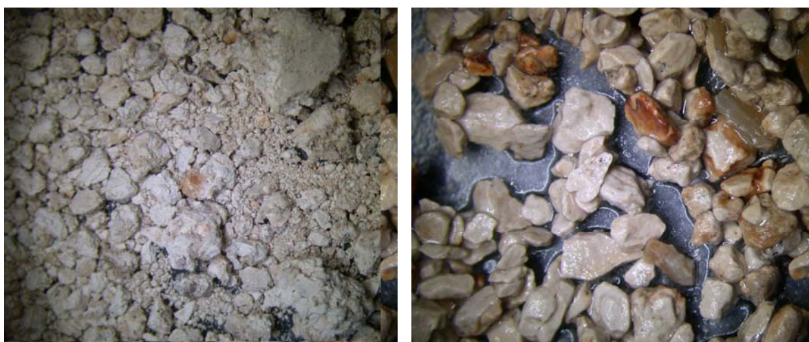
Figure 2.1. Photos of washed and cleaned cuttings fractions. Some samples had problems with mud sticking to the surface of cuttings (left), even after the initial washing and cleaning; an additional sieving and washing under tap water cleaned up the cuttings. Non-chalk constituents, mis-coloured or iron-coated cuttings were removed by hand picking or a magnet (right). Credit: Mærsk Laboratory.
