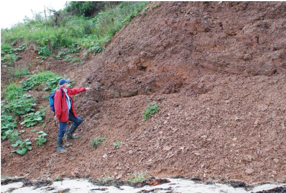
Figure 1. Red, calcareous, very fine-grained, sticky, plastic marine clay with microfossils (Røsnæs Clay Formation) at Albæk Hoved, Jylland.
