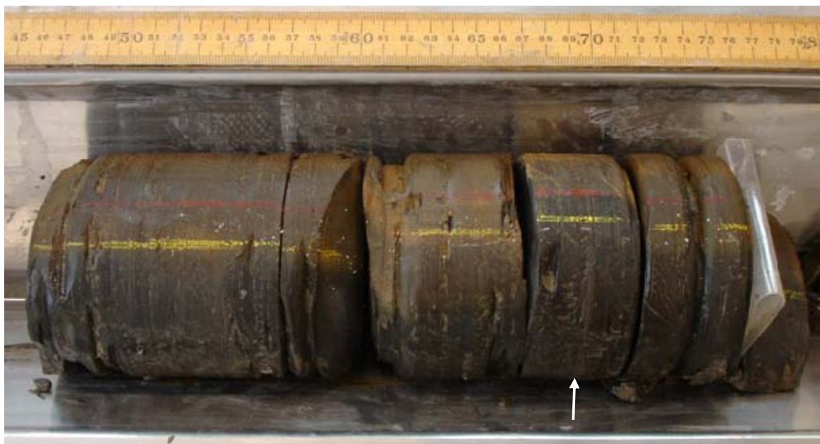
Fig. 2.2. Stenlille-2, C#2, B#5, 1483.8 – 1484.8 m. The photo shows the lower ~ 30 cm of the core box before several attempts to cut a cylindrical plug; top of box is towards the left. A vertical 1½" (38 mm) plug was cut successfully from one of the bottom pieces of full core (arrow) at 1484.7 m. The well was drilled in 1987 and the caprock section of core #2 preserved with drilling mud and simulated formation water in the glassfiber liner tube. After 23 years of preservation the core appears as fresh a the day it was received in the laboratory.
