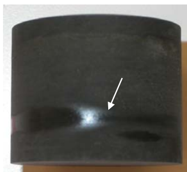
Figure 2.3. Side and top of the vertical \varnothing ~ 38 mm diameter plug sample drilled for the reservoir condition caprock test. A partly open, bedding plane parallel fracture is seen at the white arrow as formation water is slowly leaking out from the fracture. The fracture does not present a problem to the caprock test because the direction of flow is perpendicular to the fracture.
