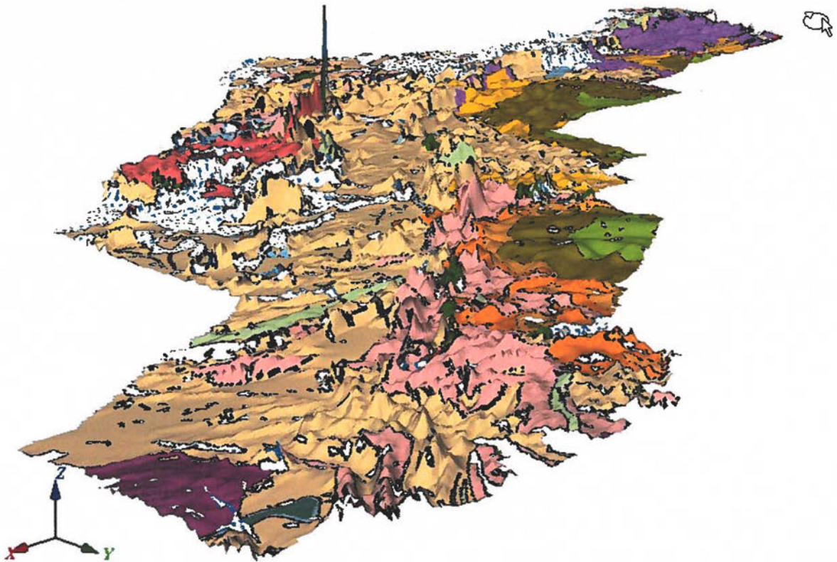
Figure 22. Geological map draped onto the relief of the total magnetic field anomaly from the AEM Greenland 1994 survey. View from northeast. With the exception for the Smith Sound Group, black lines represent boundaries between rock units.
