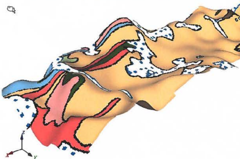
Figure 37. Geological map draped on Bouguer anomaly (1500 m half-wavelength, 2.67 \text{ g/cm}^3 ) from eastern part of the 2010 survey. View from northeast. With the exception for the Smith Sound Group, black lines represent boundaries between rock units. The legend is shown in Figure 15.
