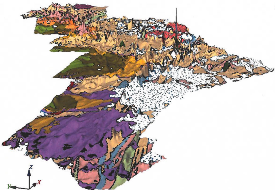
Figure 23. Geological map draped onto the relief of the total magnetic field anomaly from the AEM Greenland 1994 survey. View from west-southwest. With the exception for the Smith Sound Group, black lines represent boundaries between rock units.
