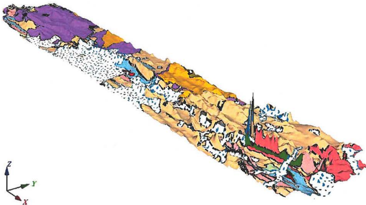
Figure 20. Geological map draped on total magnetic field anomaly data from the SGL 2010 survey. View from southeast. With the exception for the Smith Sound Group, black lines represent boundaries between rock units.
